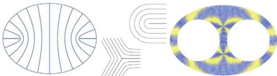
Fig. 5.13 Left : A texture in a nematic film with two positive half-charged defects. Center : The director field near positive ( top ) and negative ( bottom ) half-charged defects. Right : The nematic field with two negative half-charged defects in a film with two holes
