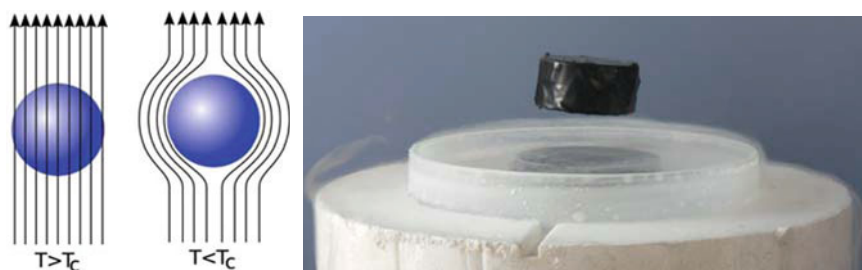
Fig. 6.9 Left: Magnetic field avoiding a superconductor. Right: A levitating magnet
