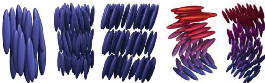
Fig. 5.11 Schemes of liquid crystalline phases. From left to right : nematic, smectic A, smectic C, cholesteric, smectic C*
