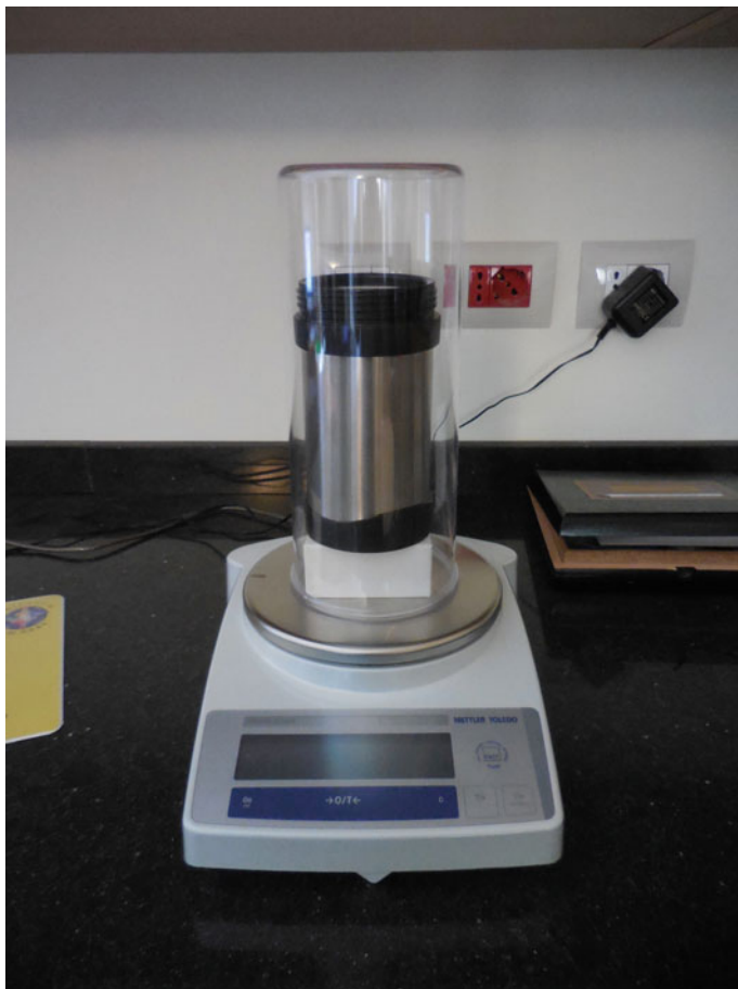
Fig. 14 The apparatus for measuring heat capacity by LN2 immersion
