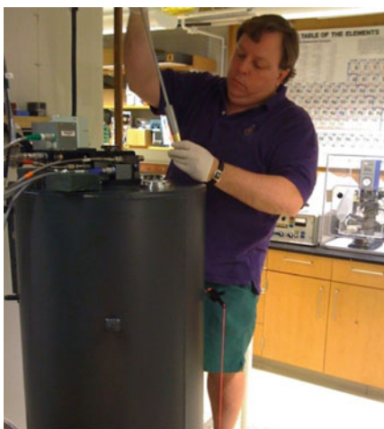
Fig. 12 (above) Fr. Cyril Opeil S.J. with the quantum design physical properties measurement system—thermal transport option (PPMS) at Boston College. (below) A small piece of a meteorite in the PPMS sample mount (Source C. Opeil S.J.)
