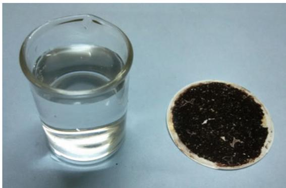
Nanosheets have nanoscale thickness, but the other two dimensions are much larger in size when compared to nanoparticles and hence nanosheets can be filtered out easily. The reaction mixture containing the catalyst was poured into a filtration assembly with a  $0.2\ \mu\text{m}$  cellulose acetate membrane. TNS catalyst was easily filtered out from the reaction mixture leaving behind a clear permeate (Fig. 6).
