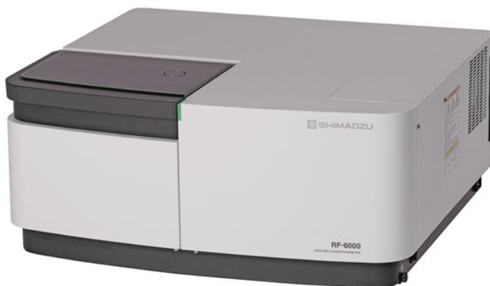
Fig. 3.5 UV-vis spectrofluorophotometer. Courtesy of Shimadzu
