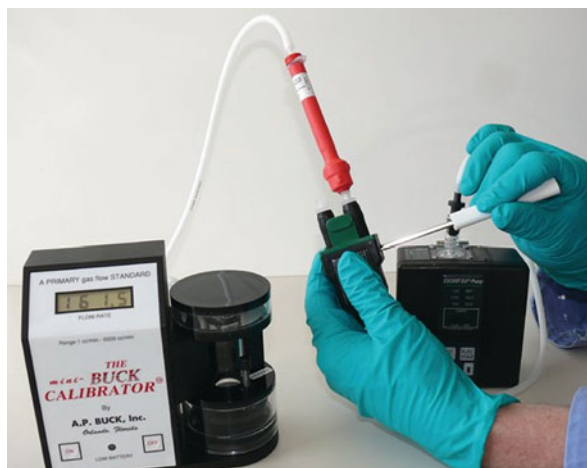
Fig. 4.3 Air sampling pump. Courtesy of Sigma-Aldrich
