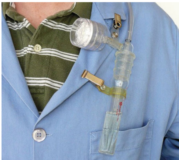
Fig. 4.4 Cassette for particulate sampling. Courtesy of Sigma-Aldrich
