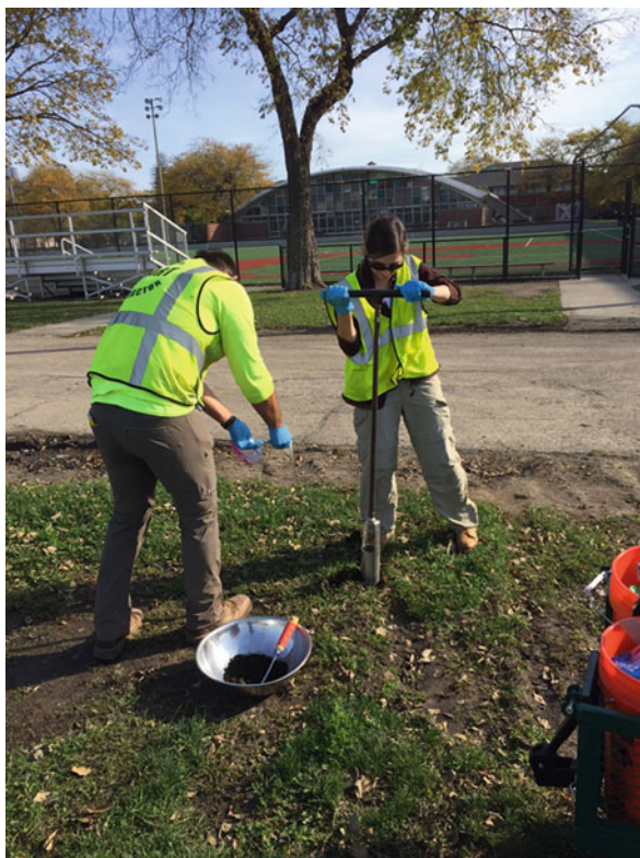
Fig. 4.7 Soil sampling with an auger device. Courtesy of U.S. EPA
