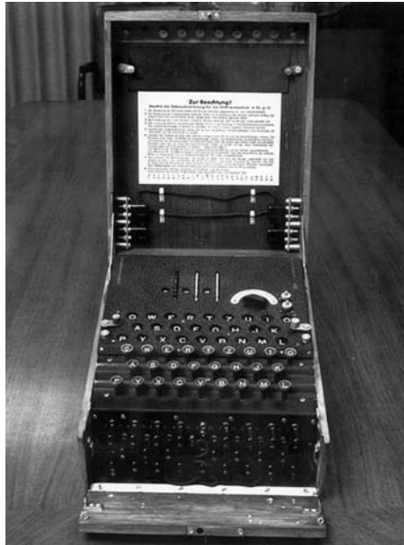
Exhibit 1-4 The German Enigma coding machine.
