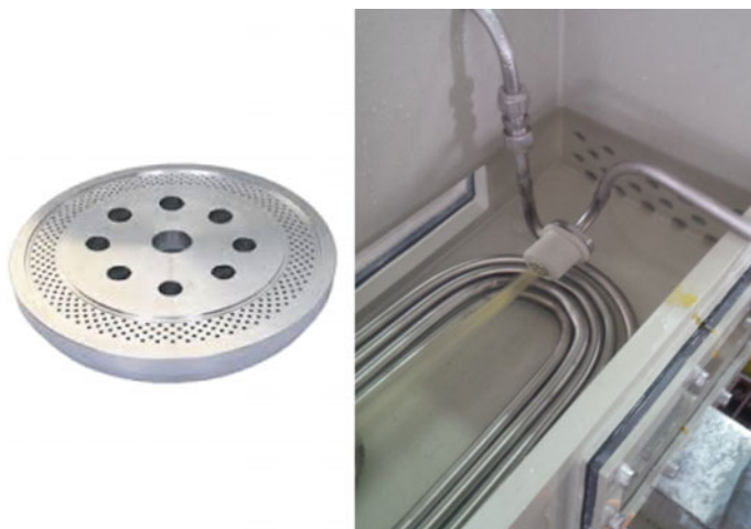
Fig. 5.66 Enlarged photo of a spinneret (left, https://www.tradeindia.com/fp1246480/Spinneret-For-Staple-Fibre-Yarn.html , accessed on September 29, 2017) and the dope filaments as they are pressured out of the orifices (right, courtesy of Thuringian Institute for Textiles and Plastics Research, TITK, Rudolstadt, Germany)
