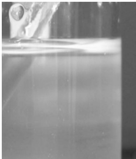
Fig. 5.53 Cellulose (2%) dissolved in an aqueous mixture of 7% NaOH with 0.6% boric acid
