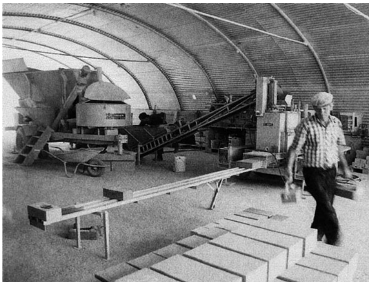
Fig. 8.8 Hydraulic machine for CEB production
