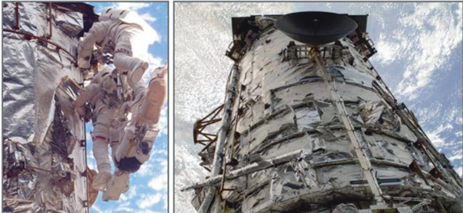
Fig. 3.5. Severe degradation to the outer layer of the Hubble Space Telescope's multi-layer insulation after 19 years of exposure. Image Credit: NASA
