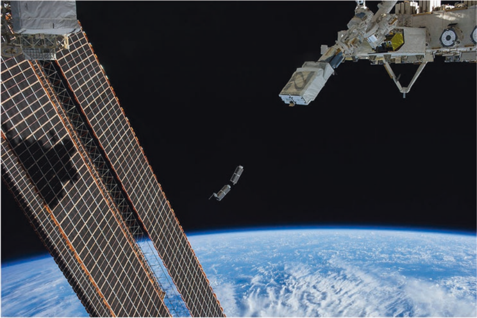
Fig. 4.6. A set of NanoRacks CubeSats is photographed by an ISS crew member after the deployment by the NanoRacks Launcher attached to the end of the Japanese robotic arm. (February 25, 2014). Image Credit: NASA
