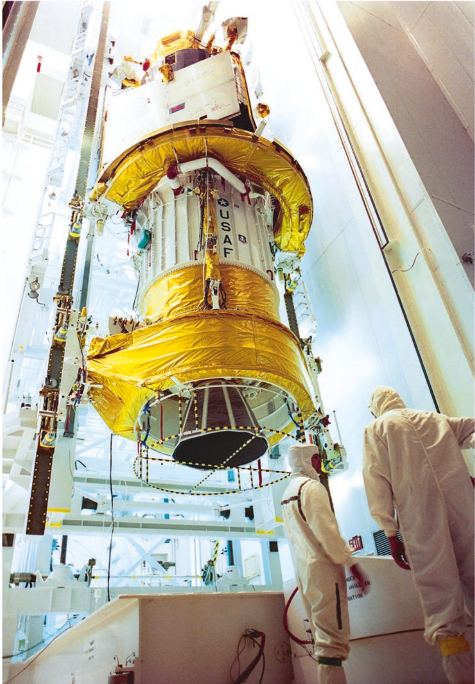
Fig. 7.3. STS-44 DSP satellite and IUS during preflight processing at Cape Canaveral. Image Credit: NASA
