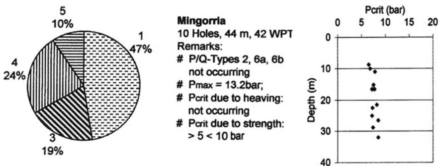
Fig. 5.21 Mingorria. Portion of P/Q-Types (left) and relation  $P_{crit}/\text{Depth}$  for Types 3 and 5 (right)
