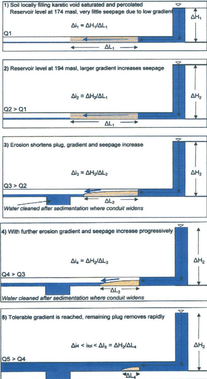
Fig. 3.57 Mujib Dam. Erosion of fillings from plugged karst channels at higher hydraulic gradient
