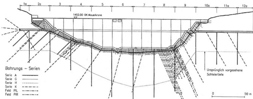
**Fig. 3.41** Panix Dam. Original area of grout and boreholes curtain eventually carried out: Series A and K—drilled for investigation, Series G and H—contact grouting along the inspection gallery, PIL and PIR—local test grouting on the left and right slopes, respectively
