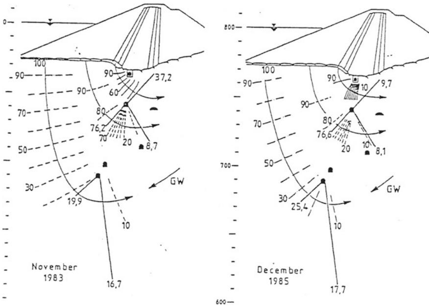
**Fig. 3.39** Pueblo Viejo Dam. Uplift reduction (given in %) during fully impounded reservoir in November 1983 and December 1985, section indicates the situation beneath the right abutment
