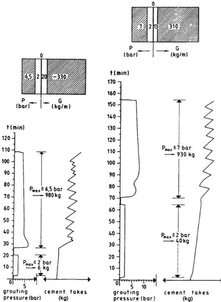
**Fig. 3.27** Aabach Dam. Tests to investigate course of grouting—very small grout takes during low pressure but large take after intentional hydrofracturing
