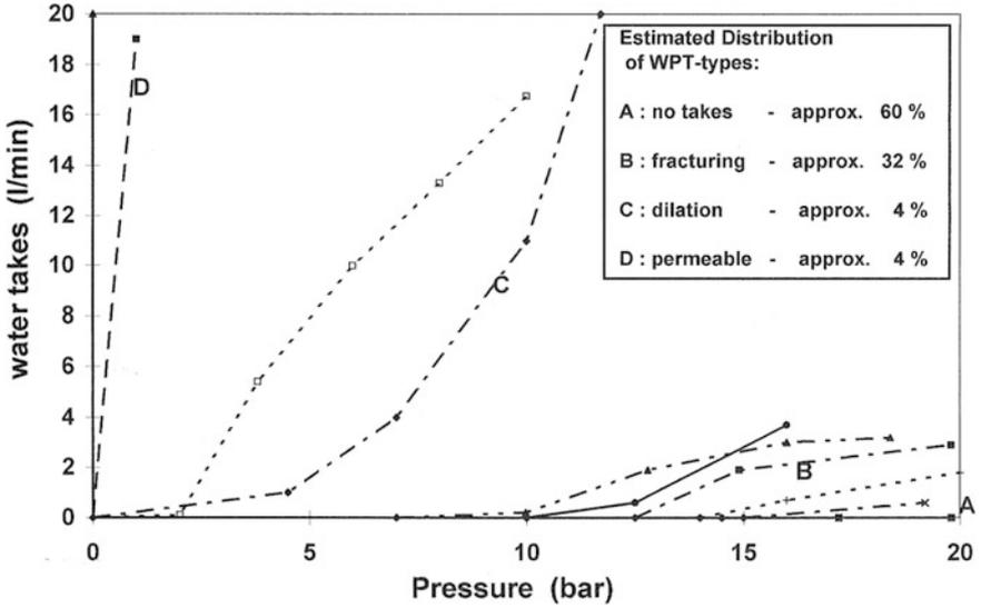
**Fig. 4.18** Typical classification of P/Q-diagrams. Competent granite fractured at medium-sized pressures due to laminated texture
