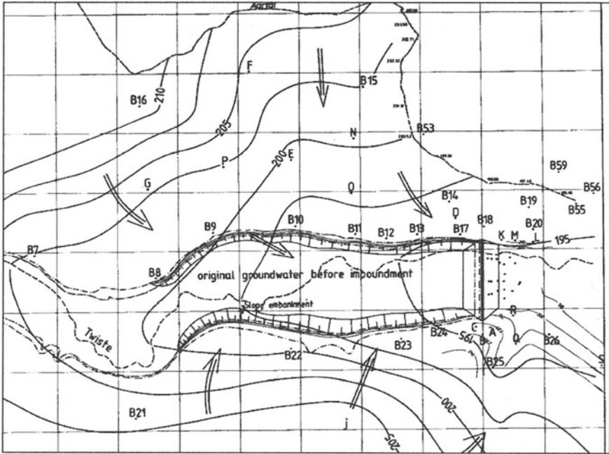
Fig. 7.9 Twiste Dam. The original groundwater table
