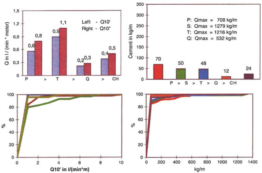
**Fig. 3.50** Mujib Dam. Mean values and frequency distribution of WPT-results (*left*) and grout takes (*right*) obtained in Section GG of Phase 1
