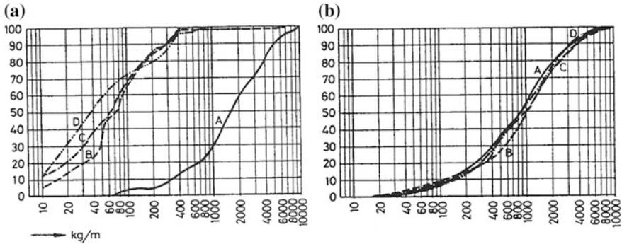
Fig. 3.11 a, b Twiste Dam, frequency distribution of grout takes for series A, B, C, D
