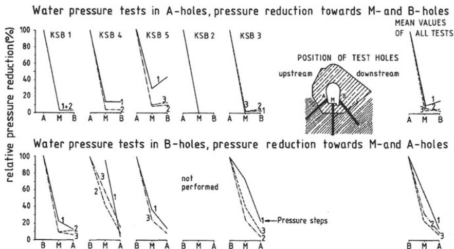
Fig. 4.22 Different directions of WPT to examine different uplift reduction
