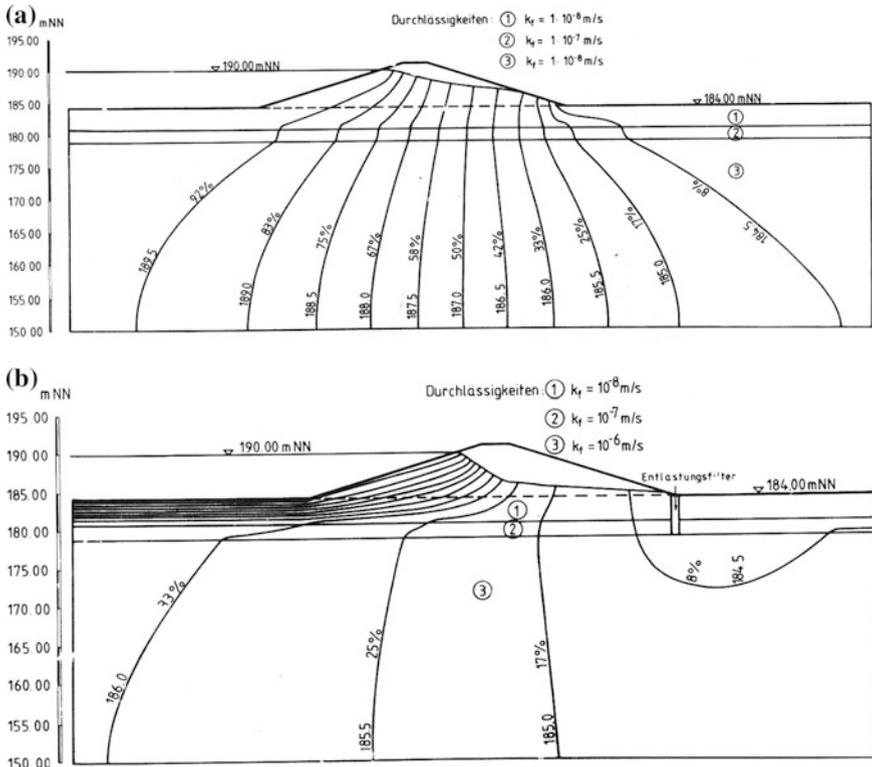
Fig. 7.11 a–f Modelling of the under-seepage at the Sandwasser Dam under different settings
