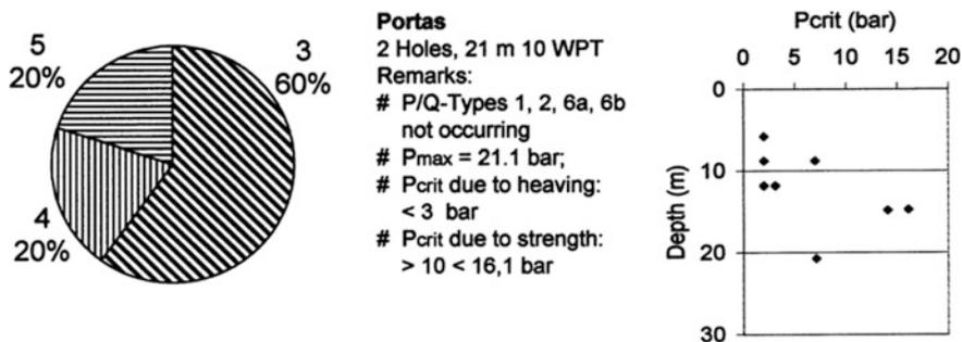
Fig. 5.24 Las Portas. Portion of P/Q-Types (left) and relation  $P_{crit}/Depth$  for Types 3 and 5 (right)
