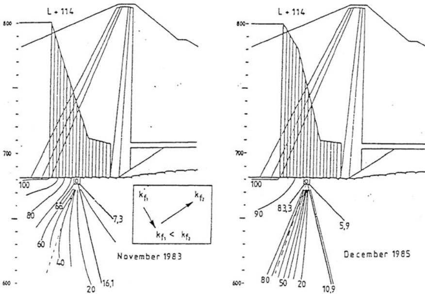
**Fig. 3.38** Pueblo Viejo Dam. Uplift reduction during fully impounded reservoir in November 1983 and December 1985, section indicates the situation within the middle of the valley
