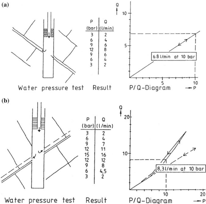
Fig. 4.2 a WPT, increasing and decreasing pressure steps, P/Q-diagram indicating a linear relationship. b WPT, increasing and decreasing pressure steps, P/Q-diagram indicating an over-proportionate relationship caused by dilation
