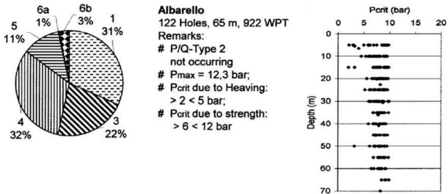
Fig. 5.8 Albarello. Portion of P/Q-Types (left) and relation  $P_{crit}/Depth$  for Types 3 and 5 (right)
