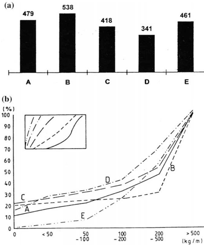
**Fig. 3.31** Yuracmayo Dam. **a** Mean values of grout takes in subsequent series, **b** summation curves of frequency distribution of individual grout takes of subsequent series; small one inscribed exemplifies progressive sealing
