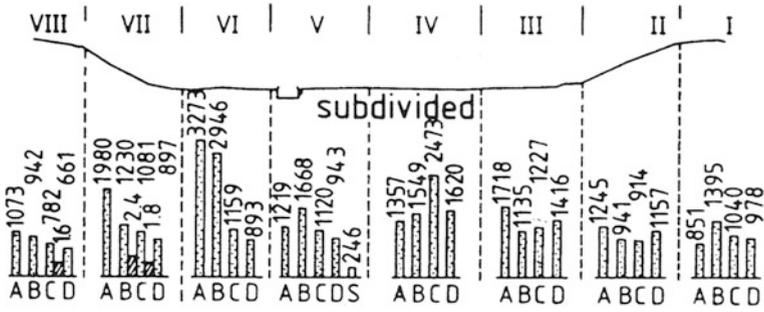
Fig. 3.8 Twiste Dam: mean values of grout takes
