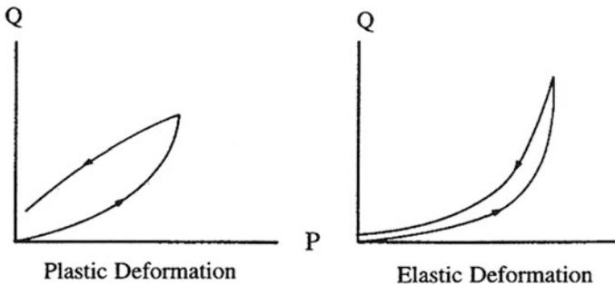
**Fig. 4.14** P/Q-diagrams indicating dilation of water paths
