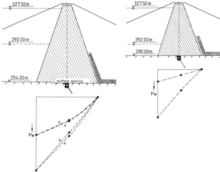
**Fig. 3.6** Tavera Dam. Linear reduction of uplift pressure
