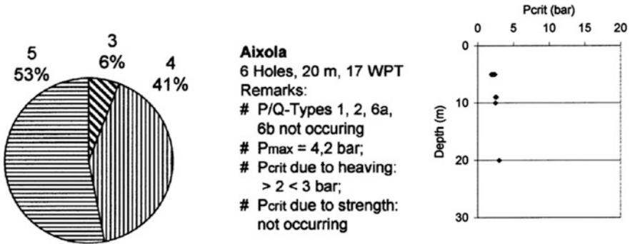
Fig. 5.7 Aixola. Portion of P/Q-Types (left) and relation  $P_{crit}/Depth$  for Types 3 and 5 (right)
