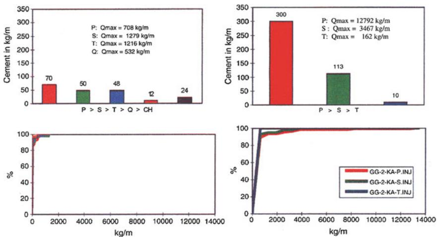
**Fig. 3.52** Mujib Dam. Mean values and frequency distribution of grout takes obtained in Section GG of Phase 1 (*left*) and Phase 2 (*right*)
