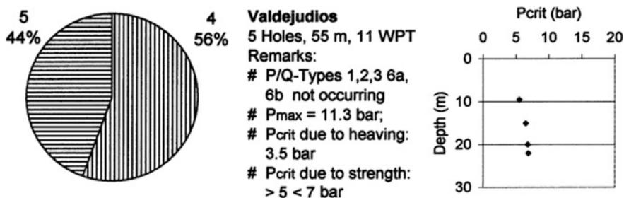
Fig. 5.27 Valdejudios. Portion of P/Q-Types (*left*) and relation  $P_{crit}/\text{Depth}$  for Type 5 (*right*)
