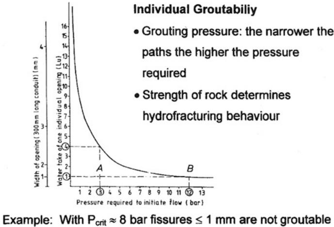
**Fig. 5.32** Relationship between width and grouting pressure determined on geologically defined models
