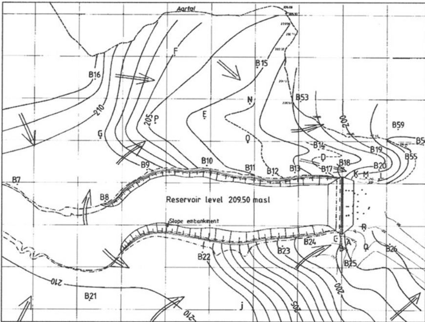
Fig. 7.10 Twiste Dam. Groundwater table after filling the reservoir
