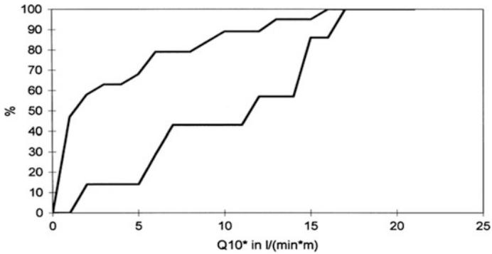
**Fig. 5.31** Relative frequency distribution for the WPT-results obtained in Hole B 5, differences between  $Q_{10}'$  (left) and  $Q_{10}^*$  (right)
