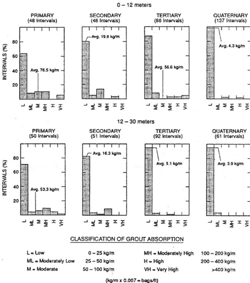
Fig. 6.6 Frequency distribution of grout takes based upon grout take classification proposed by Deere
