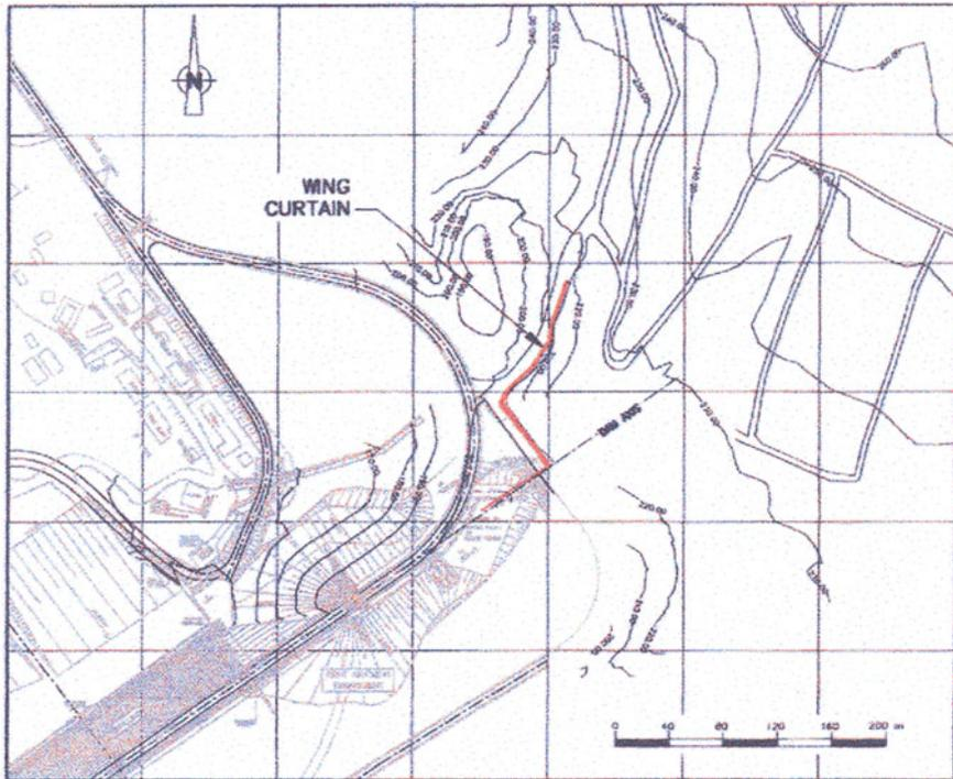
**Fig. 3.47** Mujib Dam. Layout of the grout curtain at the right abutment; in red: Wing Curtain
