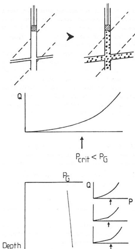
There, only wide fissures can be grouted requiring low pressures due to their small head losses activated by friction. With depth, the grouting pressures can increase, thus, narrower paths can be sealed, leaving a smaller residual permeability. Grout suspensions of low viscosity should be preferred. Heavier suspensions imply the risk of a more intense fracturing.
