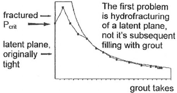
**Fig. 8.2** Grouting path curve (GPC) of Project C indicating hydrofracturing and subsequent filling
