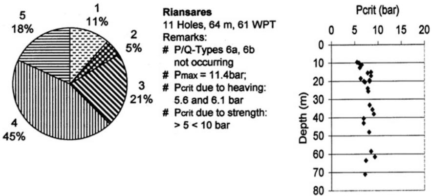
Fig. 5.26 Riansares. Portion of P/Q-Types (left) and relation  $P_{crit}/Depth$  for Types 3 and 5 (right)
