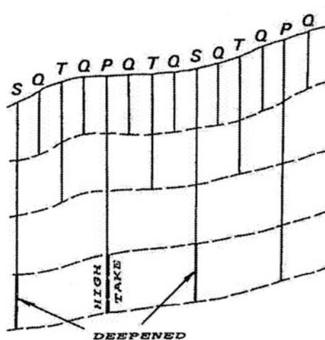
Fig. 5.29 Staggered depth for grout holes of subsequent series
