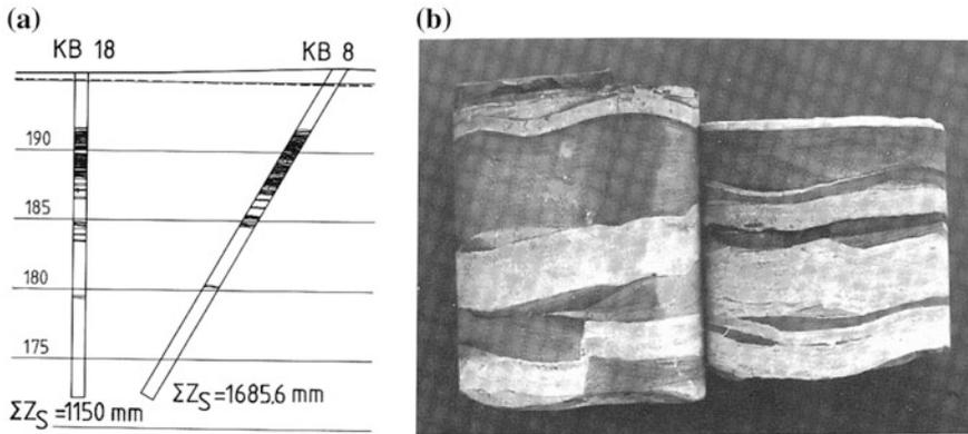
**Fig. 3.10 a, b** Twisté Dam: groutstone layers deposited along fractured bedding planes demonstrate inadequate grouting technology
