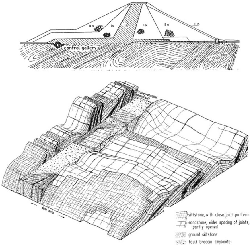
**Fig. 3.28** Aabach Dam. Geological situation in the dam area
