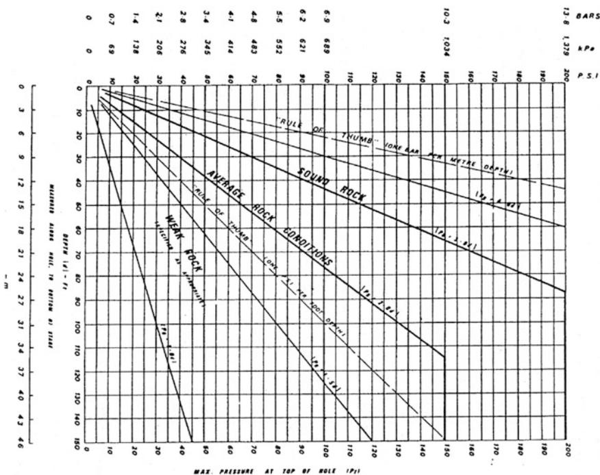
Fig. 5.28 Increase of grouting pressure with depth, different increase rates for soft and hard rock types according to Houlsby (x—pressure, above given in psi (kpa and bar, below given in psi for the top of the hole), y—depth, given in feet, and m)
