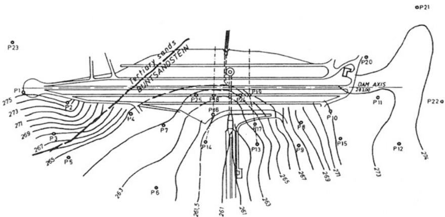
**Fig. 7.5** Antrift Dam. Influence of a fault on the reduction of uplift
