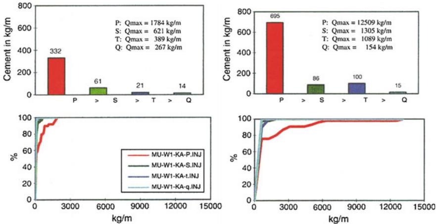
**Fig. 3.55** Mujib Dam. Mean values and frequency distribution of grout takes in Section W1 (*left*) and W2 (*right*), Phase 2
