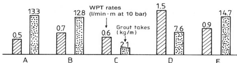
**Fig. 3.1** Tavera Dam. Mean values of grout takes for Sections III–VII, Series D and E were only made in Sections III and V
