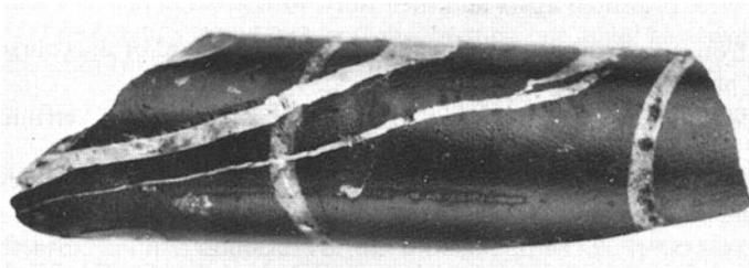
**Fig. 3.16** Möhne Dam. Groutstone deposited in fractured beddings, vertical natural Quartz-filling of fissures also fractured
