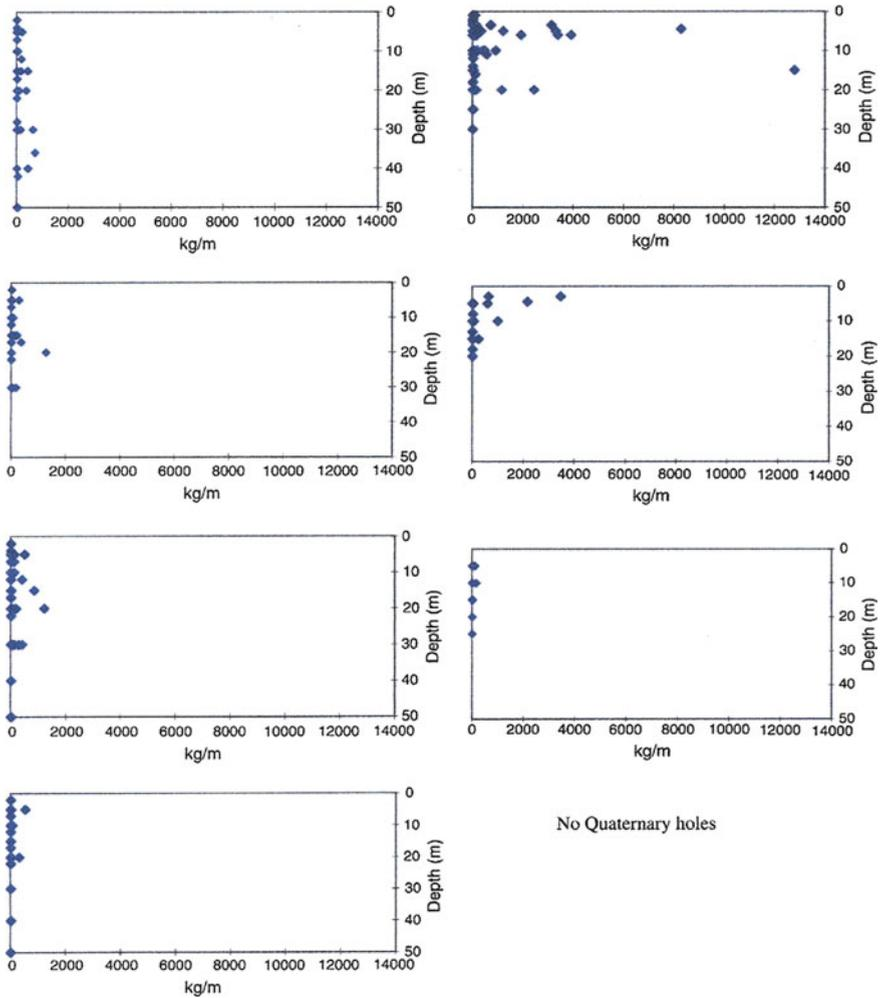
Fig. 3.53 Mujib Dam. Depth of grout takes in Series P, S, T and Q (from top to bottom) in Section GG of Phase 1 (left) and Phase 2 (right)
