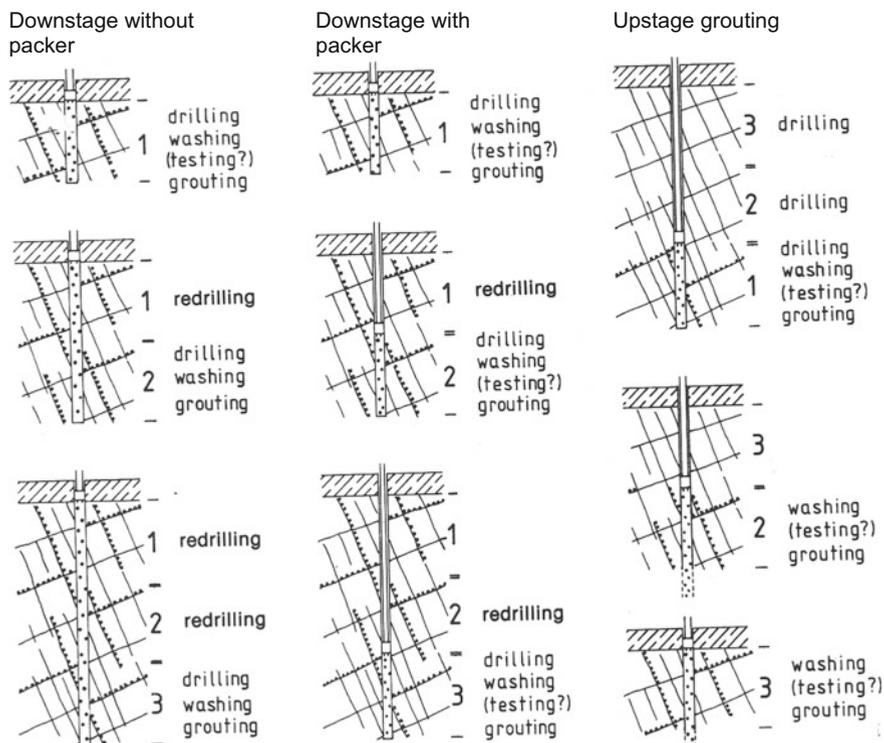
Fig. 6.3 Illustration of downstage and upstage grouting methods
