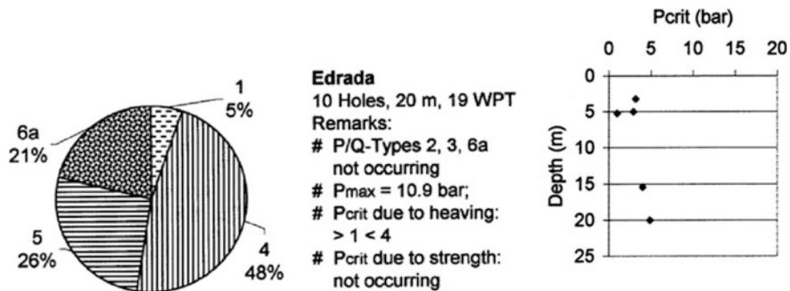
Fig. 5.18 Edrada. Portion of P/Q-Types (left) and relation P<sub>crit</sub>/Depth for Types 4 and 5 (right)
