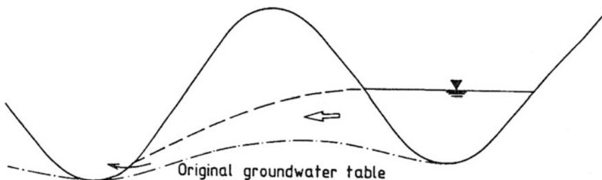
**Fig. 7.8** The deep position of the groundwater table causes a flow out of the reservoir towards the neighboring valley
