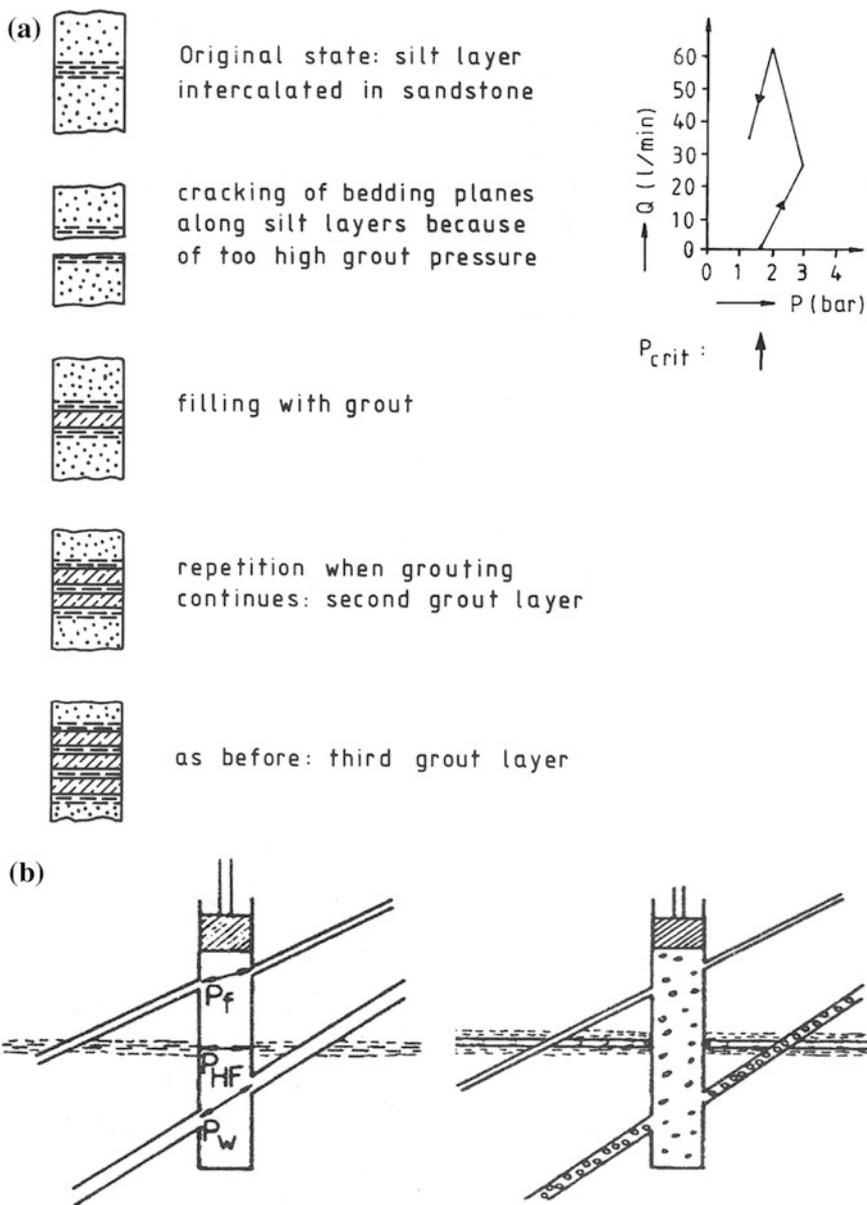
**Fig. 3.7** a Twist-dam horizontal bedding planes are fractured at low pressures and filled with grout. Further grouting phases yield repetition of fracturing along bedding planes subsequently also grouted. b Twist Dam: wide fissures are grouted at low pressures, fine fissures need high pressure but bedding planes are fractured and grouted before
