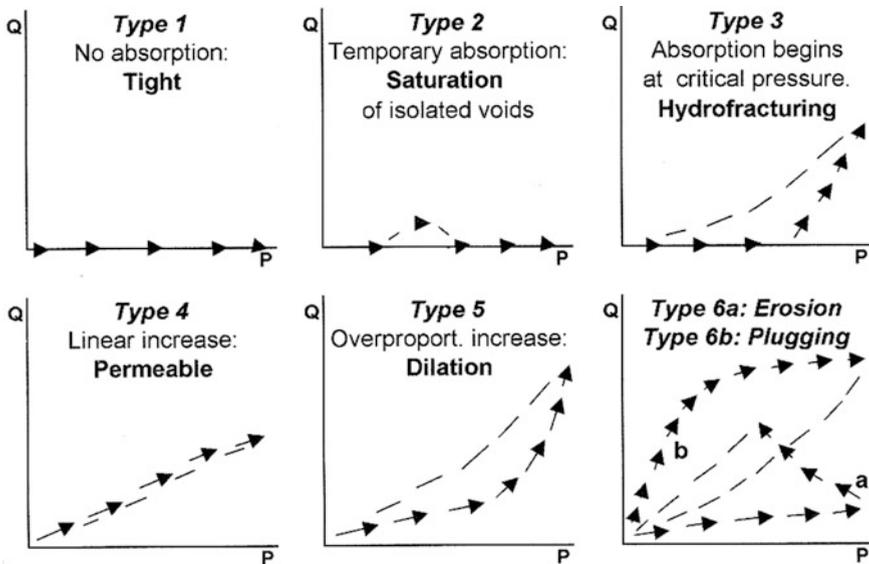
Fig. 5.4 Classification system of P/Q-diagrams identify geotechnical conditions
