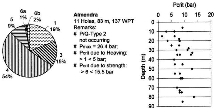
Fig. 5.9 Almendra. Portion of P/Q-Types (left) and relation P<sub>crit</sub>/Depth for Types 3 and 5 (right)
