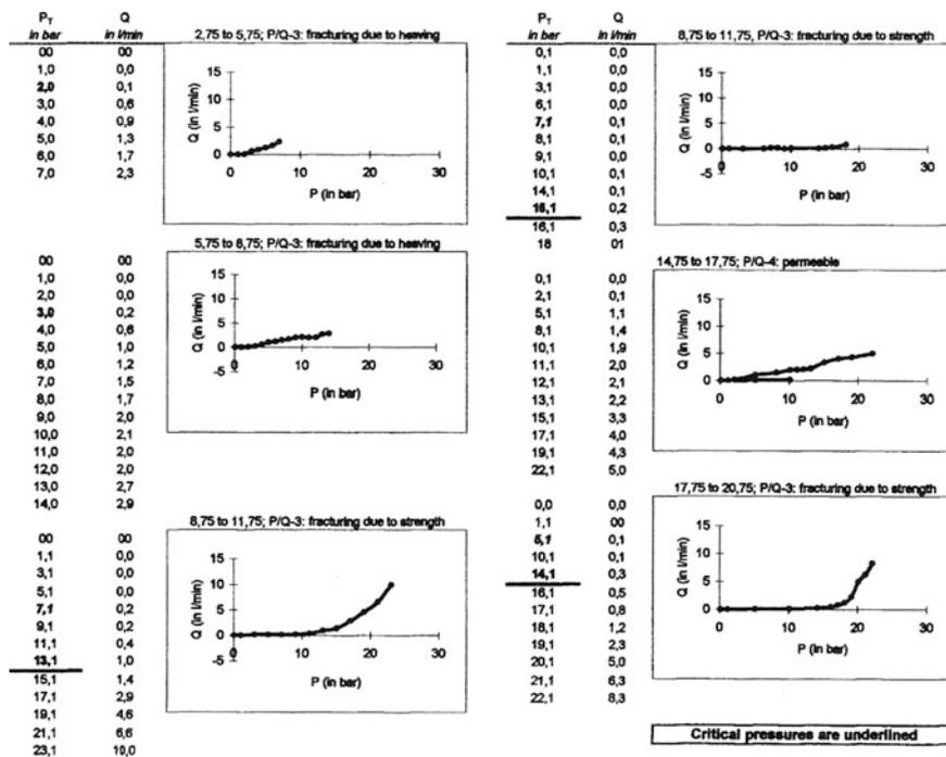
Fig. 5.3 Sequence of P/Q-diagrams originating from WPTs in Hole S-1 drilled at Las Portas
