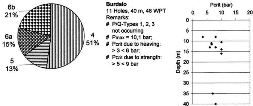
Fig. 5.13 Burdalo. Portion of P/Q-Types (left) and relation P<sub>crit</sub>/Depth for Types 3 and 5 (right)
