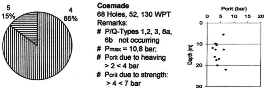
**Fig. 5.16** San Cosmade. Portion of P/Q-Types (*left*) and relation  $P_{crit}/Depth$  for Types 4 and 5 (*right*)
