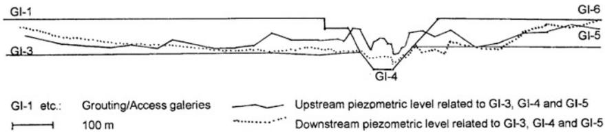
**Fig. 3.34** Pueblo Viejo Dam. Section along grouting galleries/tunnel showing piezometric levels related to fully impounded reservoir on upstream and downstream side of the curtain and changes between November 1983 and December 1985
