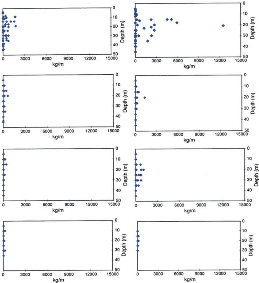
**Fig. 3.56** Mujib Dam. Depth of grout takes in Series P, S, T and Q (from *top* to *bottom*), Section W1 (*left*) and W2 (*right*), Phase 2
