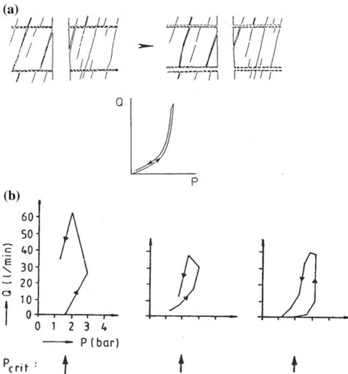
**Fig. 4.16** a Typological classification of P/Q-diagrams: sandstone-siltstone with pronounced bedding planes prone to hydrofracturing, permeable rock section is fractured along the bedding after reaching the critical pressure. b Typological classification of P/Q-diagrams: sandstone-siltstone with pronounced bedding planes prone to hydrofracturing, tight rock section is fractured along the bedding after reaching critical pressure
