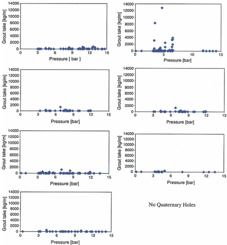
**Fig. 3.59** Mujib Dam. Relationship between grouting pressure and grout takes in Series P, S, T and Q (from *top to bottom*) in Section GG. Phases 1 (*left*) and (*right*)
