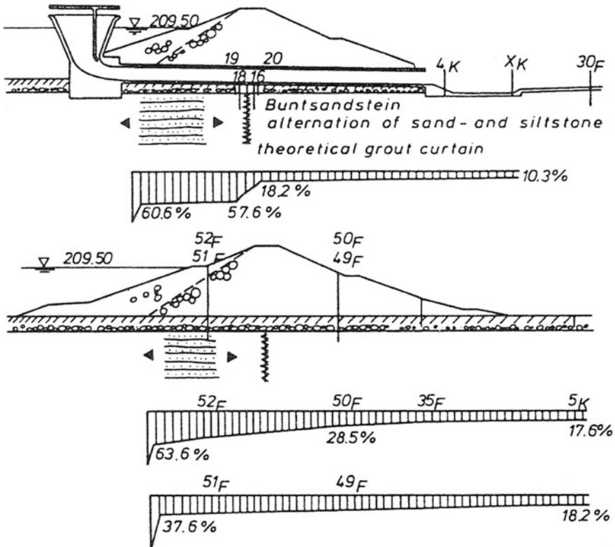
**Fig. 7.3** Twiste Dam. Over-proportionate head reduction across the alluvial loam upstream of the dam
