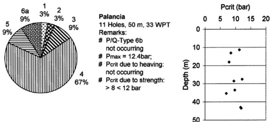
Fig. 5.22 Palancia. Portion of P/Q-Types (left) and relation  $P_{crit}/\text{Depth}$  for Types 3 and 5 (right)
