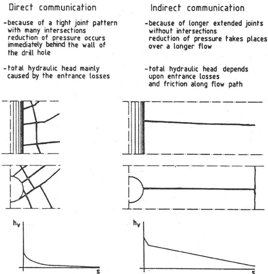
**Fig. 6.2** The relationship between the type of water routing around the borehole and grouting pressure (schematic illustration)
