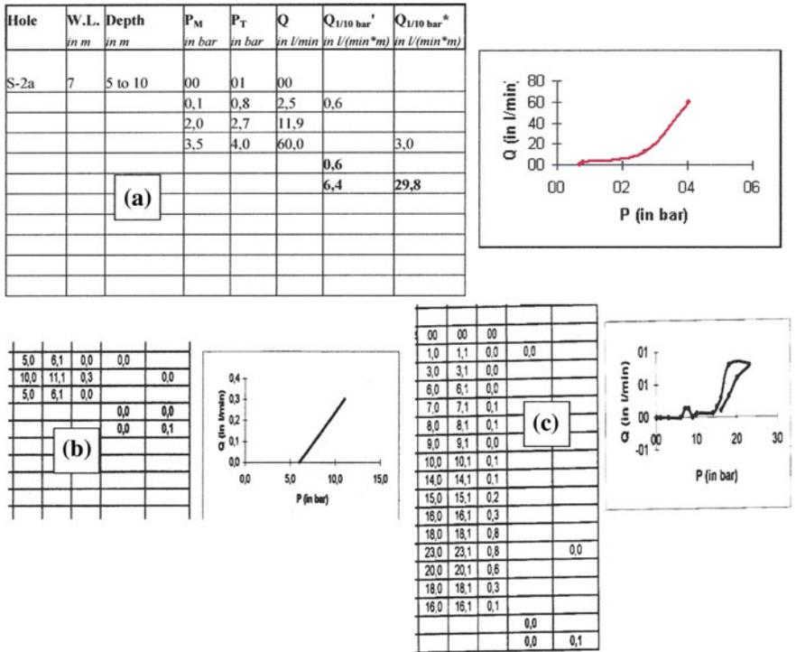
Fig. 5.2 Number of pressure steps determine accuracy of tests and their P/Q-diagrams
