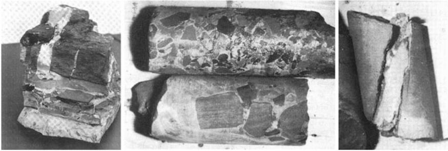
**Fig. 3.13** Twist Dam: results of grouting work Phase 1: grouted fault zone filled with debris, steep wide fissures filled with grout but interrupted by intruded horizontal groutstone layer
