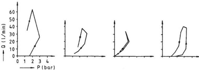
Fig. 3.12 Twiste Dam. Typical P/Q-diagrams indicating low critical pressure
