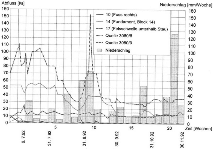
Fig. 3.46 Panix Dam. Quantities of water out of springs depend on rain falls
