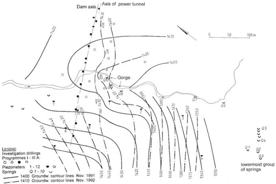
**Fig. 3.43** Panix Dam. Groundwater contour lines—before and after impoundment (1991/1992), location of drill-holes for investigation—Programs 1-III.A, piezometers 1-12, springs (Q1-Q10)
