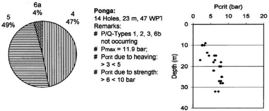
Fig. 5.23 Ponga. Portion of P/Q-Types (left) and relation  $P_{crit}/Depth$  for Types 4 and 5 (right)
