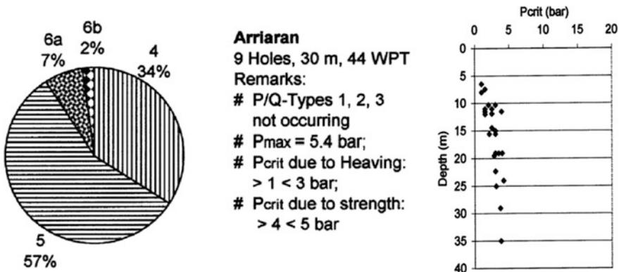
Fig. 5.11 Arriaran. Portion of P/Q-Types (left) and relation  $P_{crit}$ /Depth for Types 4 and 5 (right)
