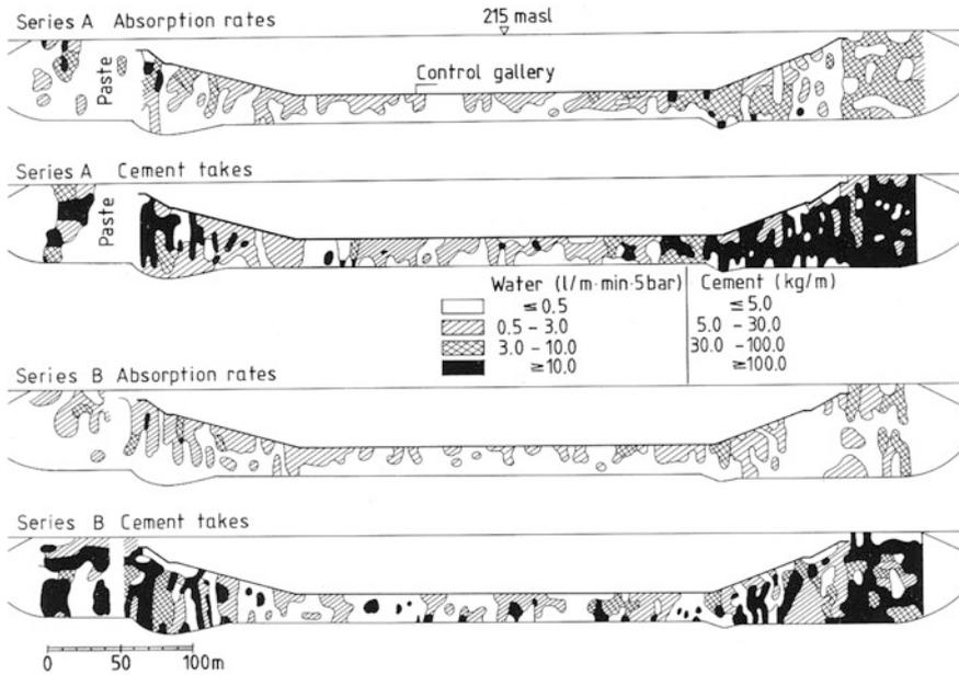
Fig. 3.18 Möhne Dam. WPT-results and grout takes of series
