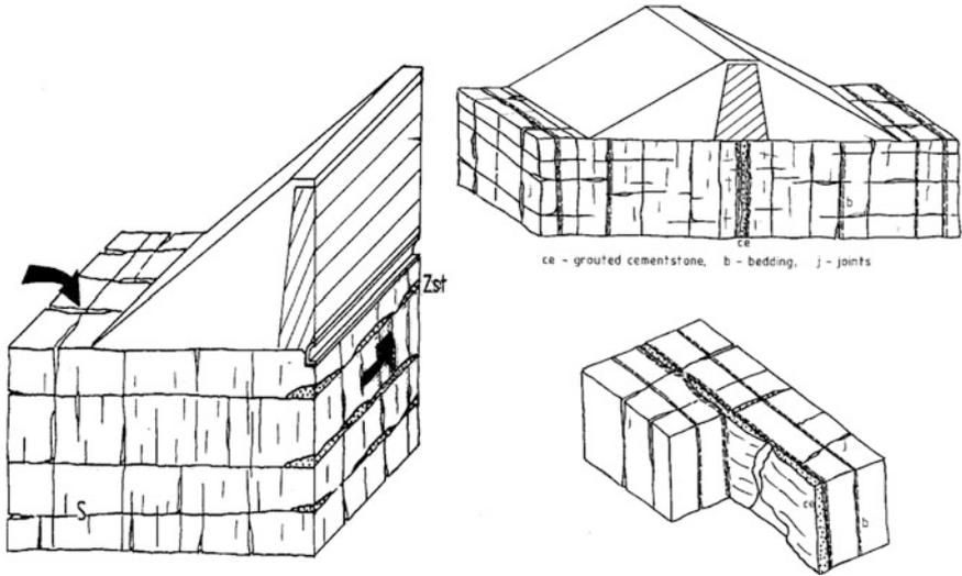
Fig. 3.25 Groutstone pillows intercalated along horizontal bedding planes have little hydraulic effect only (left), vertical pillows are possible only in exceptional cases (right)
