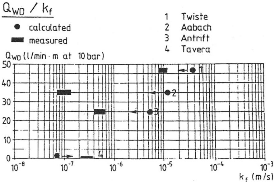
Fig. 4.13 Comparison of calculated and measured  $k_f$ -values confirm the impossibility to convert WPT-values into  $k_f$
