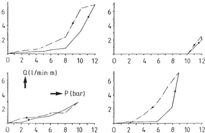
**Fig. 3.17** Möhne Dam. Typical P/Q-diagrams indicating widely ranging critical pressures; fracturing falsifies WPT-values
