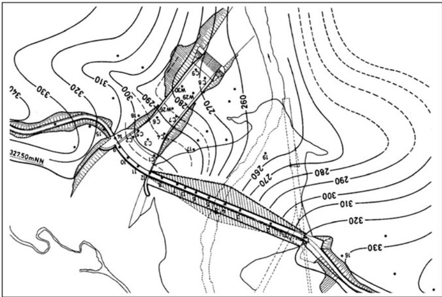
Fig. 7.2 Tavera dam. Groundwater contours show a steeply inclined groundwater table hereby confirming the imperviousness of the rock
