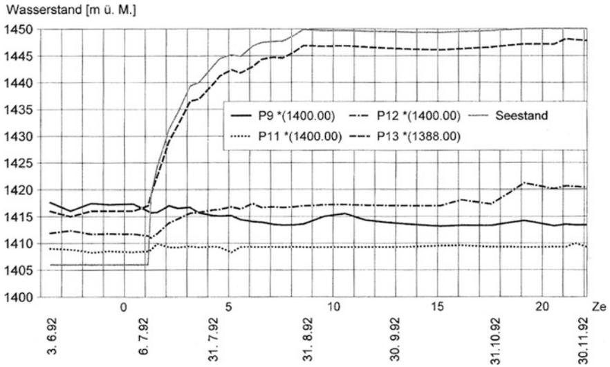
Fig. 3.44 Panix Dam. Hydrographs of representative piezometers: P9, P11, P12 downstream of the dam, P13 upstream of the dam
