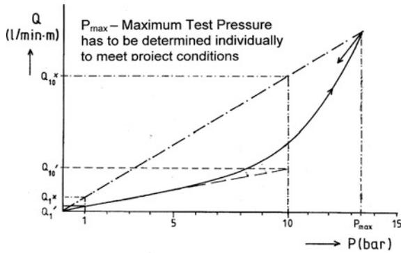
**Fig. 3.49** Definition of WPT parameters  $Q_{10}'$  (original permeability) and  $Q_{10}^*$  (provoked permeability)
