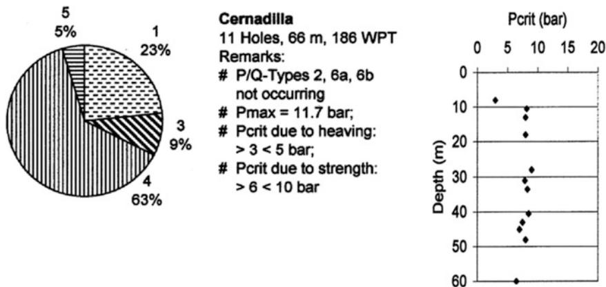
Fig. 5.15 Cernadilla. Portion of P/Q-Types (left) and relation  $P_{crit}/Depth$  for Types 3 and 5 (right)
