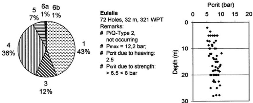
**Fig. 5.19** Santa Eulalia. Portion of P/Q-Types (left) and relation  $P_{crit}$ /Depth for Types 3 and 5 (right)
