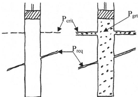
**Fig. 5.33** Open paths remain ungrouted if latent planes are fractured before
