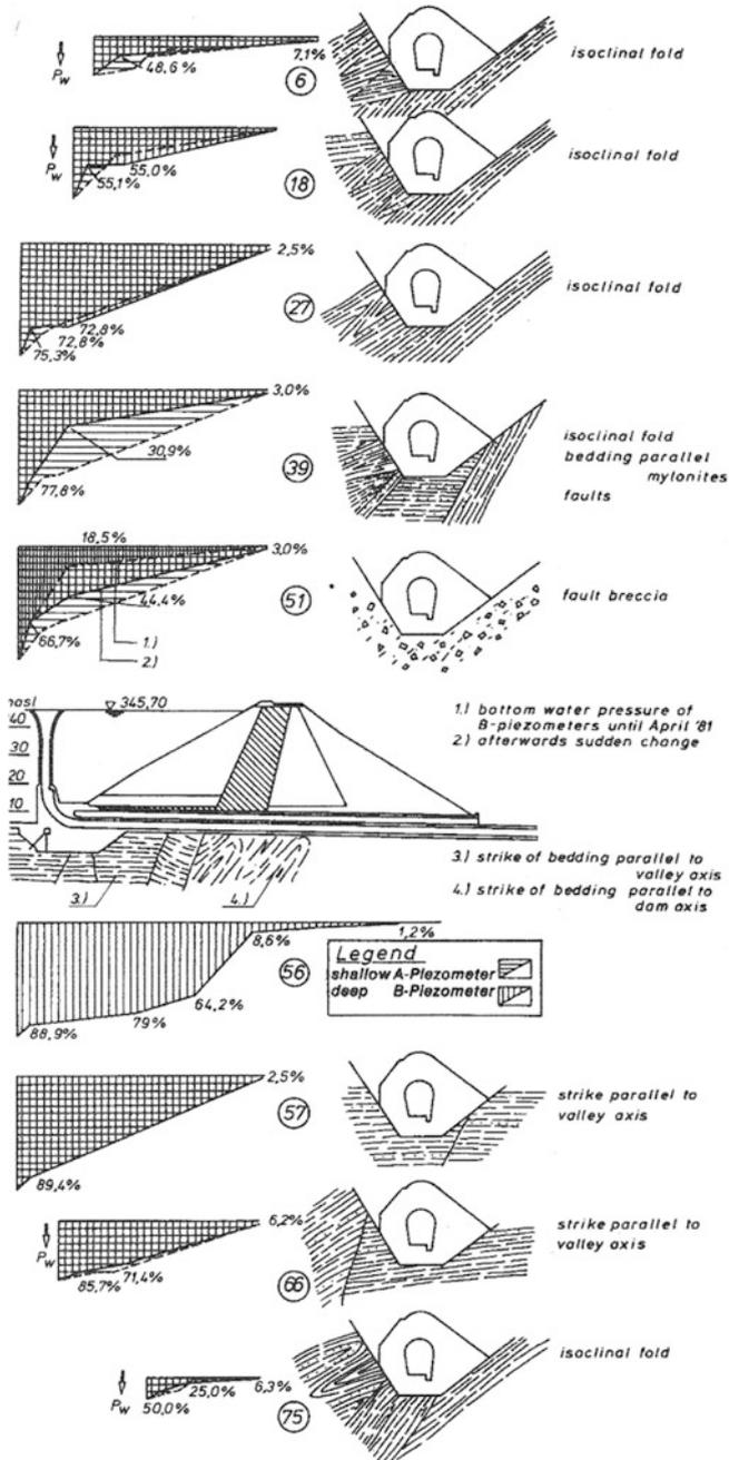
Fig. 3.29 Aabach Dam. Reduction of uplift pressure across the inspection gallery
