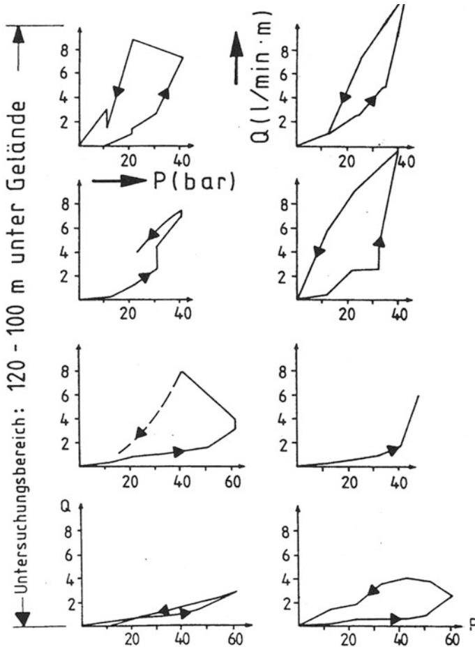
**Fig. 4.21** Typological classification of P/Q-diagrams: massive limestone, hard, fracturing occurs at very high pressures
