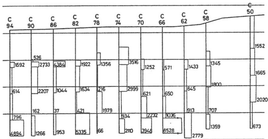
Fig. 6.4 Individual grout takes plotted in bars along groutholes
