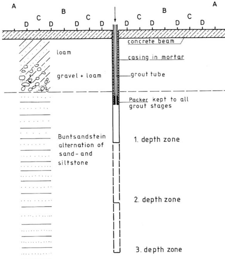
Fig. 3.9 Twiste Dam, grouting scheme, with packer fixed inside casing
