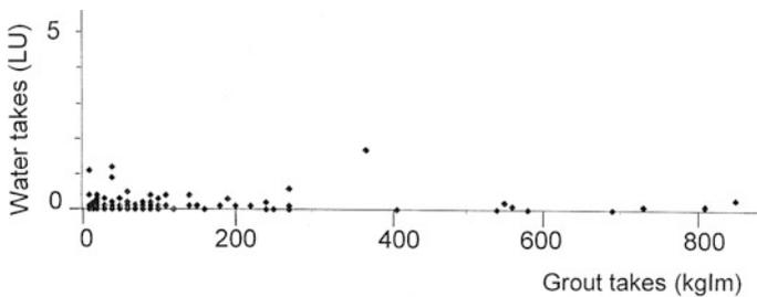
**Fig. 8.3** Even low grouting pressure provoked large grout takes due to hydrofracturing in impervious rock (Part of Fig. 3.23)
