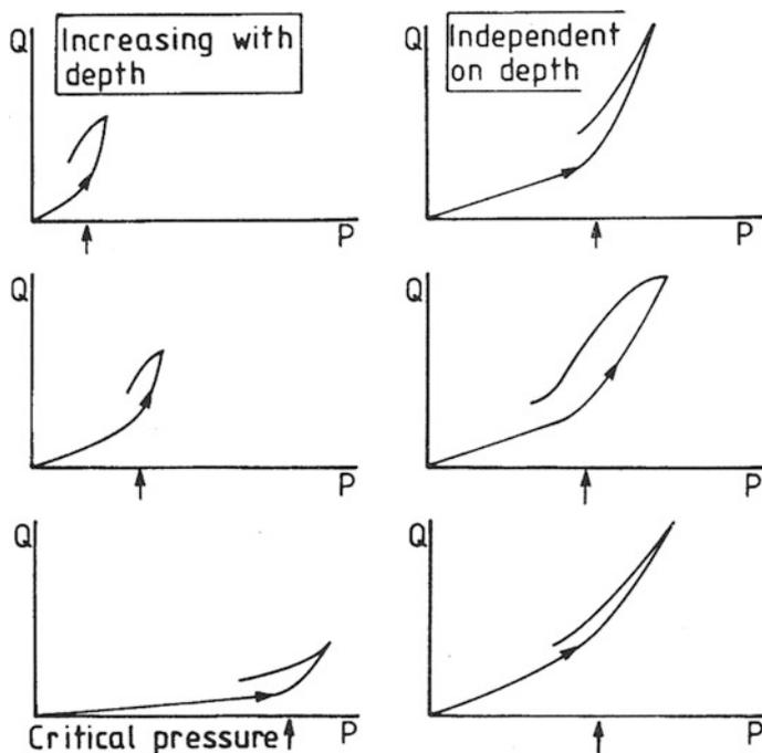
**Fig. 4.8** Critical pressures for different rock bond: disconnected—increasing with depth, connected—-independent of depth
