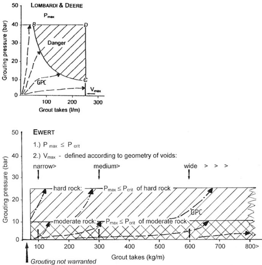
**Fig. 8.4** Comparison of grouting criteria for penetration grouting. *Top* Example for high grouting intensity of GIN = 2000, according to Lombardi & Deere. *Below* Grouting determined by individual facts: critical pressures, wide fissures absorb larger maximum grout volumes
