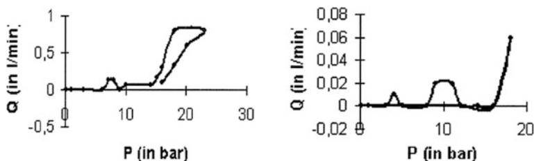
Fig. 5.25 Las Portas. Diagrams of P/Q-Type 3. Indicating gradual beginning of hydrofracturing
