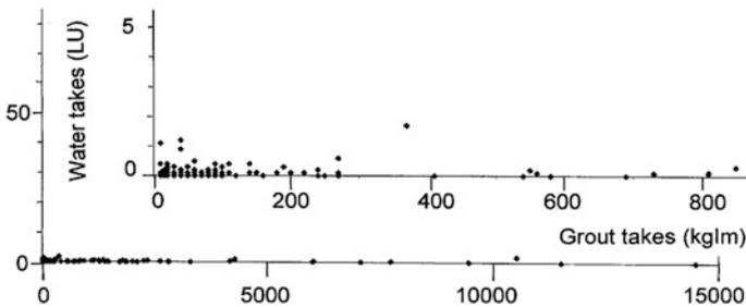
**Fig. 3.23** Almendra Dam. Relation between water and grout takes. Explanation: the upper coordinates present the segment out of the lower one at an enlarged scale:  $x = 800$  or  $y = 5$
