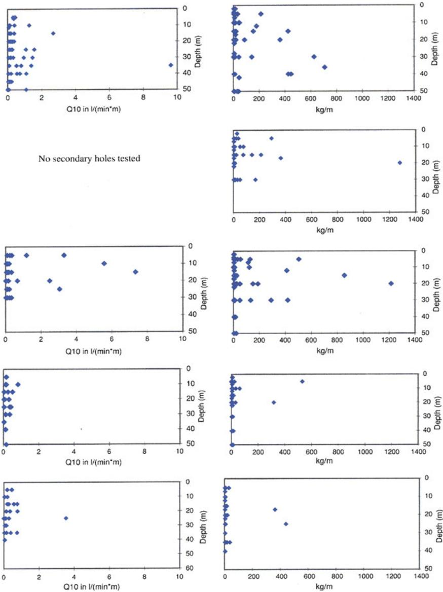
**Fig. 3.51** Depth of WPT-results (*left*) and grout takes (*right*), obtained in Series P, S, T, Q and CH (from *top* to *bottom*) in Series GG of Phase I
