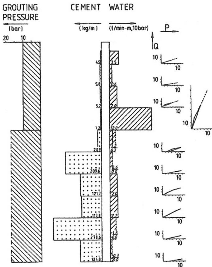
Fig. 3.3 Tavera Dam. Higher grouting pressures cause larger grout takes due to hydrofracturing
