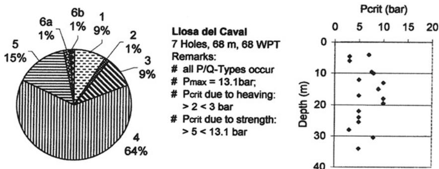
**Fig. 5.20** Llosa del Caval. Portion of P/Q-Types (left) and relation P<sub>crit</sub>/Depth for Types 3 and 5 (right)
