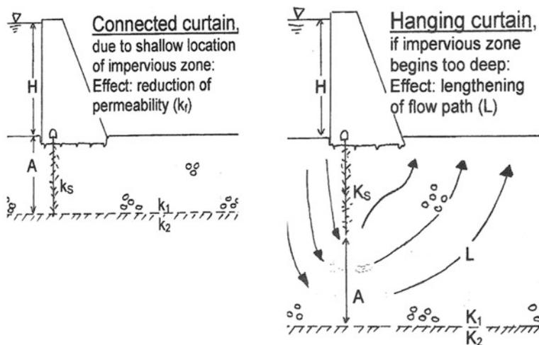
**Fig. 6.1** Connected curtain (*left*), hanging curtain (*right*) depending on depth of less permeable zone:  $k_1 > k_2 \approx k_s$
