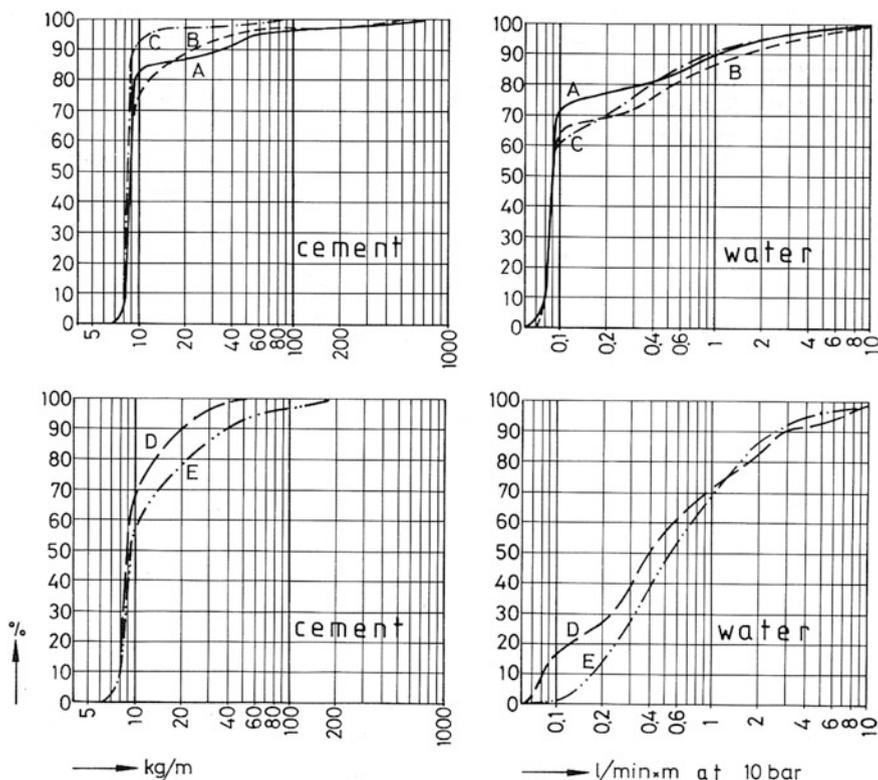
Fig. 3.5 Tavera Dam. Summation curves showing the relative frequency distribution
