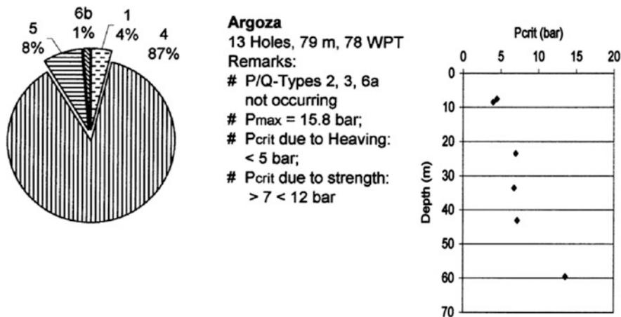
Fig. 5.10 Argoza. Portion of P/Q-Types (left) and relation P<sub>crit</sub>/Depth for Types 3 and 5 (right)
