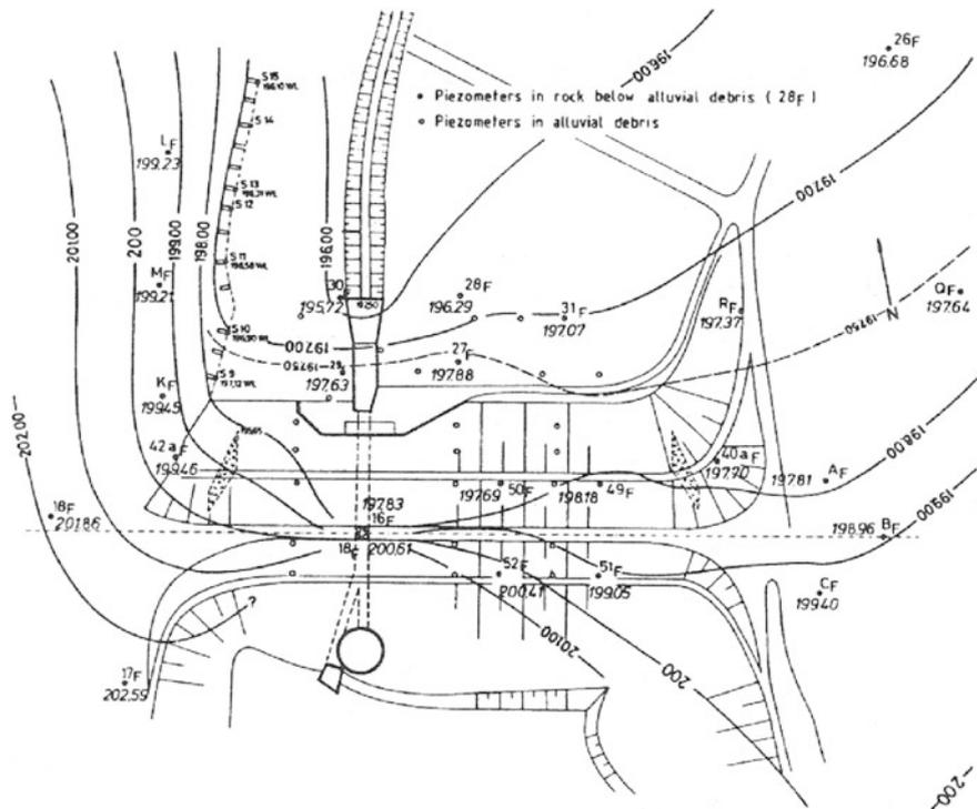
Fig. 7.7 Difference in reduction of uplift along the dam
