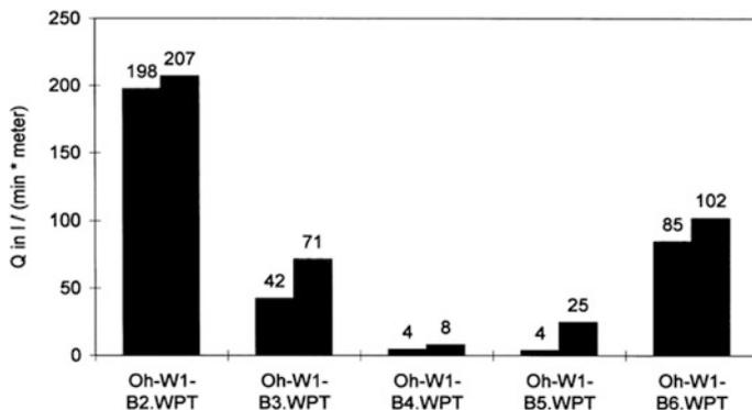
**Fig. 5.30** Differences between mean values of  $Q_{10}'$  (left) and  $Q_{10}^*$  (right) for WPTs carried out in single holes characterizing a section of individual permeability
