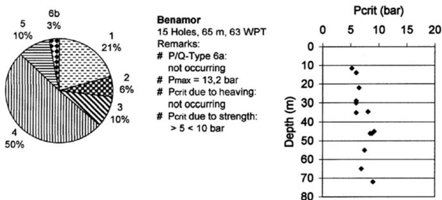
Fig. 5.12 Benamor. Portion of P/Q-Types (left) and relation  $P_{crit}$ /Depth for Types 3 and 5 (right)
