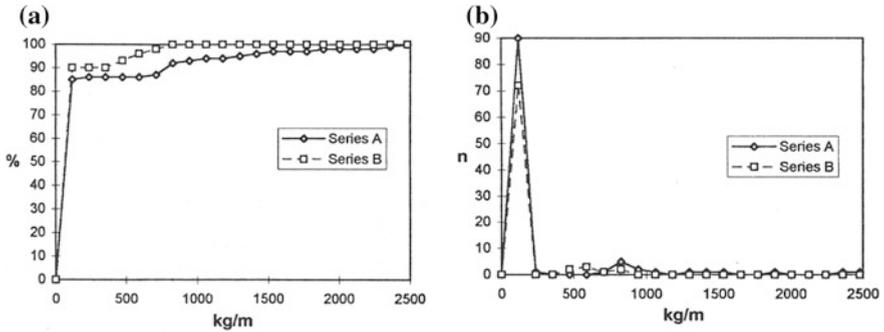
**Fig. 6.7** a Statistical evaluation of grout data obtained in Karstic limestone; the relative frequency distribution of all grout takes. b Absolute frequency distribution of all grout takes
