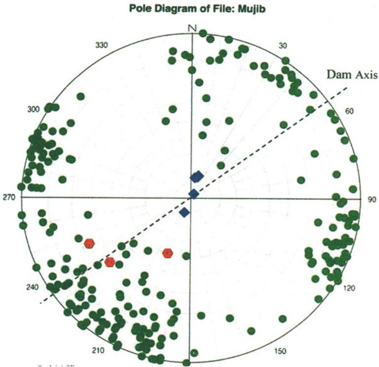
**Fig. 3.48** Mujib Dam. Density of joints; *bold line* dam axis: *green* joints, *blue* beddings, *red* faults
