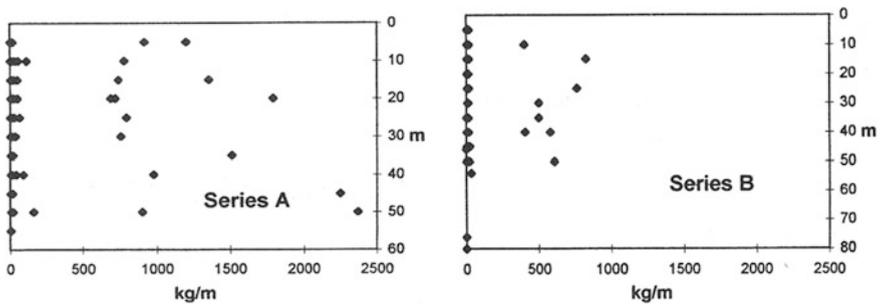
**Fig. 6.9** Distribution of individual grout takes related to depth; A = primary B = secondary
