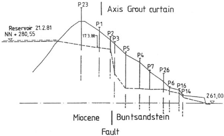
Fig. 7.6 Antrift Dam. Influence of a fault on the reduction of uplift
