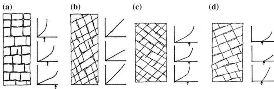
**Fig. 5.5** Factors ruling hydrojacking and hydrofracturing depend on the state of the rock bond; from **a** (left) to **d** (right)
