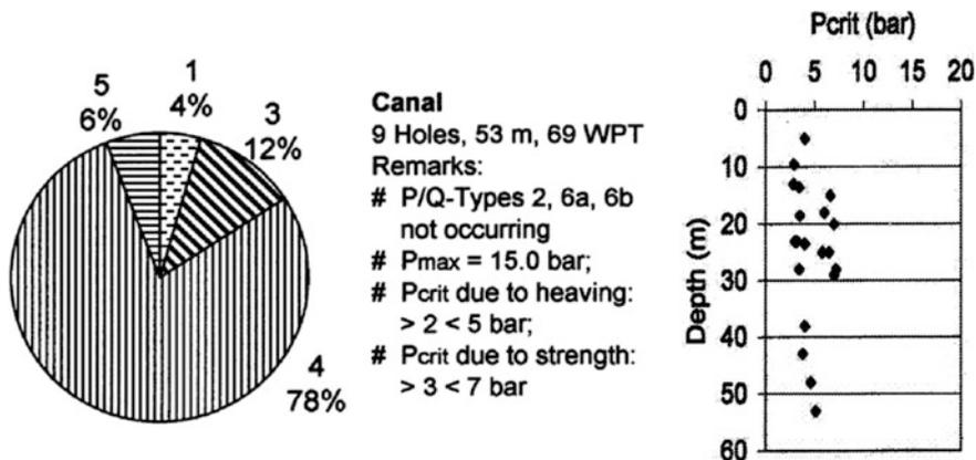
Fig. 5.14 El Canal. Portion of P/Q-Types (left) and relation  $P_{crit}/Depth$  for Types 3 and 5 (right)
