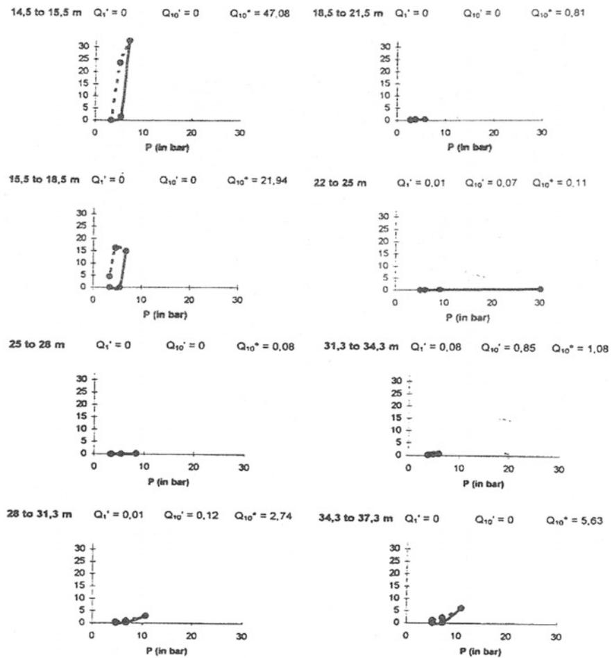
Fig. 3.30 Yuracmayo Dam. Hydrofracturing of latent bedding-like planes at pressures  $\leq 10$  bar hydrofracturing caused bad results
