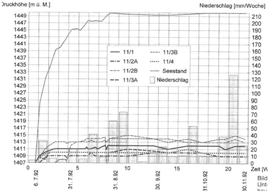
Fig. 3.45 Panix Dam. Hydraulic behaviour inside the dam—very little reaction due to rain
