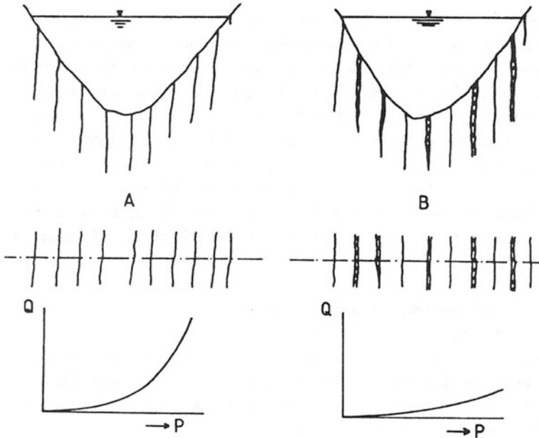
**Fig. 6.18** Groutstone pillows intercalated along vertical beddings, crossing the dam axis and being prone to hydrofracturing, may diminish fracturing and thus the over-proportionate increase of seepage
