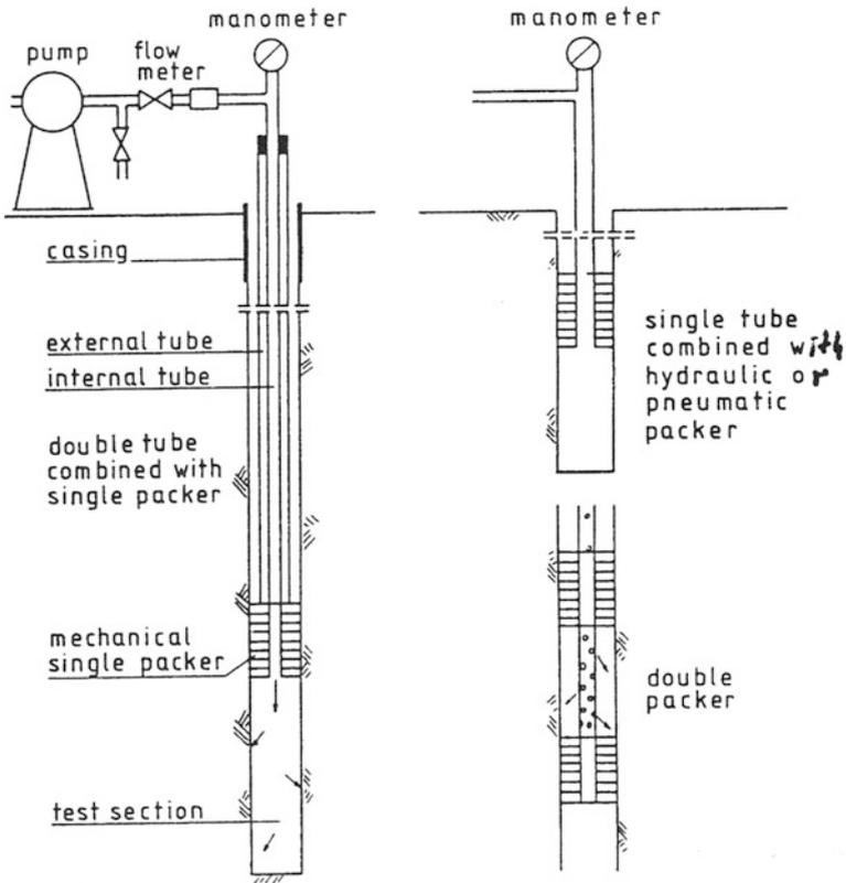
Fig. 4.1 Layout of water pressure test (WPT) considering different packer systems
