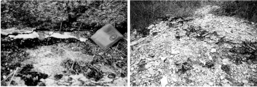
**Fig. 3.22** Almendra Dam. Grout suspension flew out of the surface of the slope and was deposited in layers of various centimetres in thickness
