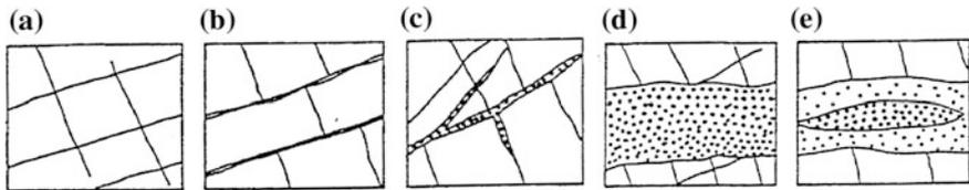
**Fig. 3.40** Pueblo Viejo Dam. Classification of rock regarding water routing, permeability, effectiveness of grout curtain altogether determining the form of uplift reduction
