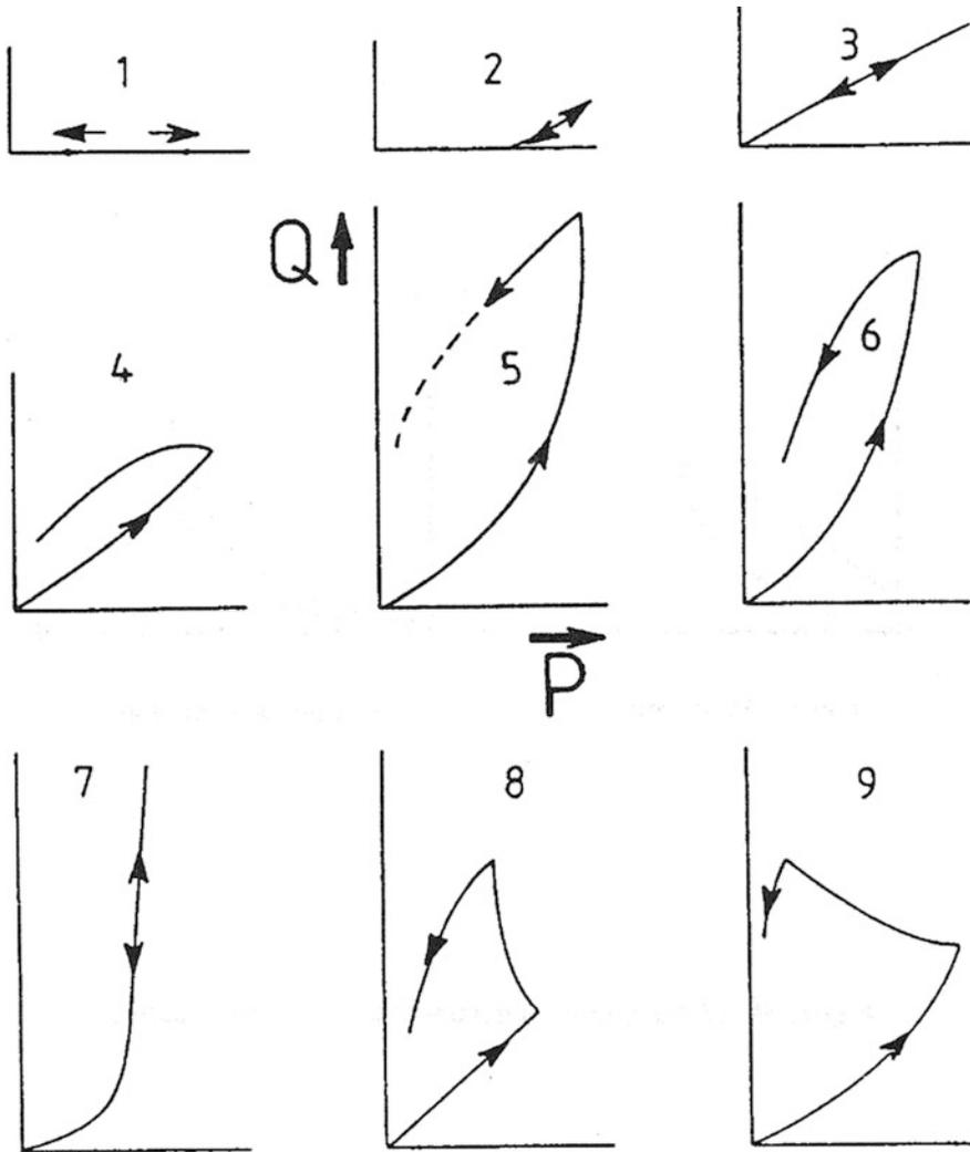
**Fig. 4.15** Selection of frequent P/Q-diagrams indicating different forms of deformation
