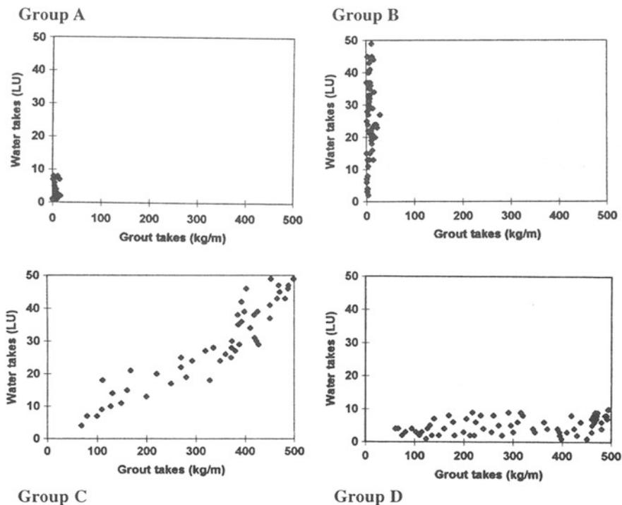
Fig. 6.10 Grouping of different relationships between WPT-results and grout takes
