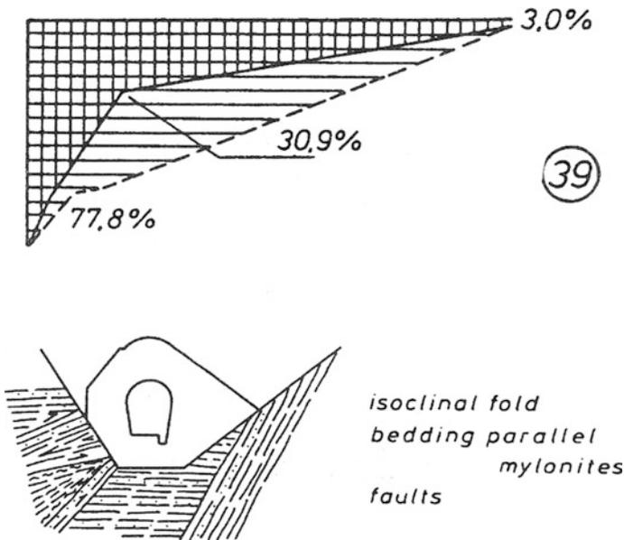
**Fig. 7.4** Aabach Dam Micro-features reduce uplift over-proportionately
