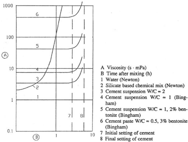
Fig. 6.17 Viscosity development of grouting materials, after Kutzner
