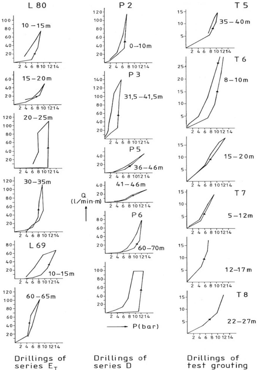
**Fig. 3.4** Tavera Dam: typical classification of P/Q-diagrams—tight rock sections are fractured and permeable sections are dilated
