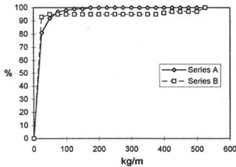
**Fig. 6.8** Statistical evaluation of grout data obtained in karstic limestone
