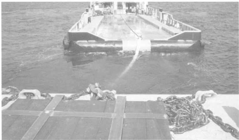
Figure 14.23 Typical arrangement of tow line and bridle
