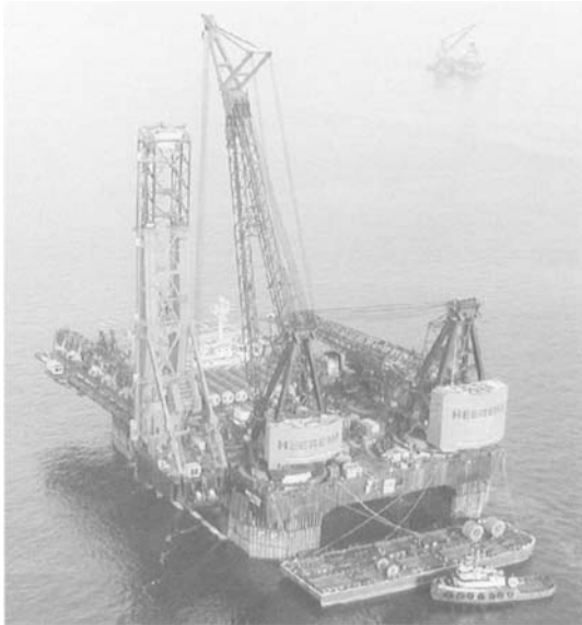
Figure 11.16 Heerema's balder in J-lay mode – Courtesy Heerema marine contractors
