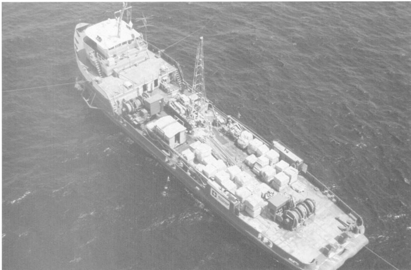
Figure 16.19 Typical supply vessel with skid mounted drill rig – M/V Perkins
