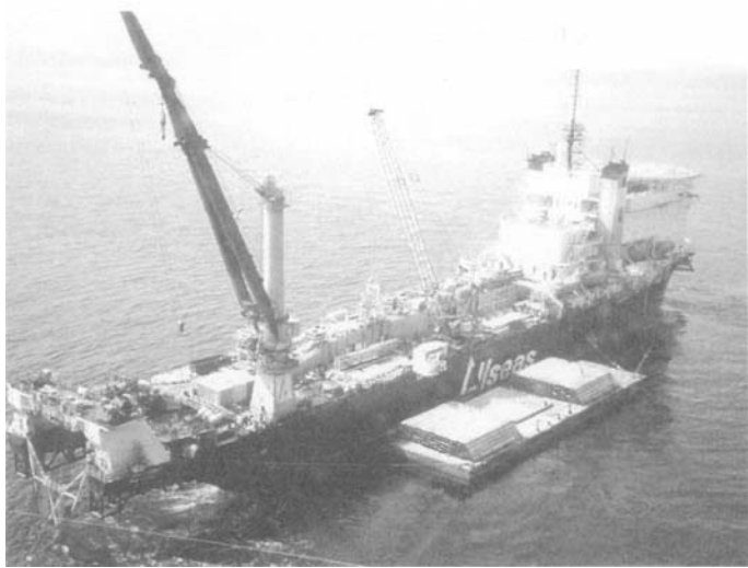
Figure 11.17 Allseas Lorelay S-lay vessel – Courtesy C. Langner
