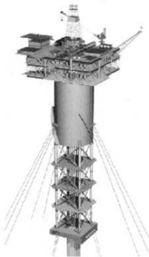
Figure 14.8 Schematic of a truss spar
