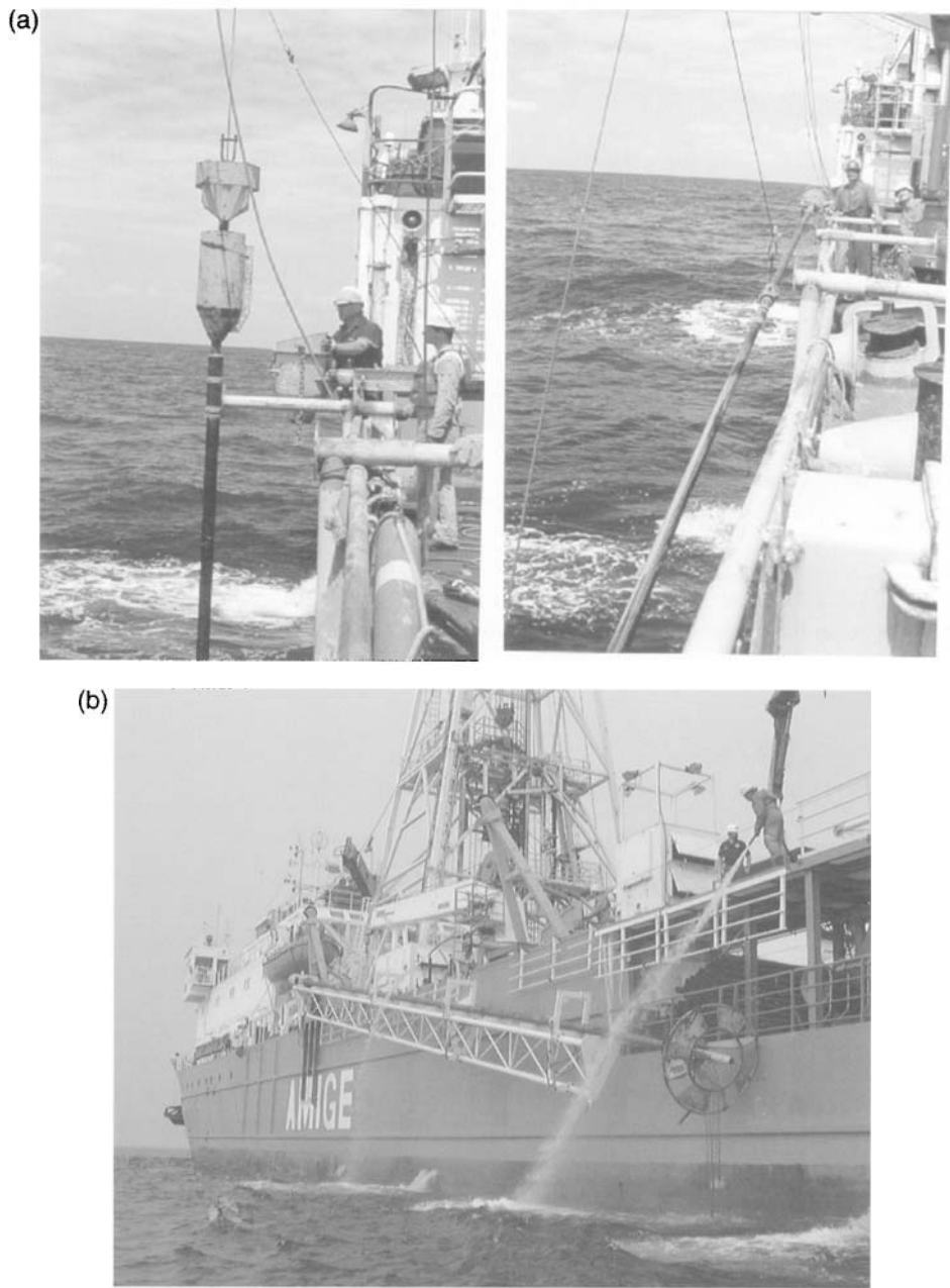
Figure 16.40 (a) Preparing a long piston corer for deployment and retrieving it to deck; (b) STACOR mega piston corer being deployed along side of vessel
