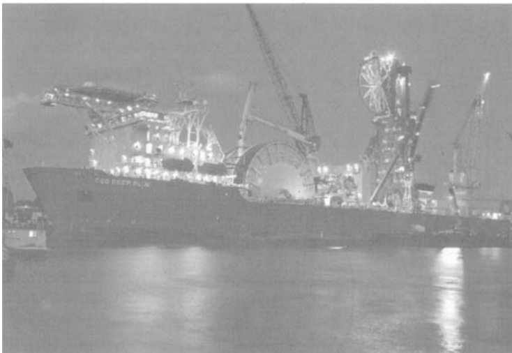
Figure 14.31 Deep Blue reel pipelay vessel
