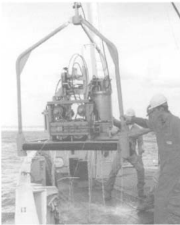
Figure 16.50 SEASCOUT minicone CPT and schematic
