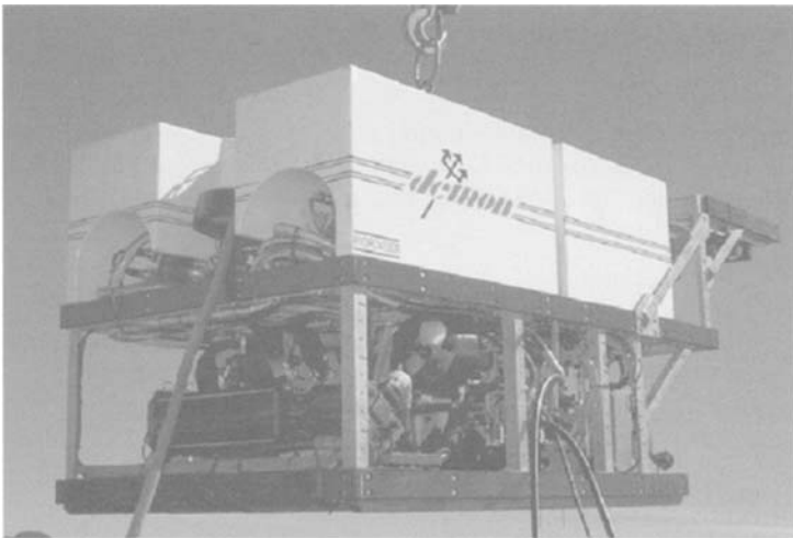
Figure 16.12 Example of an ROV (Sea Demon)
