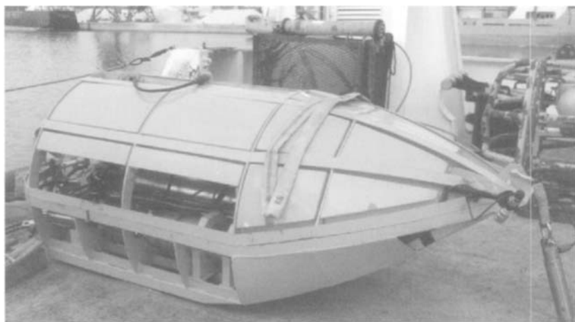
Figure 16.15 GAMBAS ® seismic refraction system – seabed tow sled
