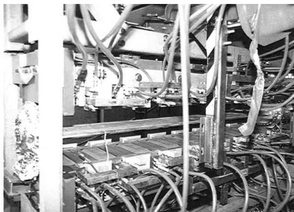
Fig. 24.3 Electromagnetic wiggler magnet with eight 1.8 T poles
