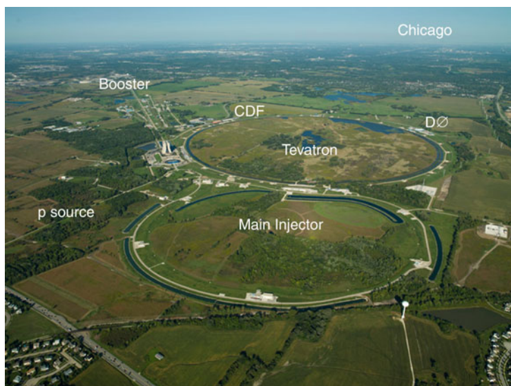
Fig. 6.2 The tunnel of the Tevatron is 6.8 km long. The Main Injector was built in the years 1993–1999 and has greatly contributed, with the upgrade of the antiproton source, to reaching the largest proton-antiproton luminosities ever obtained in a collider (Courtesy Fermilab Visual Media Services)
