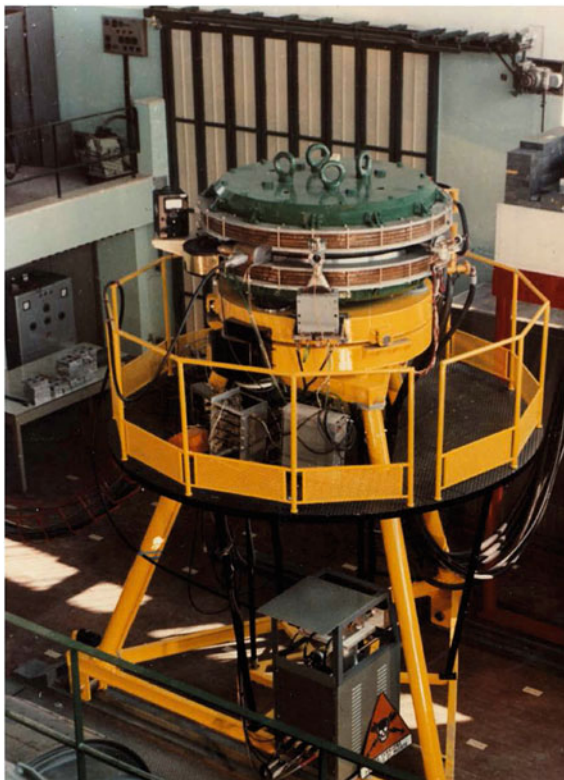
Fig. 3.4 The AdA ring was so small and light that, to alternately inject electrons and positrons coming from the same magnetic beam line, the magnet shown in the picture was rotated every few hours back and forth by 180^\circ around one of its diameters (Courtesy Istituto Nazionale di Fisica Nucleare, Frascati)
