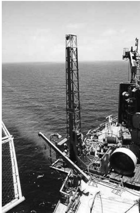
Figure 3.25 Conventional onshore drilling equipment operating over the side of a jack-up rig
