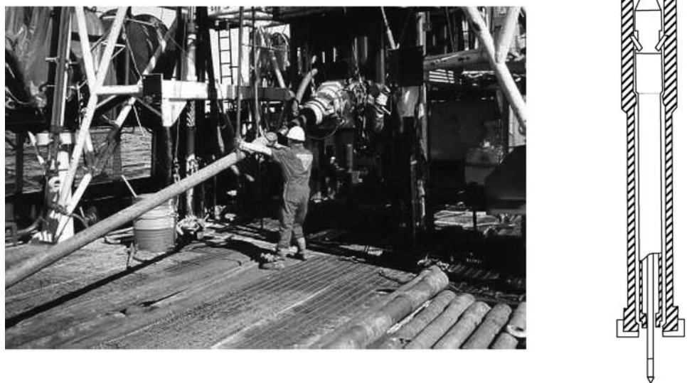
Figure 3.28 Drill bit and schematic of lower part of borehole assembly
