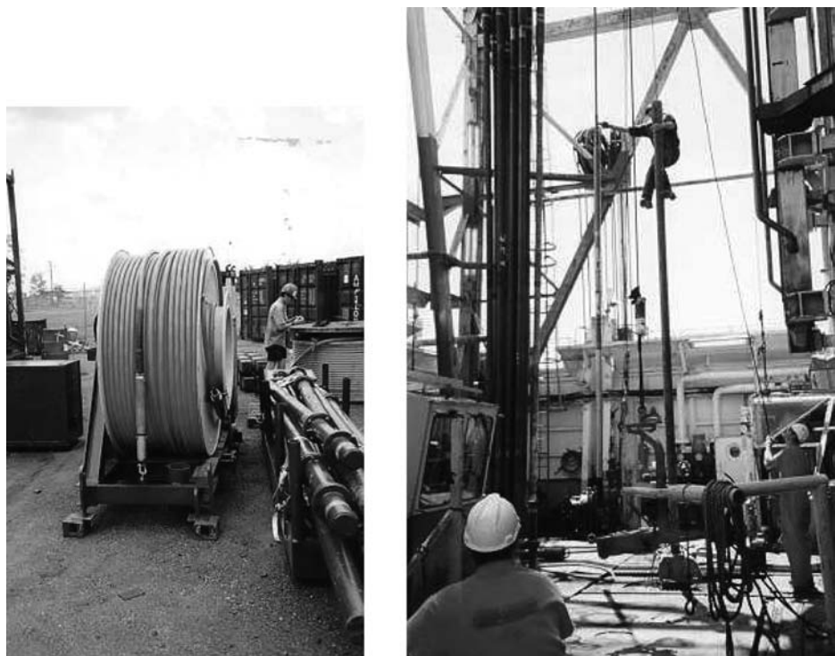
Figure 3.29 Umbilical cable and insertion of tool into drill stem
