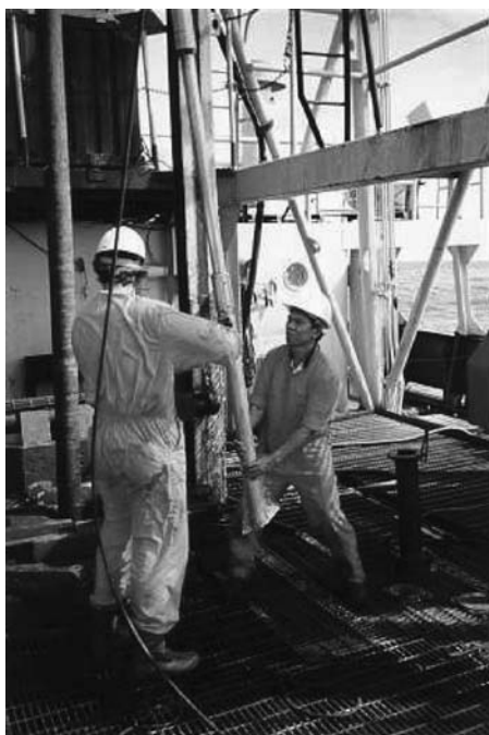
Figure 3.46 Removing the sampling tube from the piston corer
