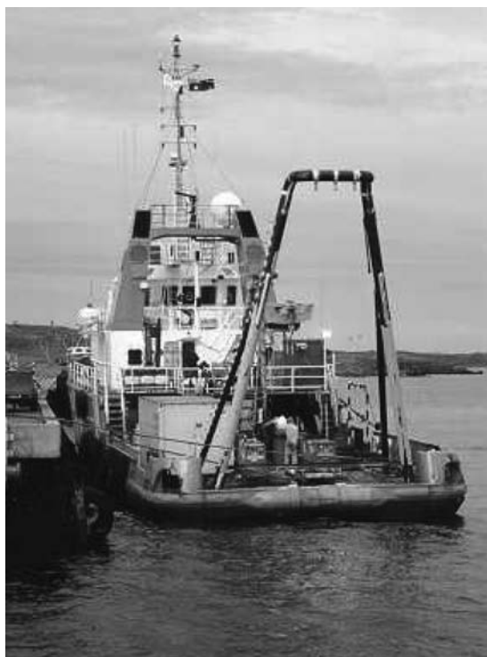
Figure 3.18 Support (or supply) vessel
