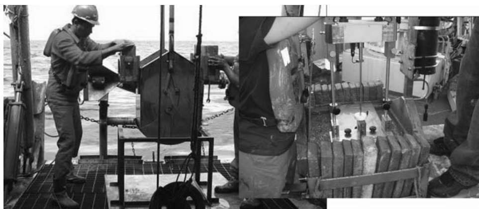
Figure 3.44 Box-core being landed and (right) set up for miniature T-bar penetrometer tests
