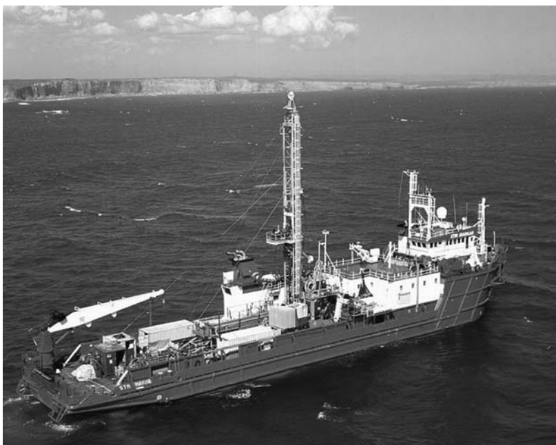
Figure 3.20 Specialised drilling vessel
