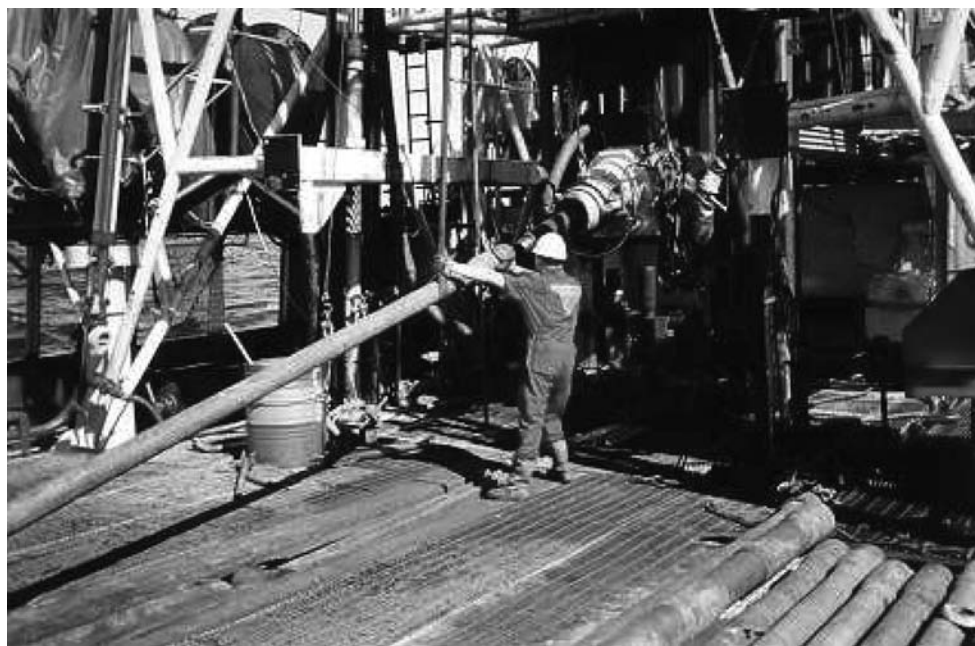
Figure 3.27 Standard 5" (127 mm) API drill string
