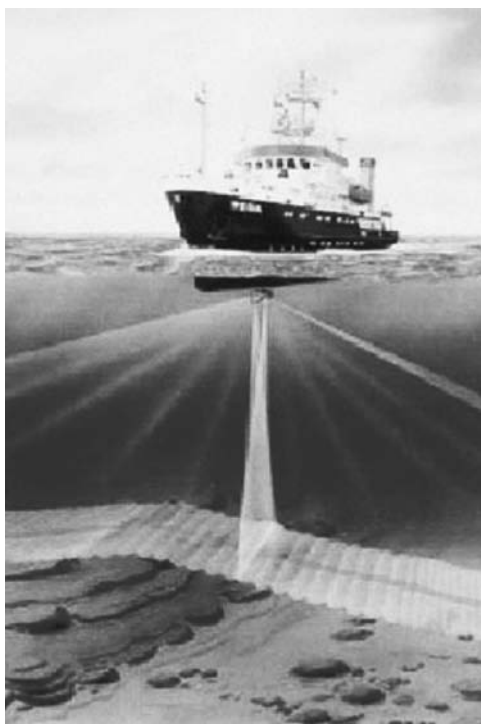
Figure 3.4 Schematic of swath bathymetry system
