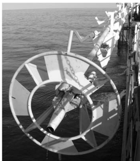
Figure 3.45 The STACOR gravity piston sampler. Reprinted from Borel, D., Puech, A., Dendani, H. and de Ruijter, M. (2002) 'High quality sampling for deep-water geotechnical engineering: the STACOR® Experience'. Ultra Deep Engineering and Technology , Brest, France, by kind permission of PennWell Conferences and Exhibitions.
