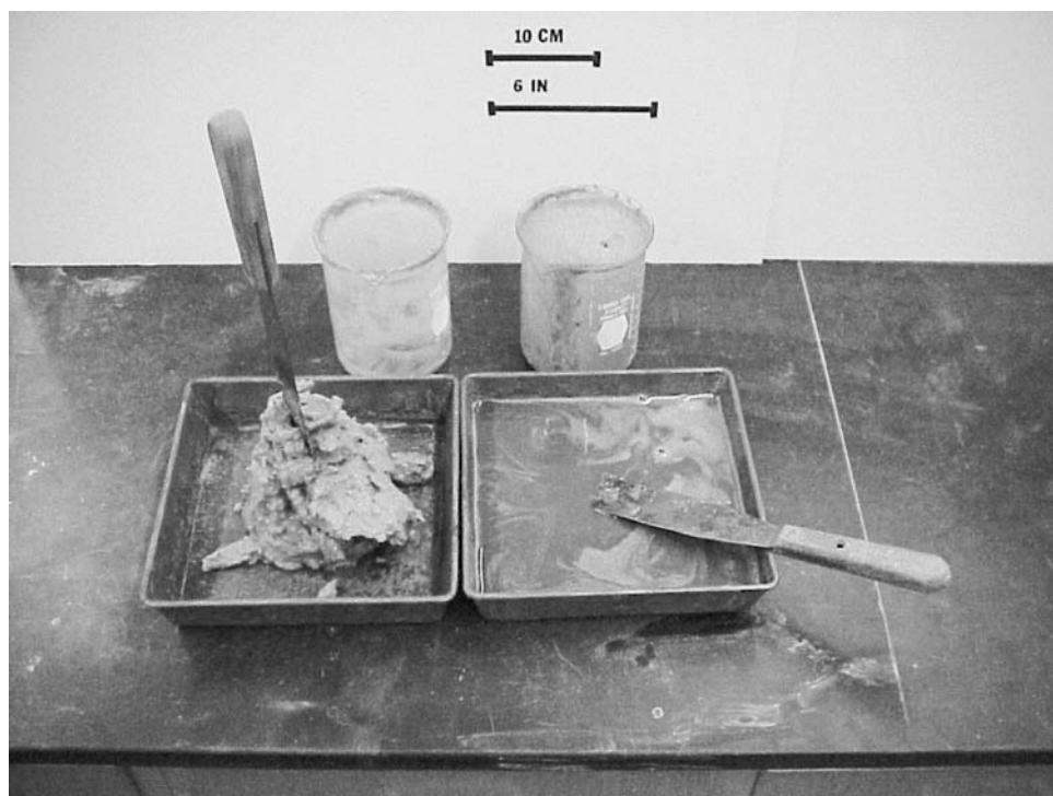
Figure 2.11 Effect of saline pore water on soil strength: salt water (left) and freshwater (right) (Elton 2001)
