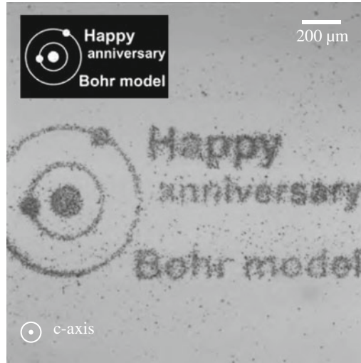
Fig. 6.5 Electrophoretic trapping of charged GC particles suspended in NOVEC 7500 in arbitrary patterns on a z-cut lithium niobate; inset shows the desired pattern, honoring the 100th anniversary of Bohr's semiclassical shell model (also published in [19])
