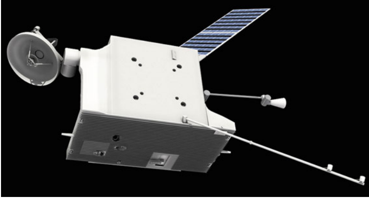
Fig. 3.9 MPO deployed for orbit about Mercury. The lower face is the 3.7 m long radiator panel, which will always face the planet and never be allowed to receive direct sunlight (ESA)
