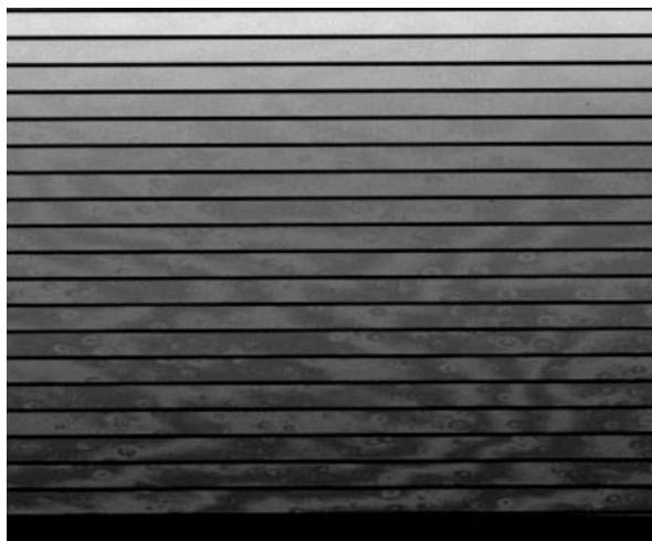
Fig. 1.5 Fringing in a CCD. Shown are spectral orders of an echelle spectrum (see below) of a white light source. Spectral orders with blue wavelengths ( \approx 5000 \text{ \AA} ) are at the top , red orders ( \approx 7000 \text{ \AA} ) are at the bottom . Fringing is more evident in the red orders
