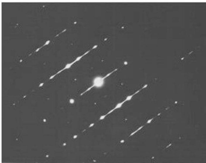
Fig. 11.4 An electron diffraction patterns taken from the CuZnAl alloy sample
