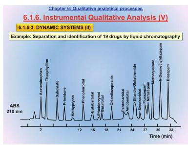
This slide illustrates the potential of liquid chromatography for multi-identification with the separation and identification of 19 drugs in human serum. Although some peaks in the chromatogram are overlapped, their retention times are different enough for qualitative identification purposes.
