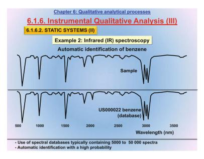
This slide illustrates the automatic identification of benzene by infrared (IR) absorption spectroscopy, which is a widely used technique for qualitative analytical purposes.
