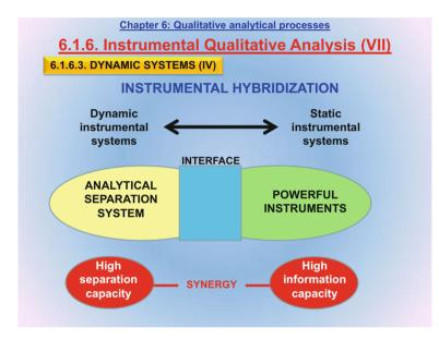
So-called *instrumental hybridization* is the synergistic combination of two or more instrument systems in order to boost their individual qualitative and quantitative information potentials. The key to an effective connection here is finding an appropriate interface with a view to maximizing analyte separation and information production.
