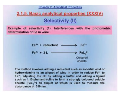
This colorimetric method for determining the amount of iron in wines involves a preliminary operation by which  $Fe^{3+}$  is reduced to  $Fe^{2+}$ ; then, ferrous ion forms a coloured chelate L that is detected and quantified with a photometer.
