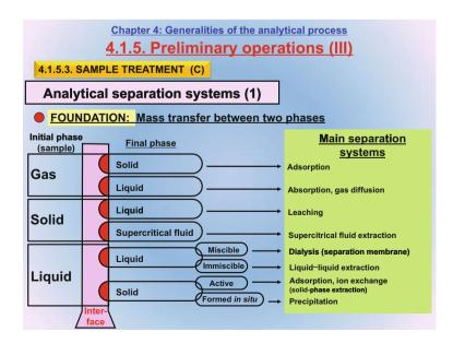
Analytical separation systems, often referred to as "analytical separation techniques" (ASTs) (see Slide 1.32), are extremely important in Analytical Chemistry because they help improve two essential properties: sensitivity and selectivity. Some authors have claimed that the history of Analytical Chemistry can be traced through progress in the development of separation systems.
