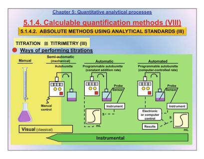
Automation has also reached titrations and titrimetries. In the process, formerly manual work has been rendered automatic. This slide compares three different types of autoburettes with a classical burette.
