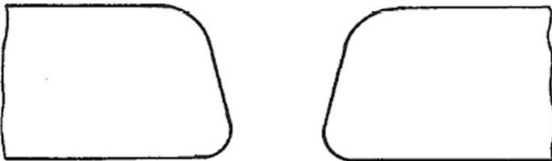
**Fig. 16** Rounded-corner effects in excessive-power laser drilling of FRPs (Abrate and Walton 2016)
