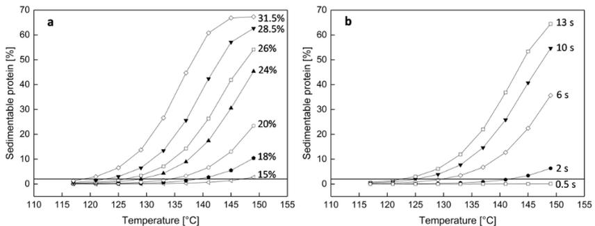
Fig. 10-1: Calculation of the expected relative amount of sedimentable protein based on the kinetic data of section 7.3 for direct steam injection heat treatments performed and investigated by Dumpler and Kulozik (2016) plotted over heating temperature and total solids (a) at a holding time of 9.5 s and depending on holding time at 27% CSM total solids.
