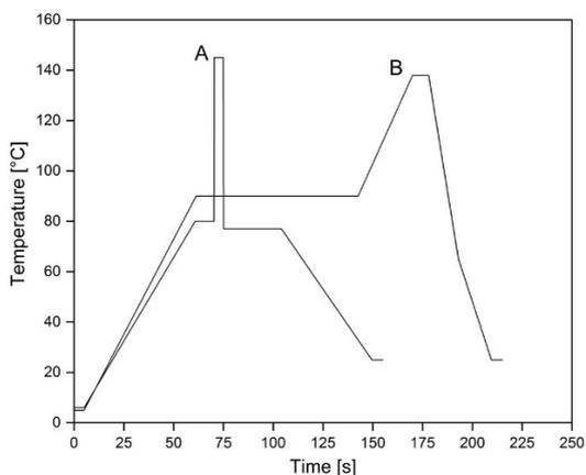
Fig. 1-12: Exemplary temperature-time profiles of direct (A) and indirect (B) UHT plants.
