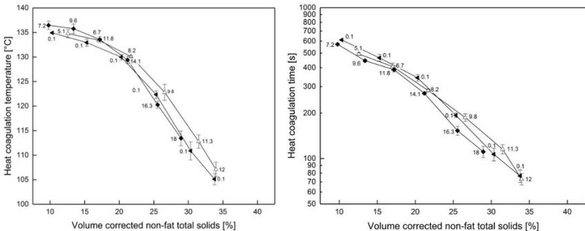
Fig. 9-5: Visually determined heat coagulation temperature (*left*) and heat coagulation time (*right*) of concentrated milk containing various proportions of milk fat depending on the volume corrected non-fat total solids. Data labels represent the relative proportion of milk fat based on the total volume of concentrated milk.
