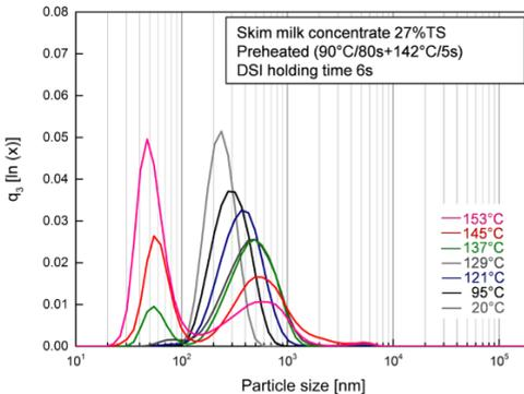
Fig. 4-6: Logarithmic density distribution  $q_3[\ln(x)]$  of the supernatant from preheated concentrated skim milk (27%TS) heat treated by direct steam injection at different temperatures measured by photon correlation spectroscopy (PCS).
