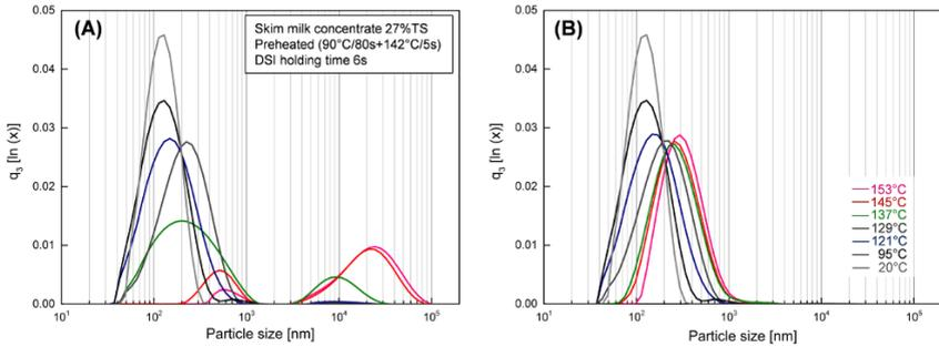
Fig. 4-5: Logarithmic density distribution  $q_3[\ln(x)]$  measured by laser light diffraction of concentrated skim milk (27%TS, preheated milk) heat treated by direct steam injection at different temperatures. Large protein aggregates included in the distribution (left) could be completely removed by centrifugation at  $4,000\times g$  for 10 min. Particle size distributions of the resulting supernatant is shown on the right.
