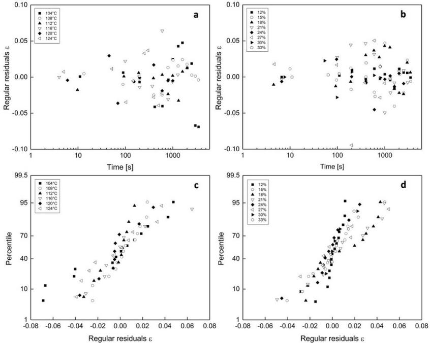
Fig. 7-8: Regular residuals of the Weibullian model fitted to the data of relative amounts of sedimentable protein of total protein for the dataset of different temperatures at a constant CSM total solids content of 27% (a) and at 116°C heating temperature for different total solids content (b). Panels (c) and (d) show the normal probability plots of the residuals.
