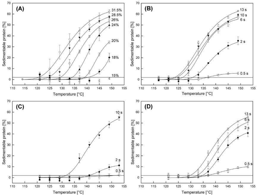
Fig. 4-7: Sedimentable aggregated protein of concentrated skim milk of different total solids at 9.5 s holding time (A), at different holding times at constant total solids content of 27% (B), 23% (C), and CSM of 27 % total solids made from UHT preheated milk (D). The onset of coagulation is indicated by a threshold level of 2% aggregated protein of total protein. Data points were fitted by a Gompertz model.
