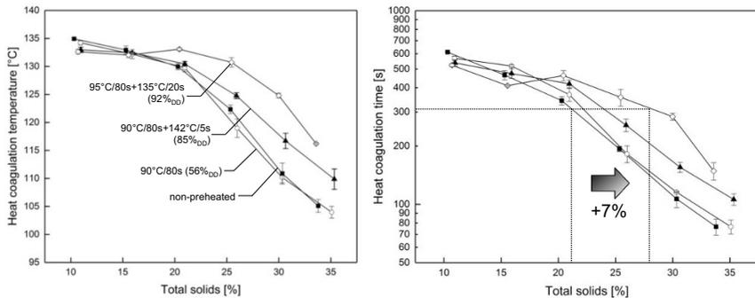
Fig. 9-3: Visually determined heat coagulation temperature (*left*) and heat coagulation time (*right*) of concentrated skim milk on lab scale depending on the total solids content. The preheat treatment conditions of unconcentrated milk before concentration by RO are indicated. The resulting degree of denaturation (DD) is also indicated in brackets.
