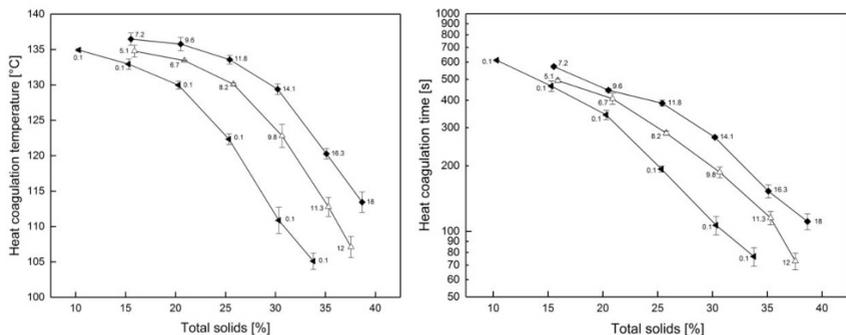
Fig. 9-4: Visually determined heat coagulation temperature (*left*) and heat coagulation time (*right*) of concentrated milk containing various proportions of milk fat depending on the total solids content. Milk fat was added as unhomogenised cream. Data labels represent the relative proportion of milk fat based on total volume of concentrated milk.
