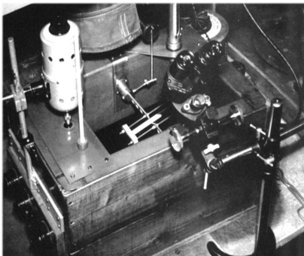
Fig. 1-13: Copper plated thermostatic paraffin bath used for the subjective heat stability test of Davies and White (1966). The sample tube attached to the carriage and the eccentric rocking the tube, a microscope (magnification 8.4), the immersion heaters (left), the stirrer and the thermometer indicating the paraffin bath temperature (left), and the thermometer for regulating the temperature (rear right-hand corner) are shown. The lamp illuminating the sample tube is not shown.<sup>5</sup>
