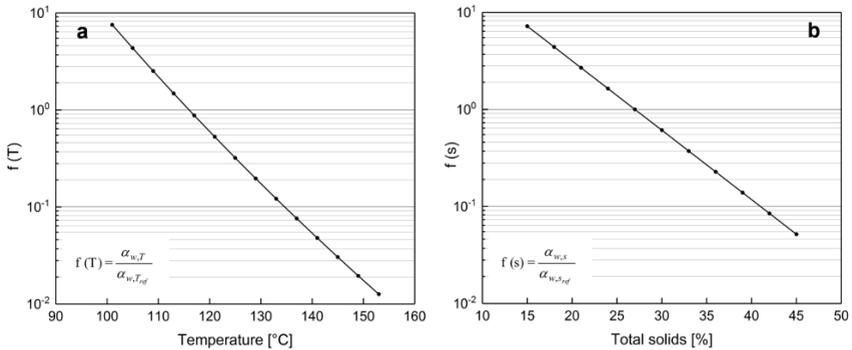
Fig. 10-3: Calculated data for the factor  $f_T$  depending on temperature (a) and  $f_s$  depending on total solids content of CSM (b).
