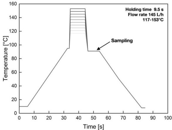
Fig. 4-2: Temperature-time profiles of the direct steam injection ultra-high temperature (UHT) pilot plant. Final product temperature was varied in steps of 4°C by adjustment of the steam pressure.
