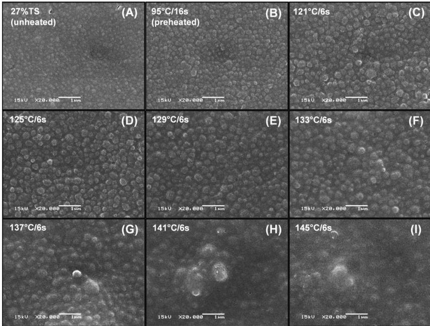
Fig. 4-4: Scanning electron micrographs of supernatants of concentrated skim milk. Unheated (A), indirect heat treated without steam injection (B) and heated by direct steam injection at different temperatures from 121 °C (C) to 145 °C (I) at a constant holding time of 6 s. Magnification of all pictures was kept constant at 20,000x.
