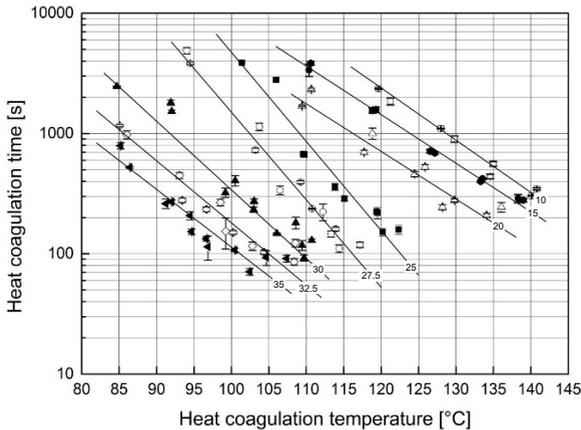
Fig. 9-1: Correlation between milk sample temperature and time of coagulation of concentrated skim milk of different total solids content. The total solids content is indicated on the regression lines (Dumpler and Kulozik 2015).
