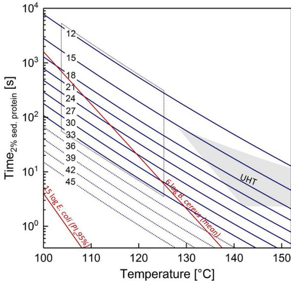
Fig. 9-2: Iso-effect lines for CSM for a critical level of 2% of sedimentable protein of total protein depending on heating temperature, heating time, and total solids content of bulk CSM (section 7.3)
