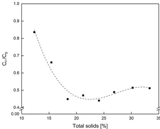
Fig. 7-2: Variation of the parameter  $a$  which represents the lower asymptote  $\frac{C_{\infty}}{C_0}$  of the Weibullian model depending on total solids.
