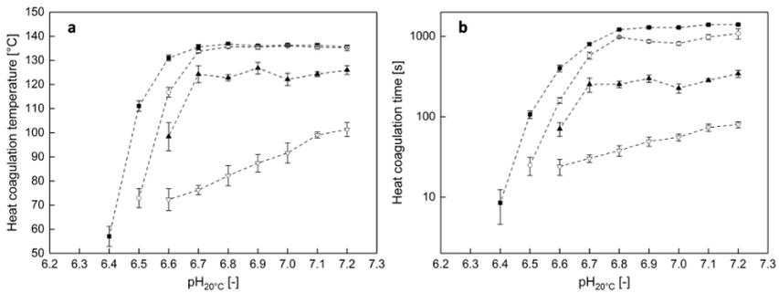
Fig. 8-5: Heat coagulation temperature (a) and heat coagulation time (b) of MCC depending on pH and addition of 0 (■), 1 (○), 2 (▲), and 3 mM (▽) soluble calcium as calcium chloride.
