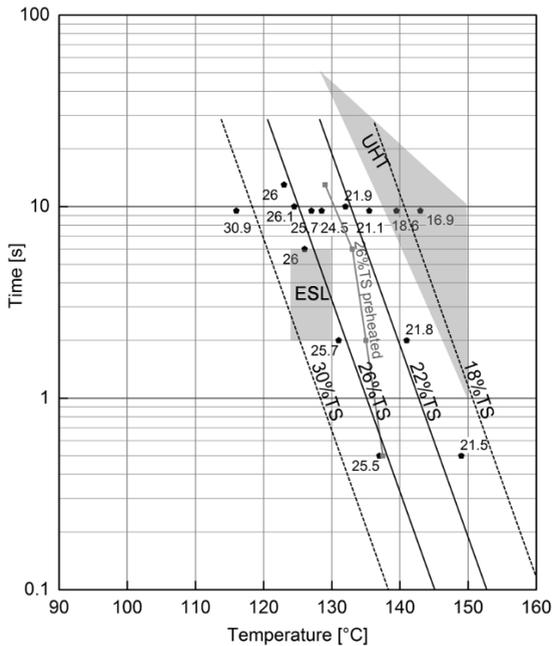
Fig. 4-8: Iso-effect lines of the onset of coagulation (2% of sedimentable protein of total protein) of concentrated skim milk heated by direct steam injection plotted on a semi-logarithmic scale. The 2% level of sediment for forearmed milk is indicated. The working areas used for ESL and UHT treatment of unconcentrated milk are shown for orientation.
