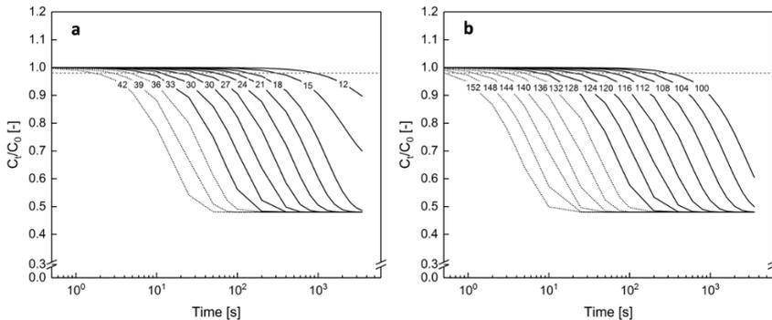
Fig. 7-5: Simulation of the relative amount of non-sedimentable protein depending on CSM total solids at 116 °C (a) and 27% CSM total solids depending on heating temperature over time on a logarithmic scale (b). A critical level of 2% of sedimentable protein of total protein indicates the onset of coagulation (*dashed lines*). Calculations based on extrapolated data are also shown (*dotted lines*).
