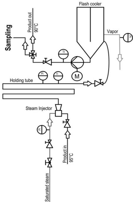
Fig. 4-1: Simplified P&I diagram of the pilot plant unit for direct steam injection heat treatment of concentrated skim milk preheated to 95 °C by indirect heat exchange prior to steam injection. Sample aliquots were taken immediately after flash evaporation of the concentrate.
