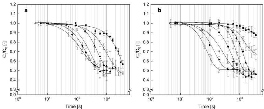
Fig. 7-1: Relative amount of sedimentable protein over the logarithmic heating time depending on heating temperature at 27% CSM total solids (a) and depending on total solids at 116 °C (b) fitted by the Weibullian model. Heating temperatures (*left*) were 104 (■), 108 (○), 112 (▲), 116 (◁), 120 (◆), and 124 °C (▽). Total solids content of the CSM (*right*) was 12 (■), 15 (○), 18 (▲), 21 (▽), 24 (◆), 27 (◁), 30 (▲), and 33% (○).
