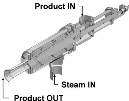
Fig. 1-11: Patented steam injector having three annular steam inlets and an adjustable mandrel to control the velocity of the product flow, bored spacers in stainless steel for the steam inlets, bevelled contact surfaces for the steam inlet into the product, and PEEK material for all product contact surfaces. Noses are forcing higher product velocities which improves the injection effect (Kowalik et al. 2007)<sup>4</sup>.
