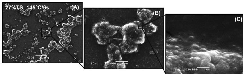
Fig. 4-3: Scanning electron micrographs of protein particles formed during direct steam injection heat treatment of concentrated skim milk at 145 °C. Magnification increases from left to right. (A) 350x, (B) 2,000x, (C) 20,000x.
