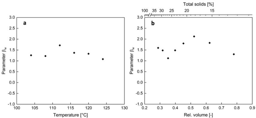
Fig. 7-3: Parameter  $\beta_w$  of the Weibullian model obtained by non-linear regression of sedimentable protein depending on heating temperature (a) and total solids content or the relative residual volume of the concentrate compared to unconcentrated skim milk (b).
