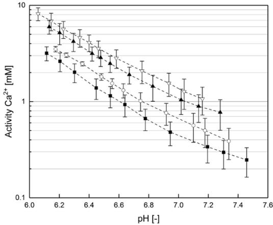
Fig. 8-6: Calcium activity in MCC depending on pH and addition of 0 (■), 1 (○), 2 (▲), and 3 mM (▽) calcium as calcium chloride.
