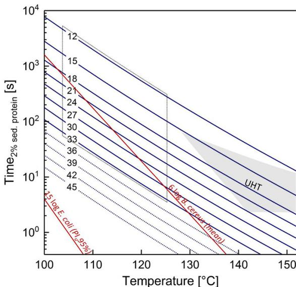
Fig. 7-6: Iso-effect lines for CSM for a critical level of 2% of sedimentable protein of total protein depending on heating temperature, heating time, and total solids content of bulk CSM. The time-temperature range covered by experiments (dotted area), extrapolated total solids contents (dotted lines) are shown. The UHT region (grey area) and certain microbial inactivation levels are indicated for orientation.
