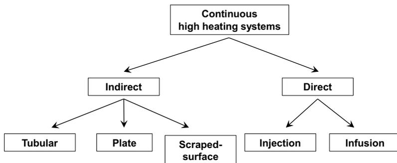
Fig. 1-9: Different types of continuous high heating systems using hot water or saturated steam as a heat transfer medium.
