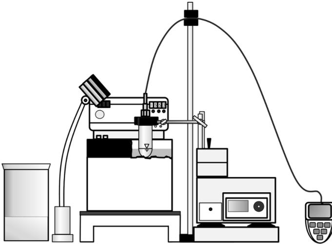
Fig. 3-1: Assembly used for determination of heat stability of unconcentrated and concentrated milk of different total solids content. Testing equipment consists of an ice-water mixture for sample cooling, an oil bath for sample heating, a lamp, a shaker equipped with a support for fixation of the screw capped round bottom borosilicate tubes and an ALMEMO® 2590-4S to record time, temperature and pH during a trial.
