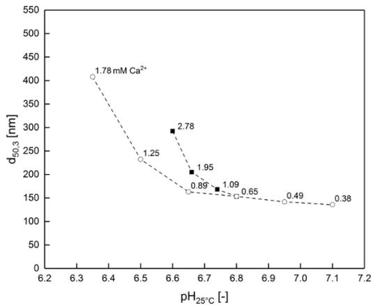
Fig. 8-9: The maximum  $d_{50,3}$  of heat treated MCC depending on pH. The change in calcium activity was obtained by addition of calcium chloride (■) or adjustment of pH (○). Data captions indicate the determined calcium activity MCC at 25 °C.
