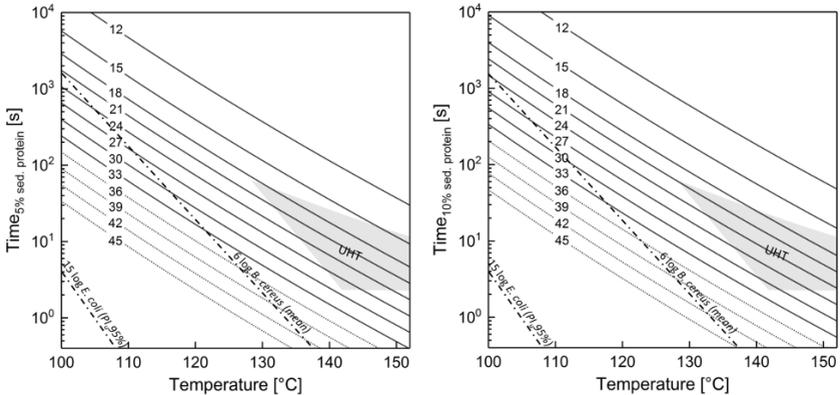
Fig. 10-2: Iso-effect lines for CSM for a critical level of 5% (left) and 10% (right) of sedimentable protein of total protein depending on heating temperature, heating time, and total solids content of bulk CSM. Extrapolated total solids contents (dotted lines) are shown, the UHT region (grey area) and microbial inactivation levels for *B. cereus* and *E. coli* (95% upper probability interval) are indicated for orientation (van Asselt and Zwietering 2006).
