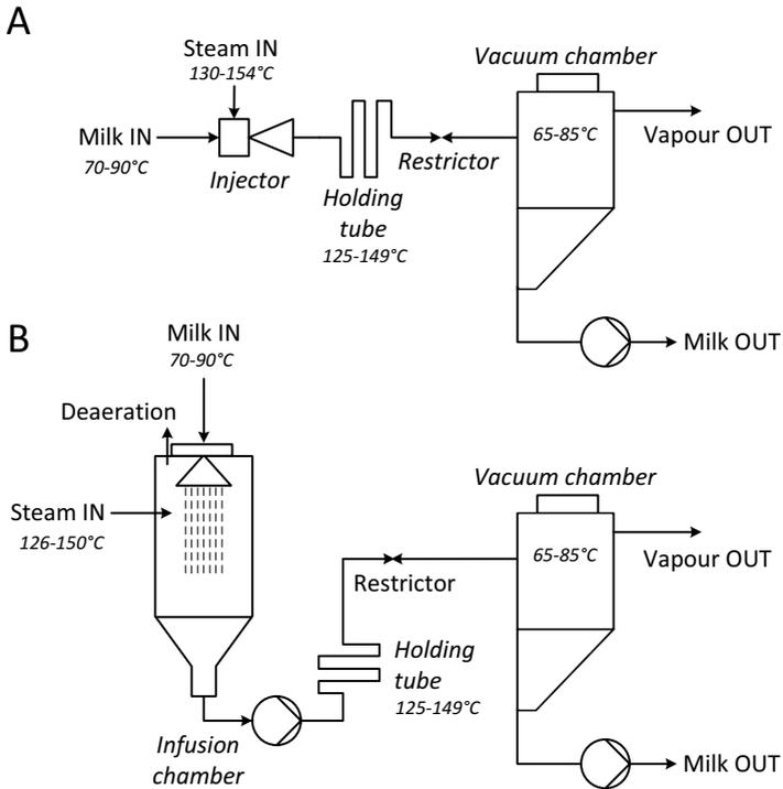
Fig. 1-10: Principle of operation of direct heating systems; (A) direct steam injection, (B) direct steam infusion (Burton 1994).
