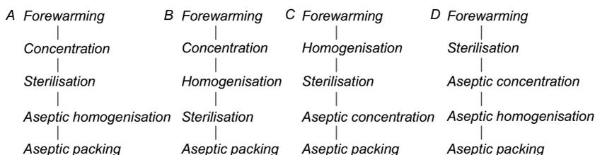
Fig. 1-17: Processing alternatives for the manufacture of evaporated milk or concentrated sterile milk in general using the UHT process for sterilisation. The term 'forewarming' is equivalent to preheating of unconcentrated milk before concentration (Muir 1984).
