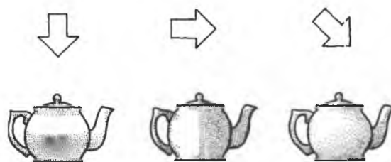
5.10 Strength and direction of flow. Usual lighting preference for pleasant modelling of objects and visual comfort is as shown on the right, oblique and with helpful but not excessive contrast
