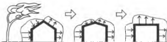
2.2 Loads from wind. Apart from buffeting turbulence, the house profile induces pressure and suction in the moving airflow
