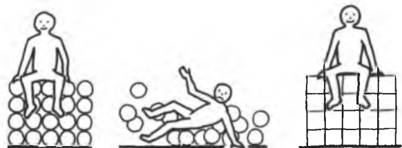
1.6 Masonry is more stable and strong if well fitted . . .
