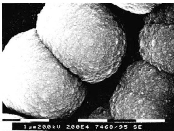
Fig. 4.20 SEM image of the cauliflower structure of silicon deposited for 10 min with 1 % \text{SiH}_4 –1 % \text{HCl} –98 % \text{H}_2 gas mixture, 1123 K substrate temperature, and 100 torr reactor pressure (Hwang et al. 2000)
