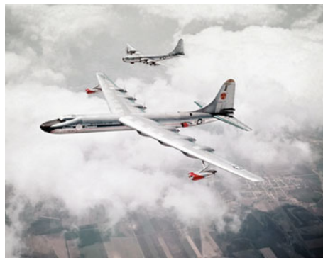
Fig. 4.6 Nuclear Airplane. In the 1950s the US modified a B36 bomber to carry a 3 MW nuclear reactor. The reactor operated for 36 h, without actually flying the plane (Department of Defense)
