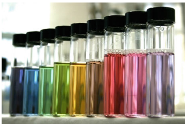
Fig. 2.11 Nanoparticles of various shape and size in solution—the plasmonic resonance determines the color (Photo with kind permission from Carsten Sönnichsen, http://www.nano-bio-tech.de/ )
