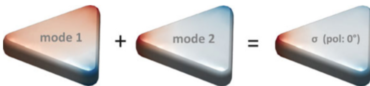
Fig. 3.8 The linear combination of the first two (degenerate) dipolar eigenmodes of an equilateral triangle generates the surface charge distribution plotted in Fig. 3.5
