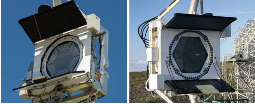
Fig. 3.3 Left Front of the MAGIC-I camera (before the upgrade) with two types of PMTs visible. Right Closeup of the MAGIC-II camera. Credit The MAGIC Collaboration
