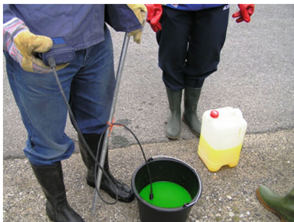
Fig. 12 Tracer preparation, conductivity measurement
