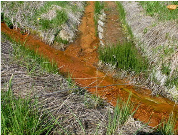
Fig. 9 Outflow of the Sedem Žien setting-pit percolating water from the bottom of the dam (samples V-3 and V-4)
