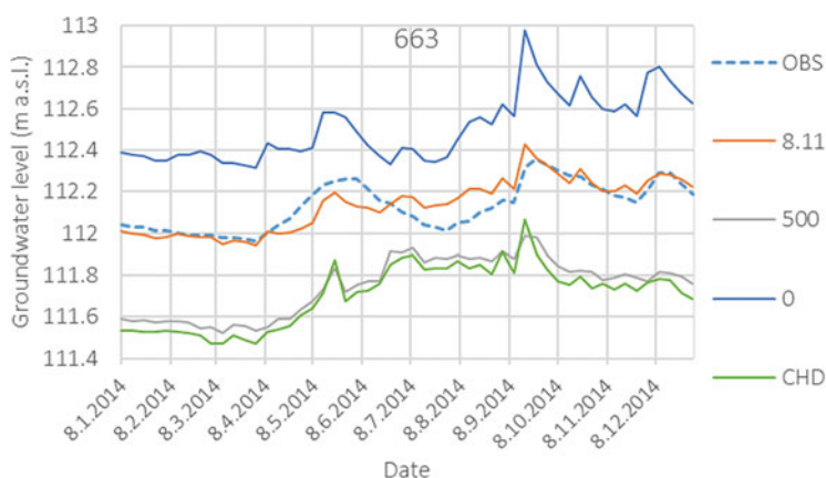
Fig. 19 Measured and simulated groundwater levels for observation probe 663
