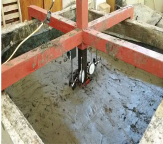
Photo 5 Soil settlement after loading
