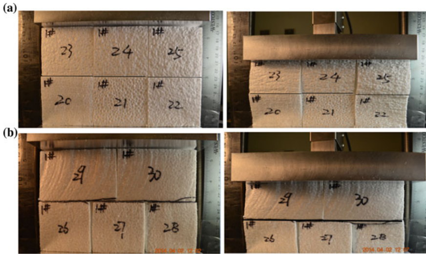
Fig. 8 a Uniform density stacked in 2 layers with continuous vertical joints, b uniform density stacked in 2 layers without continuous vertical joints; before (left) and after (right) loading
