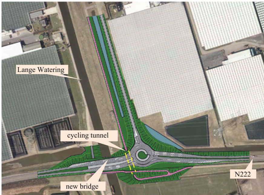
Fig. 1 The realized double-lane roundabout between the Wateringveldse polder and the regional road N222 (=the auction route)
