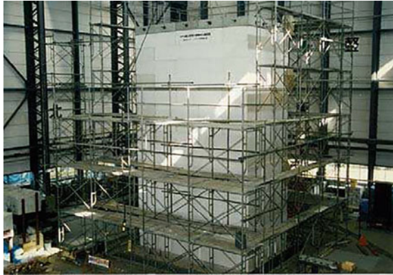
Fig. 2 8.5-m high free-standing EPS embankment test conducted by EDO and Hokkaido CERl in Japan Tsukamoto [3]
