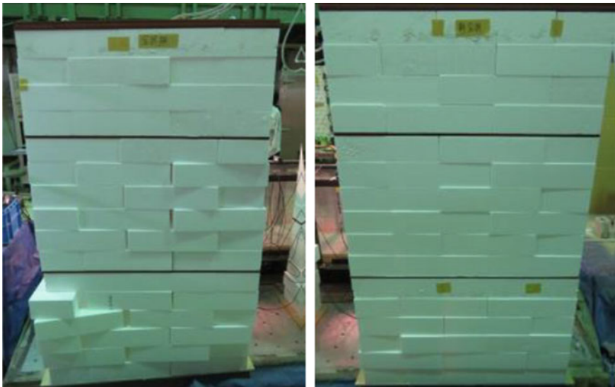
Fig. 5 Picture of EPS embankment after test—left: no JMBs—right: new JMB arrangement
