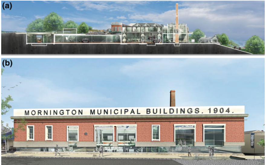
Fig. 9 a Final design showing north-south sectional perspective/underpass. b Final design showing raised 1903 part of the Mornington Cable-Car Depot building above the original 1882 basement, with gap between. Renderings by Author
