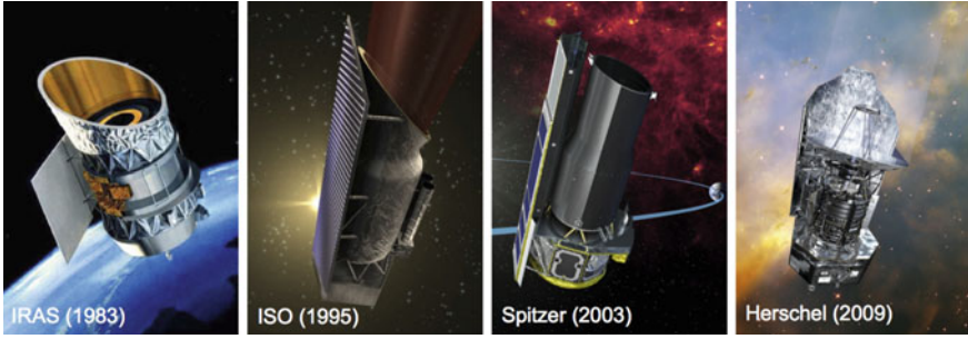
Fig. 1.4 FIR instruments in chronological order from left to right IRAS (1983), 0.6-m dish cooled at 2 K and operating at 12, 25, 60 and 100 \mu\text{m} ; ISO (1995), 0.6-m dish cooled at 2–3 K operating in the band 3–200 \mu\text{m} ; Spitzer (2003), 0.85 m dish cooled at 4 K operating in the band 3–180 \mu\text{m} ; Herschel (2009), 3.5-m dish cooled at 80 K operating in the band 55–670 \mu\text{m} . [ Credit , respectively: NASA/JPL; ESA; NASA/JPL-Caltech; ESA/AOES Medialab, background from Hubble Space Telescope image (NASA/ESA/STScI)]
