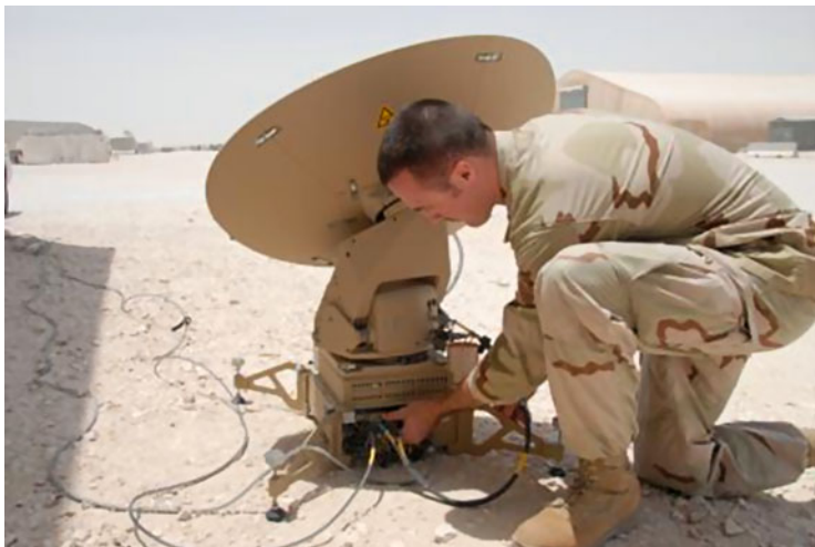
Fig. 4.5 A portable VSAT system in use by a U.S. military unit ( http://www.dvidshub.net/image/50091/vsat-helps-eod-save-lives-time#.Upo_dmR4ajd )
