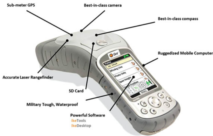
Fig. 6.5 IkeGPS hand-held integrated data collection system (Image courtesy of Ikegps)
