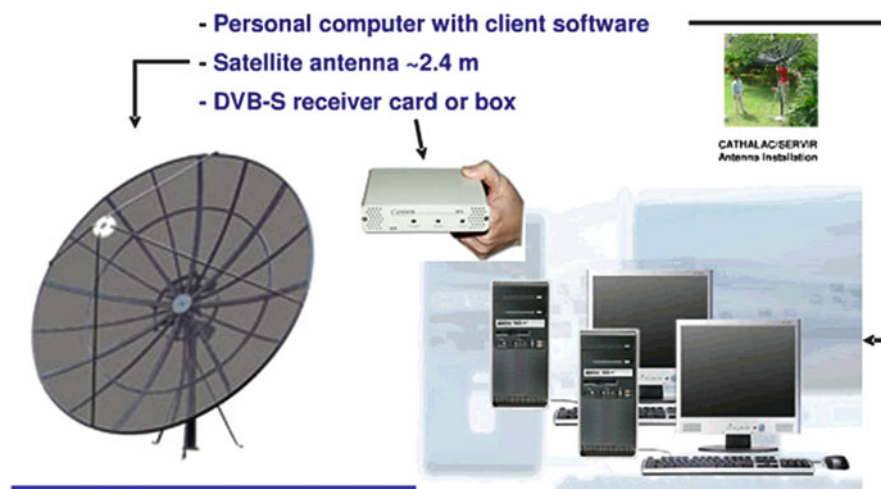
Fig. 7.8 A GEONETCAST ground station configuration (Image courtesy of NOAA)
