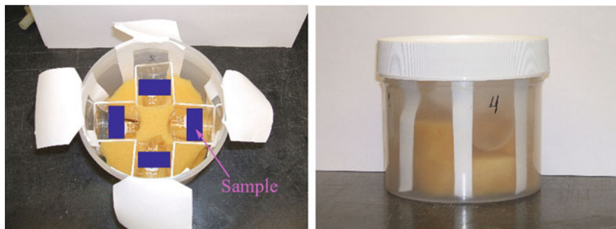
Fig. 3.3 Picture of an annealing chamber from the top ( left ) and side ( right )
