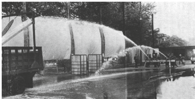
Fig. 6.1 This picture shows two water jets from identical fire hoses. Both hoses were aligned at the same angle and, for pure water, produced jets of equal reach. Then, a diluted solution with 30 ppm of high molecular weight poly(ethylene oxide) was used for the left hose. As a result, the jet exited at a higher speed, was more coherent, and had a significantly enhanced reach. (Reprinted from Bailey and Koleske 1976, Chap. 4, p. 81.)
