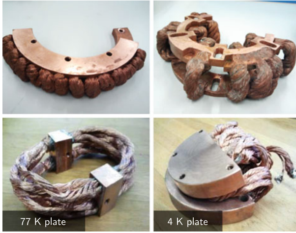
Fig. 7.5 The standard thermal anchoring of the PTR ( upper column ) was very stiff and also too short after the installation of the PTR head bellows ring. The self-made replacement of the thermal anchoring is shown below . By using longer and more flexible copper braids, the vibration transfer could be significantly reduced
