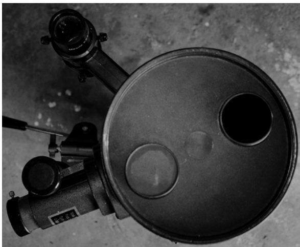
Fig. 8.9 A telescope lens cap with a hole in it to make solar viewing safer. You MUST still cover this hole with a solar viewing filter (Image by the author)
