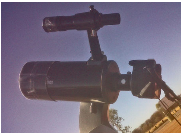
Fig. 8.7 The arrangement used to photograph Fig. 8.6, with a DSLR in prime focus (Image by the author)
