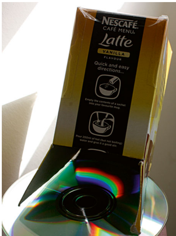
Fig. 8.42 A spectrograph like that shown in Fig. 8.41. In practice it proved to be easier to observe the spectrum of the Sun from indoors, in a room where the blinds had been mostly pulled down over the window. If this photograph is in color, the spectral lines are quite invisible. If the color is removed, two lines can be seen. Better results were obtained with a blank CD than with a blank DVD (Image by the author)
