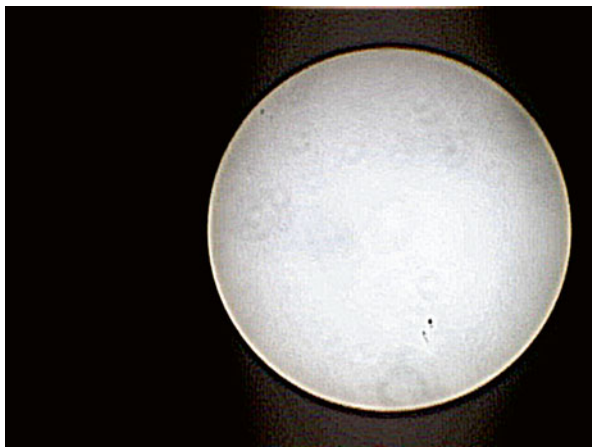
Fig. 8.5 The Sun, May 26, 2012, 07:44 UT. This image was taken with a webcam in afocal projection behind the eyepiece and a 102 mm (4 in.) f/10 Maksutov telescope on a computer-controlled alt-az mount, using a solar white light filter (Image by the author)
