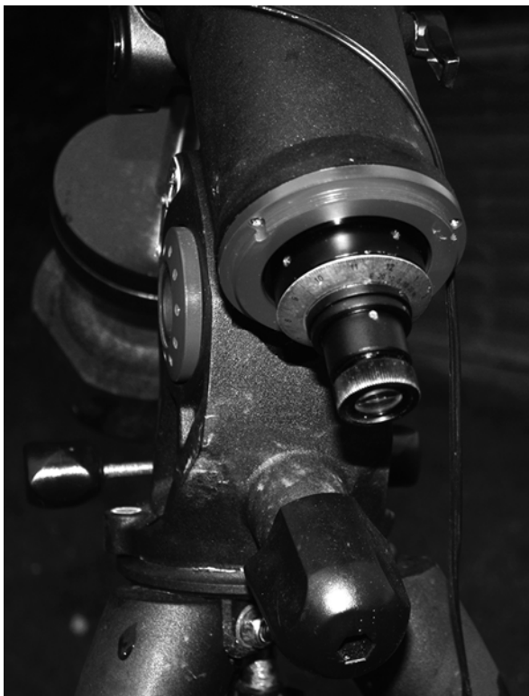
Fig. 2.9 A polar finder scope may be inserted along the right ascension axis of an equatorial mount (Image by the author)
