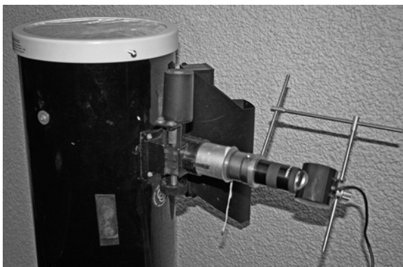
Fig. 8.3 Telescope with film in place and webcam in afocal projection, behind an eyepiece (Image by the author)
