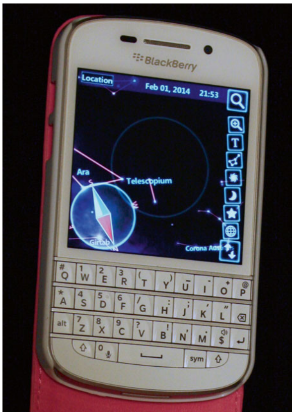
Fig. 10.1 An example of a smart phone (the BlackBerry Q10). The external appearance of such devices is usually very similar, except that most smart phones are touch-screen only. The App being shown in this case is 'Star Tracker' (Image by the author)
