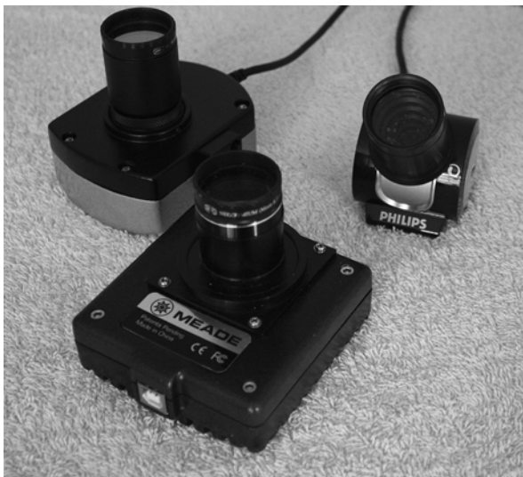
Fig. 4.1 The author's collection of Solar System imaging cameras. Front: A monochrome Meade DSI II. This was designed as a deep sky imager, but it works just fine for Solar System objects. It has a chip size of 752 \times 582 pixels, giving it a slightly wider angle of view than the 640 \times 480 chip on the color Philips SPC900NC camera ( right ). The lens has been removed from this camera. It has been replaced with a purpose-built 1.25" adaptor. To the rear left is a more modern monochrome Opticstar PL-131 M. It has a much larger 1,280 \times 1,024 chip. Because it is monochrome it has higher resolution than a color camera (see Fig. 8.46). It also has a much higher frame rate than the 5 fps of which the Philips is capable. This is good for capturing the rotation of Jupiter. The large chip makes it a lot easier to keep targets on the chip, at the cost of creating larger avi files (Image by the author)
