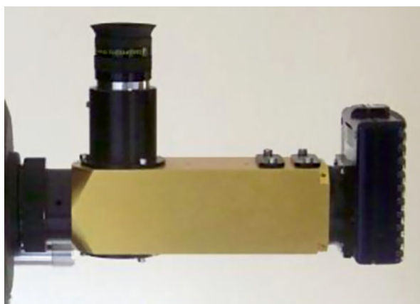
Fig. 8.47 The Elliott Instruments CCDSPEC spectrometer attached to the back of a catadioptric telescope with a Meade DSI II camera attached (Image from Elliott Instruments, Ltd., used with permission)
