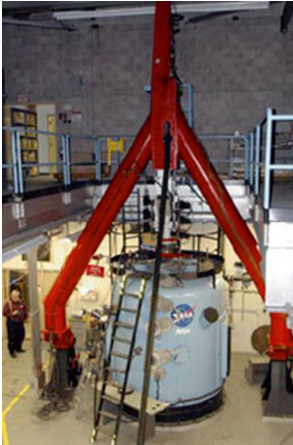
Fig. 6.32 The NASA Ames Vertical Gun Range for studying crater formation in laboratory conditions (Image courtesy of NASA)
