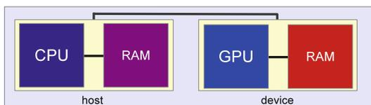
**Fig. 36** Hybrid compute node. An accelerator device (a GPU, or an Intel Xeon Phi card) is connected to an ordinary compute node through a fast bus system. Usually, host CPU and computing device each have their own RAM
