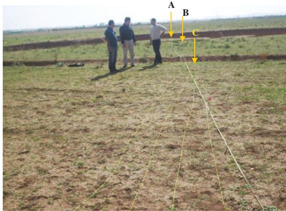
The relatively high resistive zone on the left edge of the image (below station position 22 m) could be the response of a further not deep cavity which is probably likely filled with clay. There are, however, no surface features indicative of the existence of a subsurface cavity.
