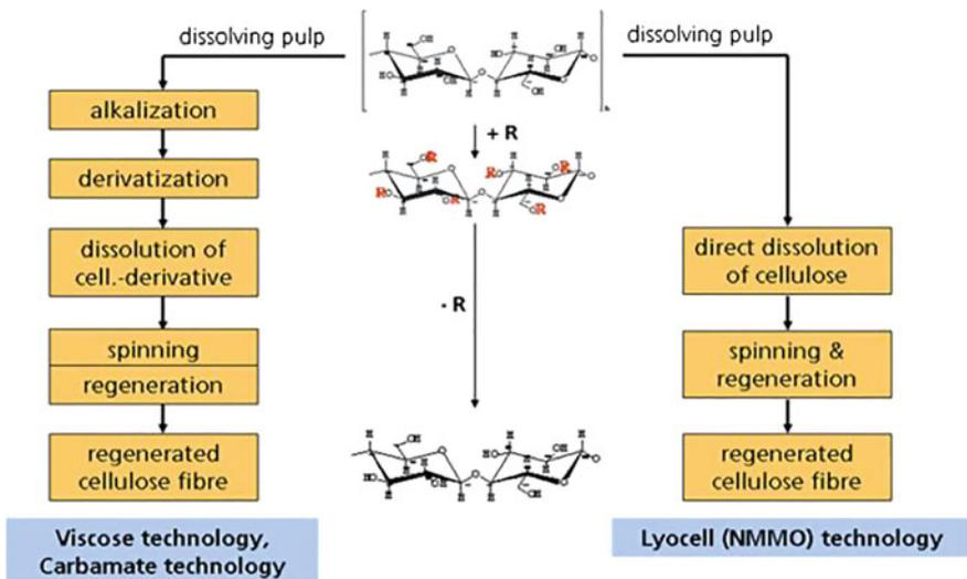
**Fig. 1.7** Processes for making cellulose regenerated cellulose fiber technologies (Fink et al. 2014)
