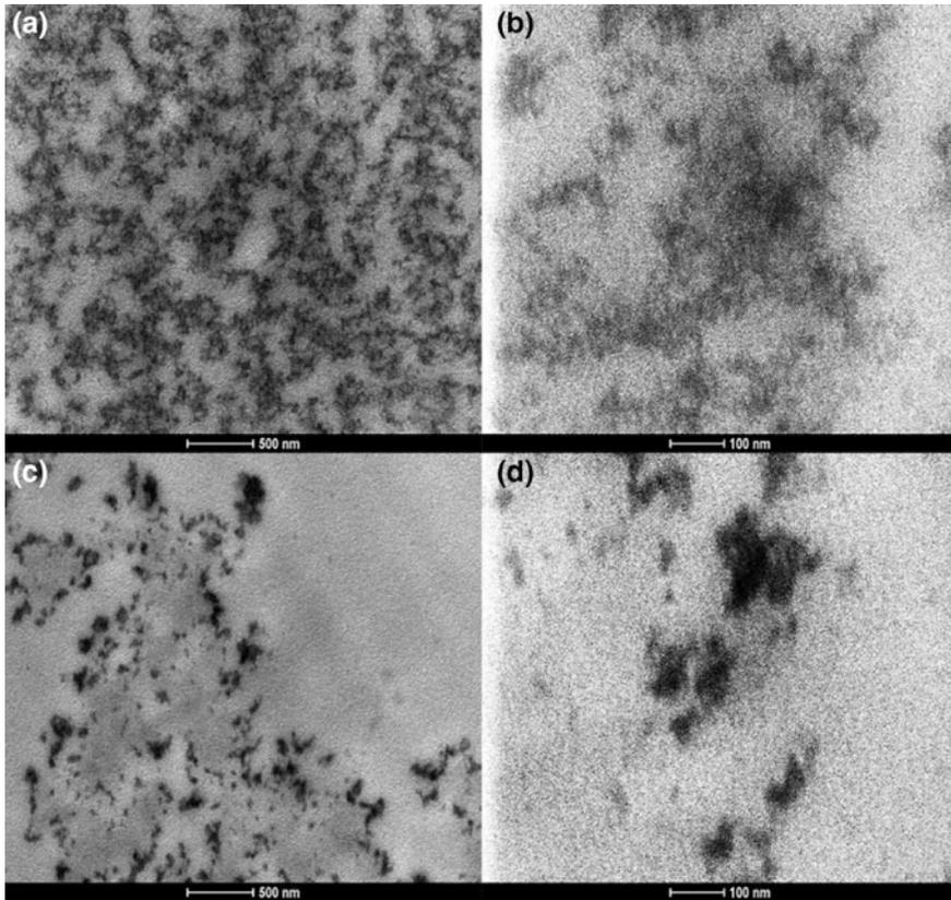
**Fig. 5.11** TEM images of **a, b** WPI fiber and **c, d** cellulose/WPI blend fibers. Adapted with permission from (Tomczyńska-Mleko et al. 2015b). Copyright 2016, Elsevier
