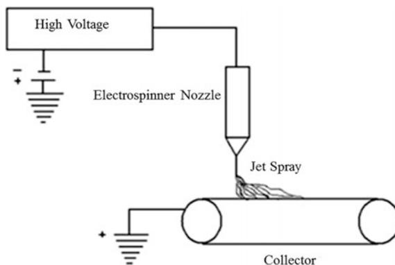
Fig. 1.6 Electrospinning process flowchart (Textile Engineer, Blogspot 2016)
