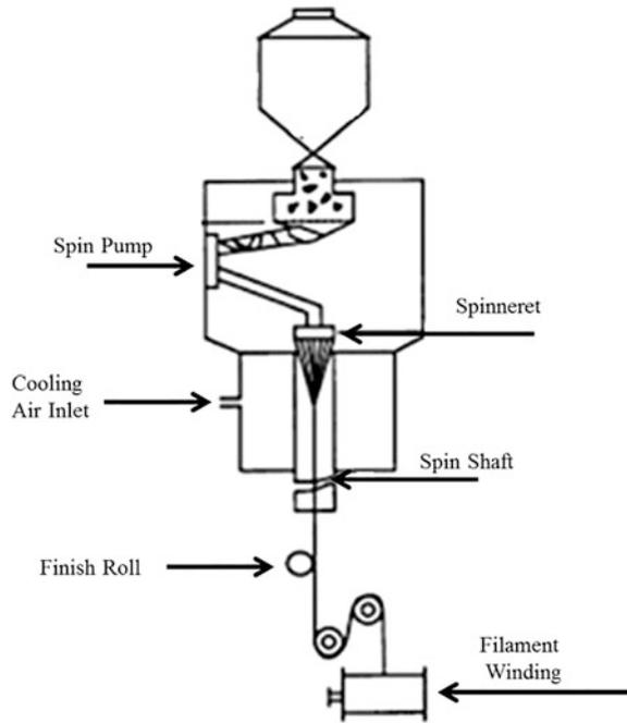
**Fig. 1.4** Dry spinning process flowchart (Textile Engineer, Blogspot 2016)
