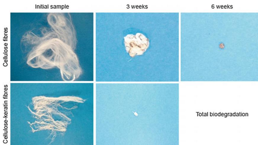
**Fig. 5.20** Biodegradation of cellulose and cellulose/keratin composite fibers by composting. Adapted with permission from (Wrzesniewska-Tosik et al. 2007). Copyright 2016, IBWCh
