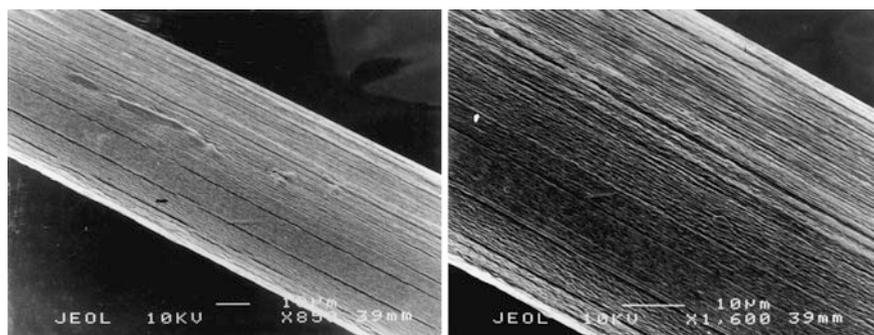
**Fig. 5.8** SEM images of the cellulose/protein (53% silk fibroin) fiber (55  $\mu\text{m}$  in diameter). Adapted with permission from (Hirano et al. 2002). Copyright 2016, Elsevier
