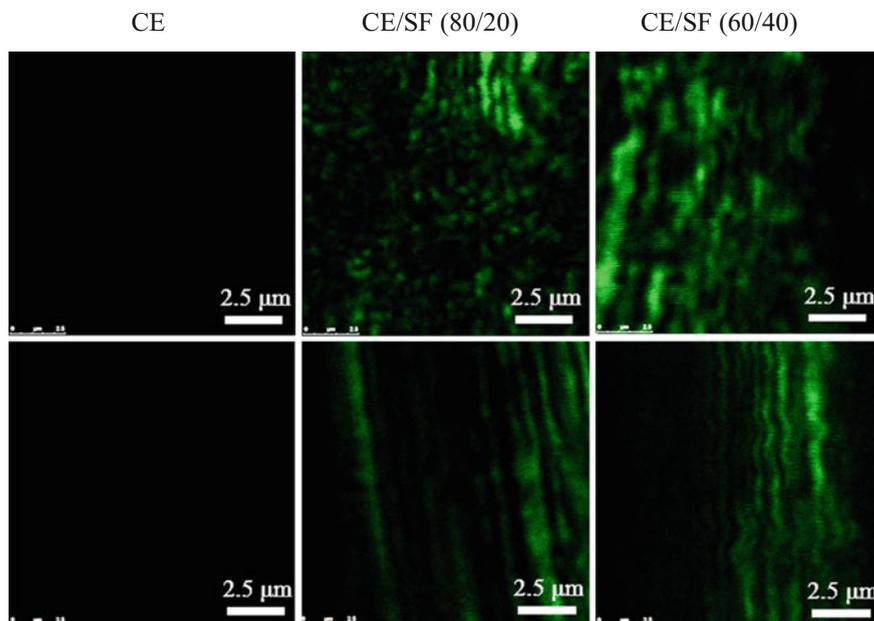
**Fig. 5.23** LSCM micrograph of cellulose and CE/SF fibers along the fiber axes (top row at  $D_r = 3.3$ , bottom row at  $D_r = 4.3$ ). Adapted with permission from (Yao et al. 2015). Copyright 2016, Springer
