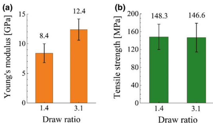
**Fig. 2.4** **a** Young's modulus and **b** tensile strength comparison of chitin Fiber set B (draw ratio = 1.4) and Fiber set C (draw ratio = 3.1) spun at a constant extrusion velocity  $V_1 = 0.09$  m/s
