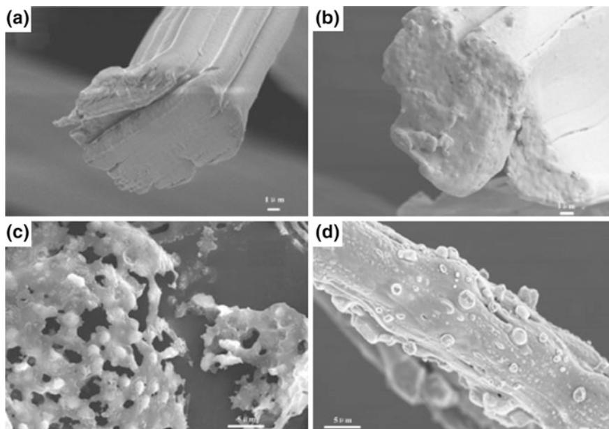
**Fig. 5.10** SEM images of the cross sections of **a** viscose fiber and **b** cyclotriphosphazene/viscose fiber, **c** residues of **a** and **d** **b** after burning behavior test. Adapted with permission from (Zhou et al. 2015). Copyright 2016, Springer
