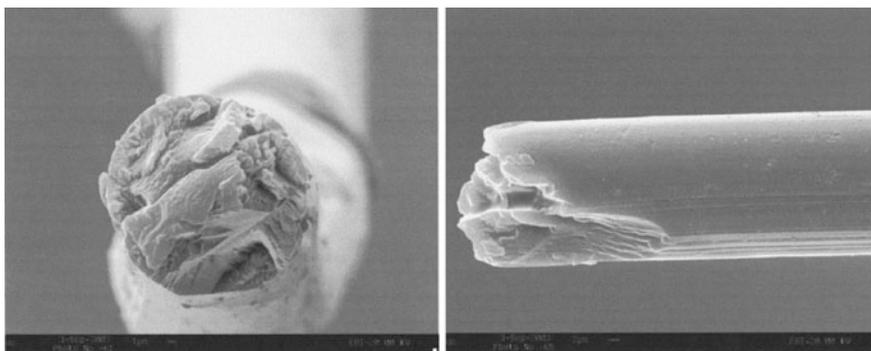
**Fig. 5.14** SEM images of the CE/SF blend fiber ( $C_p = 7$  wt% and  $D_r = 2$ ). Adapted with permission from (Marsano et al. 2007). Copyright 2016, John Wiley and Sons
