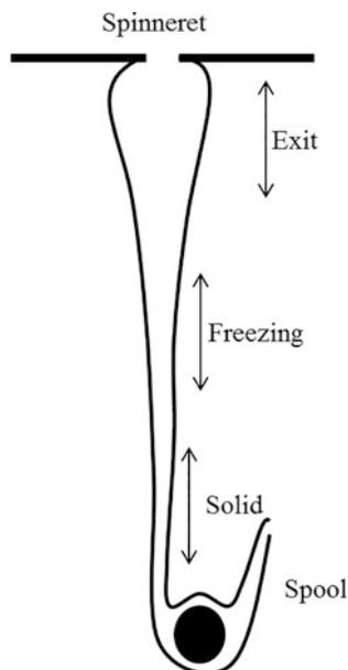
through its cross section is nearly uniform and normal stress connected with shear flow in the spinneret is practically relaxed. The elongation region extends over some scores of centimeters of the spinning path, molecular orientation develops here and solidification processes take place, thereby making this region the most important step in the technology of the spinning process (Ziabicki 1988).
