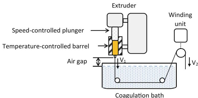
**Fig. 2.1** Schematic of dry-jet wet fiber spinning process for chitin with a constant extrusion velocity  $V_1 = 0.09$  m/s and various winding velocities ( $V_2$ )
