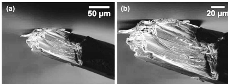
**Fig. 2.5** a, b SEM images of fracturing cross-section of Fiber set B (draw ratio = 3.1) spun at a constant extrusion velocity  $V_1 = 0.09$  m/s
