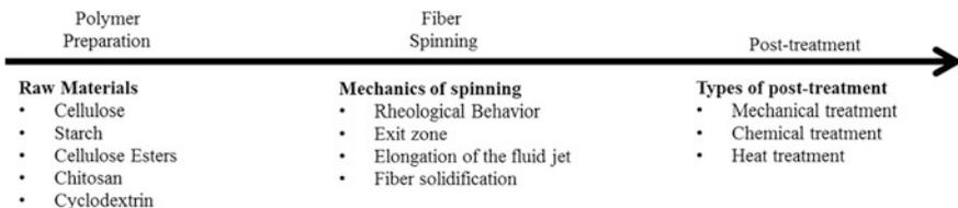
**Fig. 1.1** Steps in the manufacture of fibers
