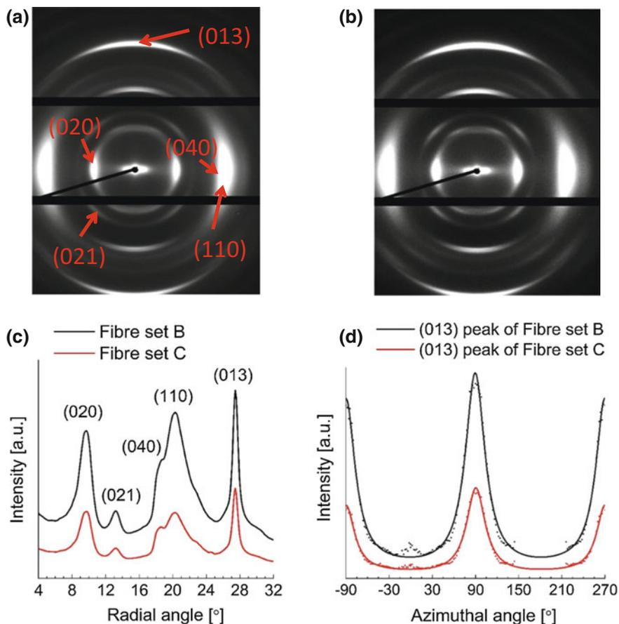
**Fig. 2.6** WAXD patterns of single chitin filament for **a** Fiber set B (draw ratio = 1.4), **b** Fiber set C (draw ratio = 3.1), **c** integrated radial scans of Fiber set B (draw ratio = 1.4) and Fiber set C (draw ratio = 3.1) spun at a constant extrusion velocity  $V_1 = 0.09$  m/s, as well as **(D)** azimuthal scans of the chitin (013) diffraction peaks of Fiber set B (draw ratio = 1.4) and Fiber set C (draw ratio = 3.1) spun at a constant extrusion velocity  $V_1 = 0.09$  m/s
