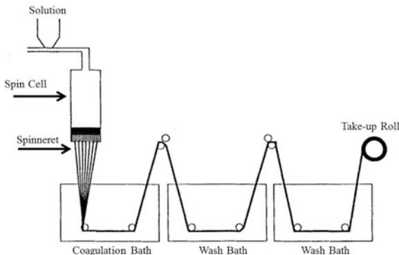
Fig. 1.5 Wet spinning process flowchart (Textile Engineer, Blogspot 2016)
