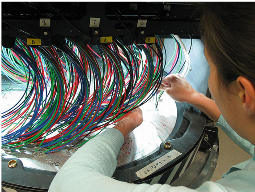
Fig. 12.2 A technician connects the fibers between the spectrograph and a metal plate that will be mounted at the focus of the Sloan Telescope. Image credit: New Mexico State University
