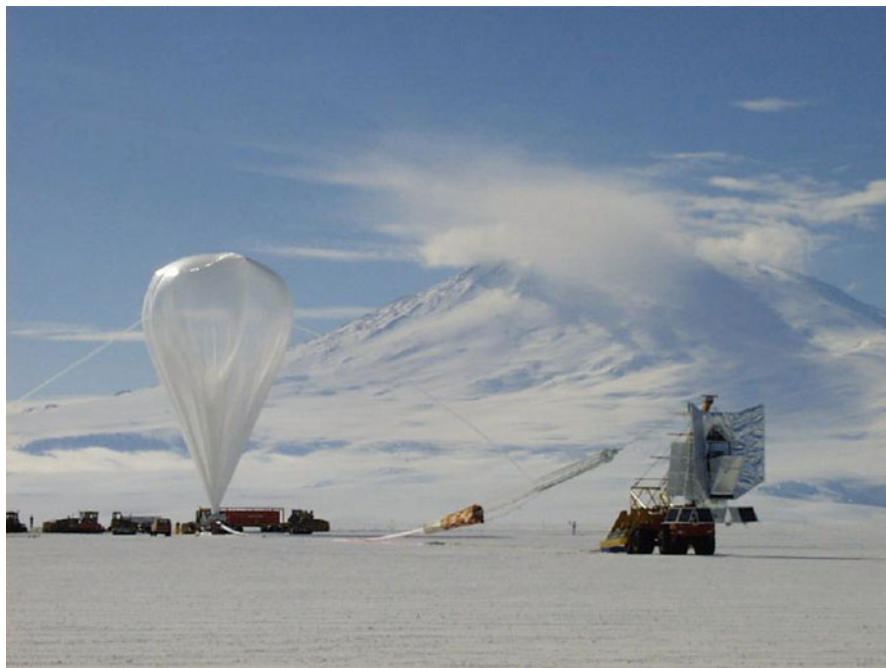
Fig. 7.6 The Boomerang telescope being launched for its 10-day trip around the South Pole. Image credit: Wikipedia
