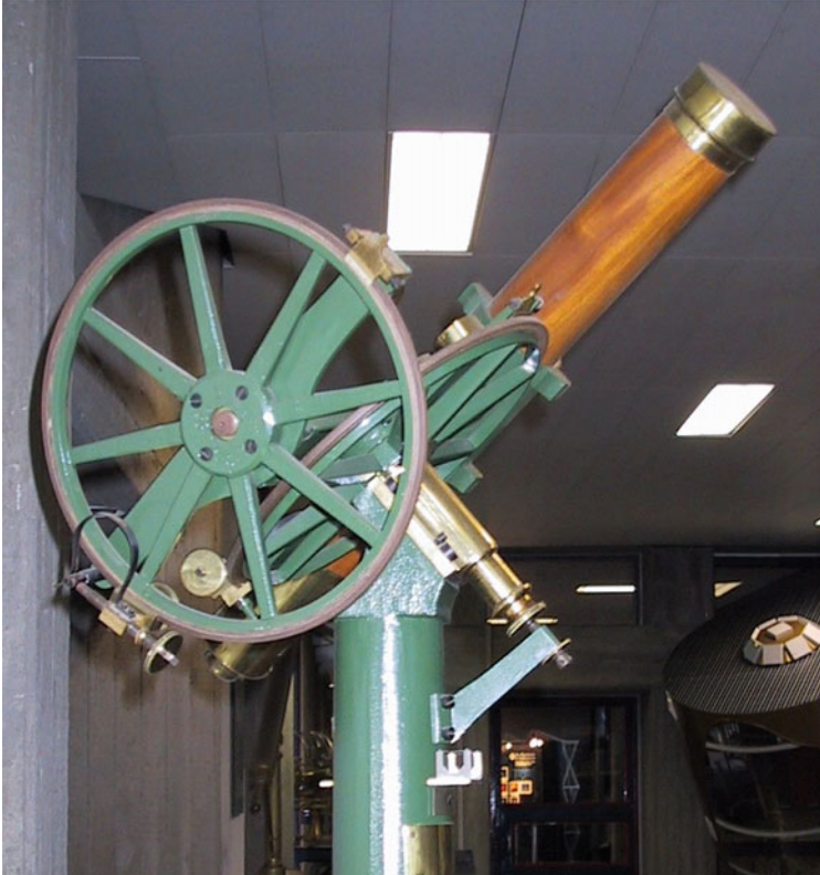
Fig. 3.9 Argelander's telescope at the Bonn Observatory. The large wheels carried the scales with which a star's position could be accurately measured. Image credit: Michael Geffert
