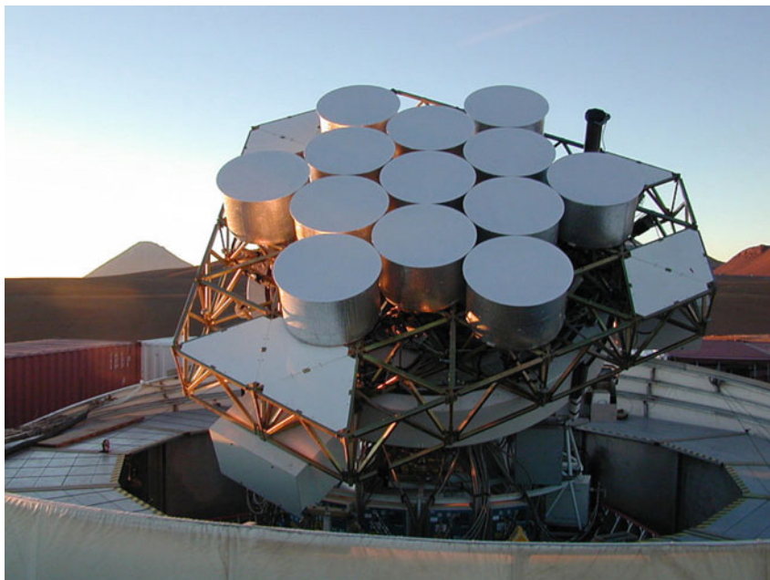
Fig. 7.5 The Cosmic Background Imager at the Chajnantor Observatory at an altitude of 5080 m in the Chilean Andes. Image credit: Caltech
