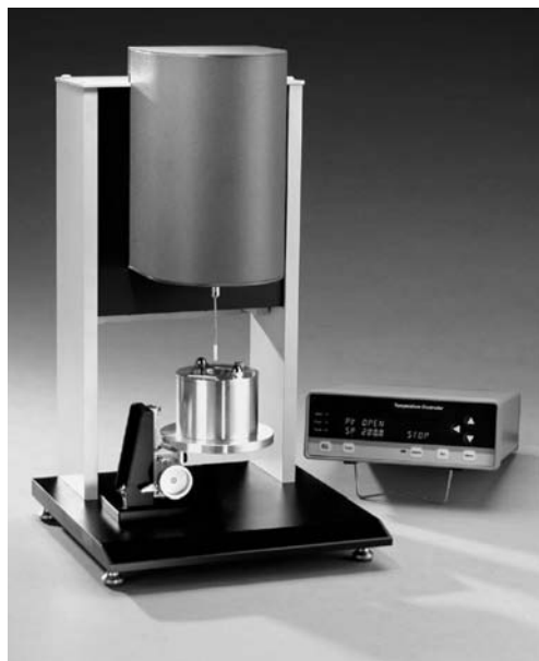
FIG. 4.9 T2SR rheometer with temperature controller and high-temperature heating cell. (Courtesy of Fluid Dynamics, Inc.)
