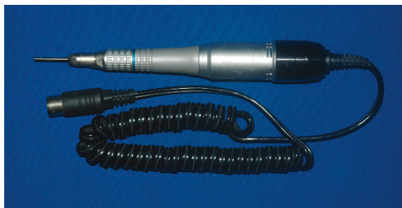
Fig. 11.2 Light duty electric hand engine used for small lesions. Dental Micro motor can be used
