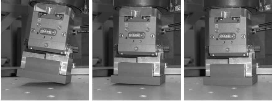
Fig. 9. Block placement by the HEXA-robot
