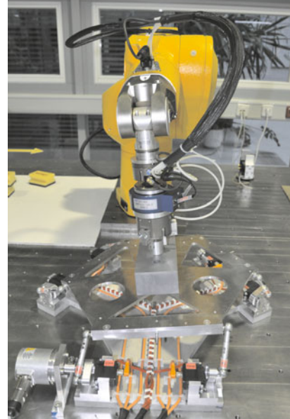
Fig. 5. Experimental setup with stiffness actuator installed in the environment.
