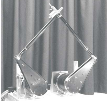
Fig. 4a. Elastic planar parallel robot FIVE-BAR
