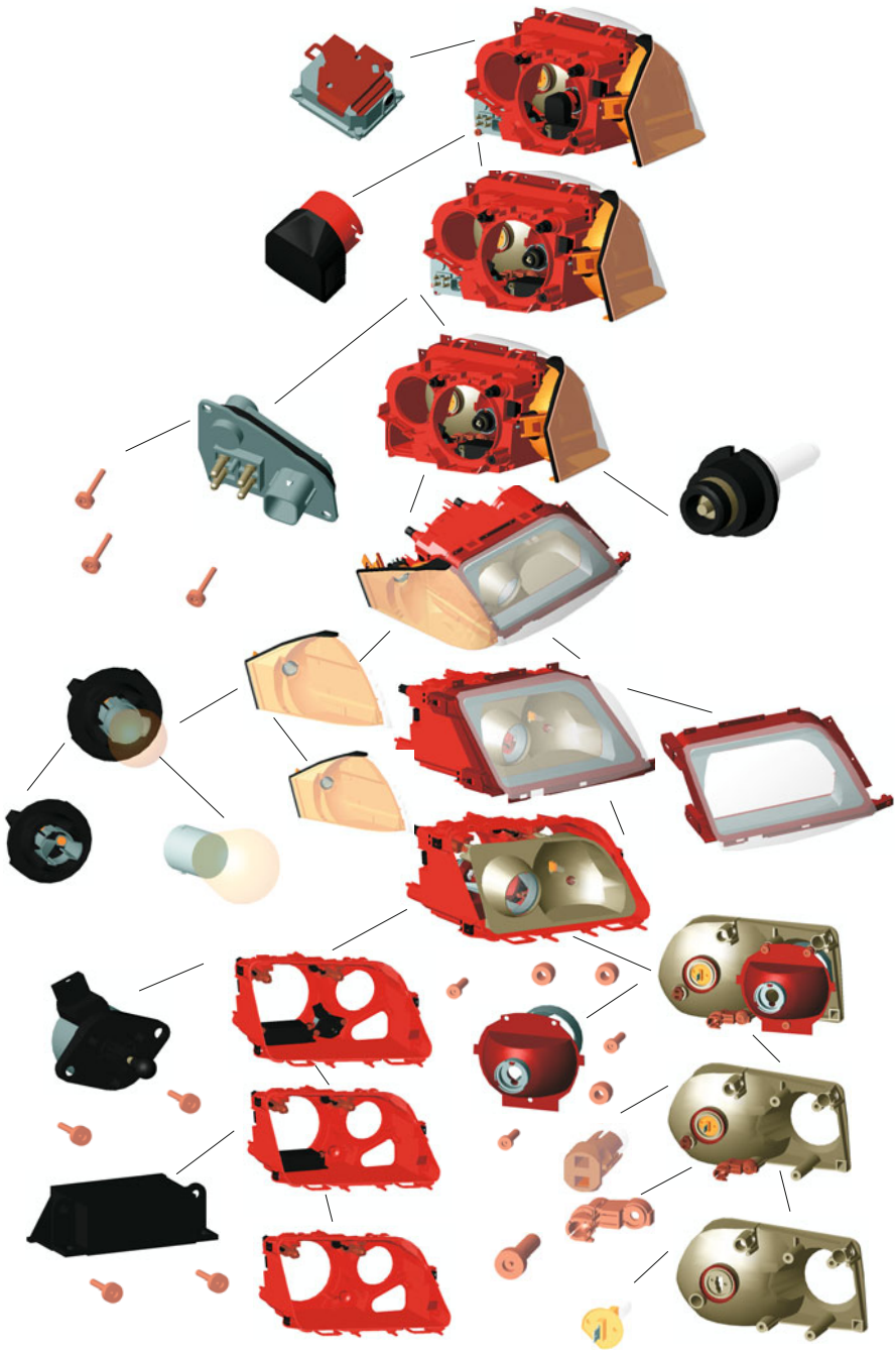
Fig. 8. A computed assembly plan for an automotive headlight assembly.
