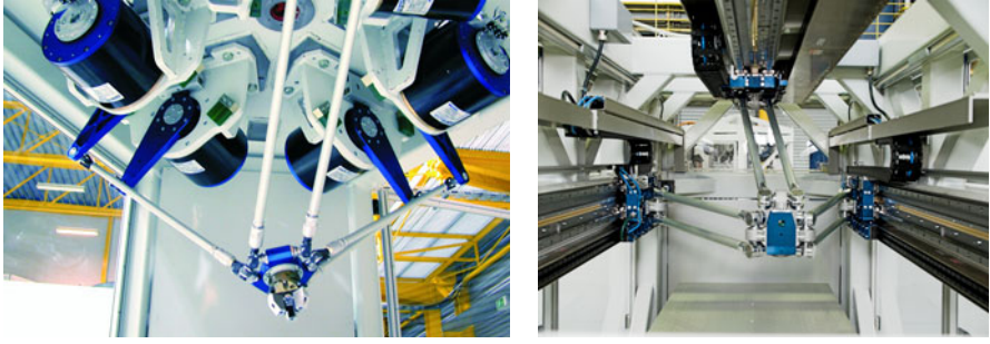
Fig. 1. Example parallel structures: a HEXA manipulator. b TRIGLIDE manipulator.
