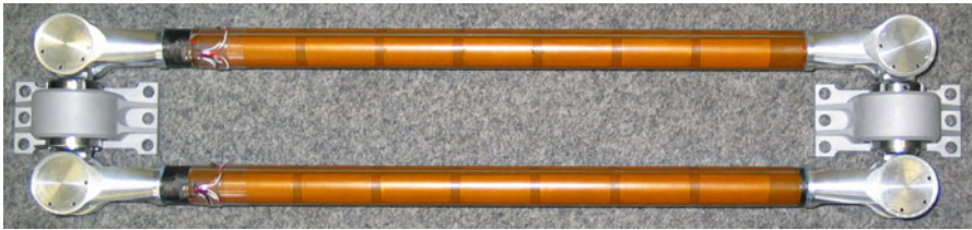
Fig. 11. Kinematic leg of the TRIGLIDE containing self-developed joints and adaptive links.
