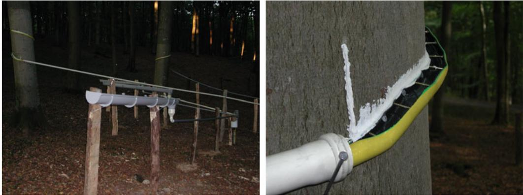
**Fig. 4.6** Throughfall (*left*) and stemflow (*right*) collection systems in the Huewelerbach experimental plot
