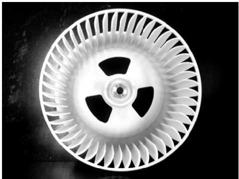
Fig. 8. The test case prototype printed with a RP machine
