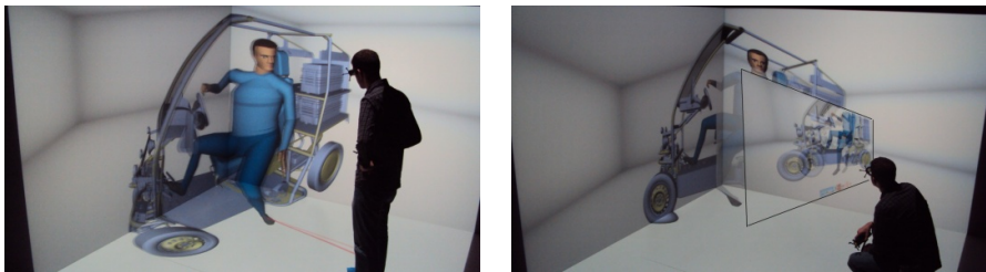
Fig. 3. The ergonomist visualizes the vehicle with the virtual human (left). The ergonomist takes a snapshot to his viewpoint (right).
