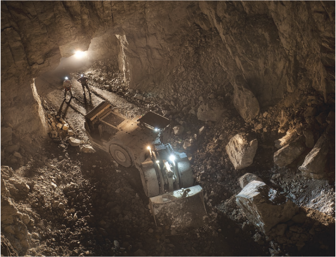
■ Fig. 5.52 LHD used with remote control (Image courtesy of Matsa, a Mubadala and Trafigura Company)
