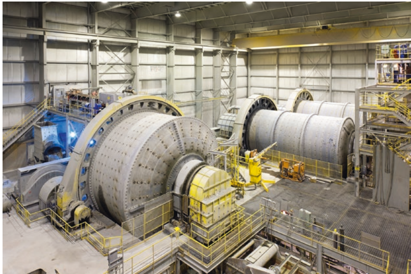
■ Fig. 1.16 Particle size reduction using mills (Image courtesy of North American Palladium Ltd.)
