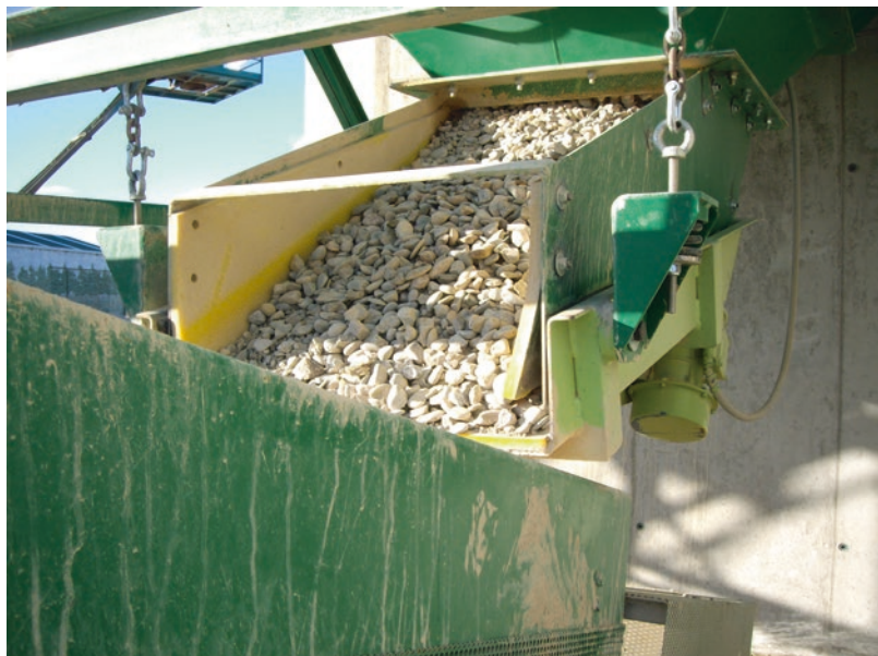
■ Fig. 6.10 Vibrating feeder in an aggregate quarry (Image courtesy of Marcelino Martínez)
