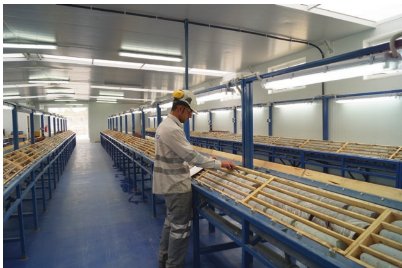
■ Fig. 3.59 Proper storage of core (Image courtesy of Matsa, a Mubadala & Trafigura Company)
