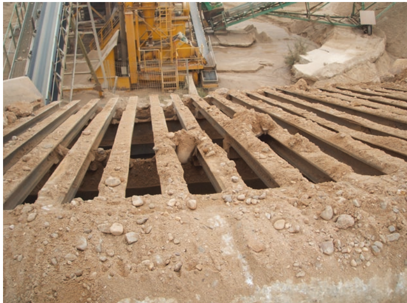
■ Fig. 6.31 Grizzly for rough screening
