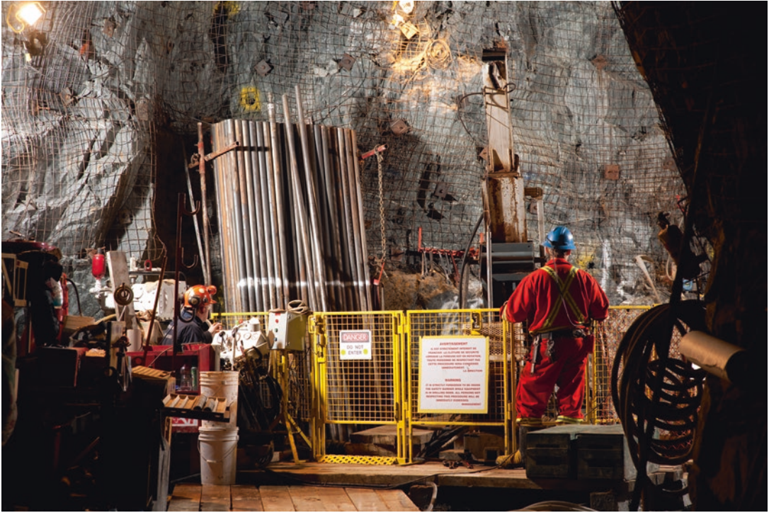
■ Fig. 3.60 Diamond drill underground exploration station (Canada) (Image courtesy of North American Palladium Ltd.)
