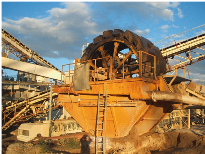
■ Fig. 6.85 Dewatering wheel (Image courtesy of CEMEX)
