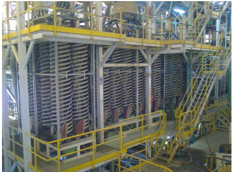
▣ Fig. 6.50 Multiple units of spiral concentrator (Image courtesy of Daytal Resources Sapin S.L.)
