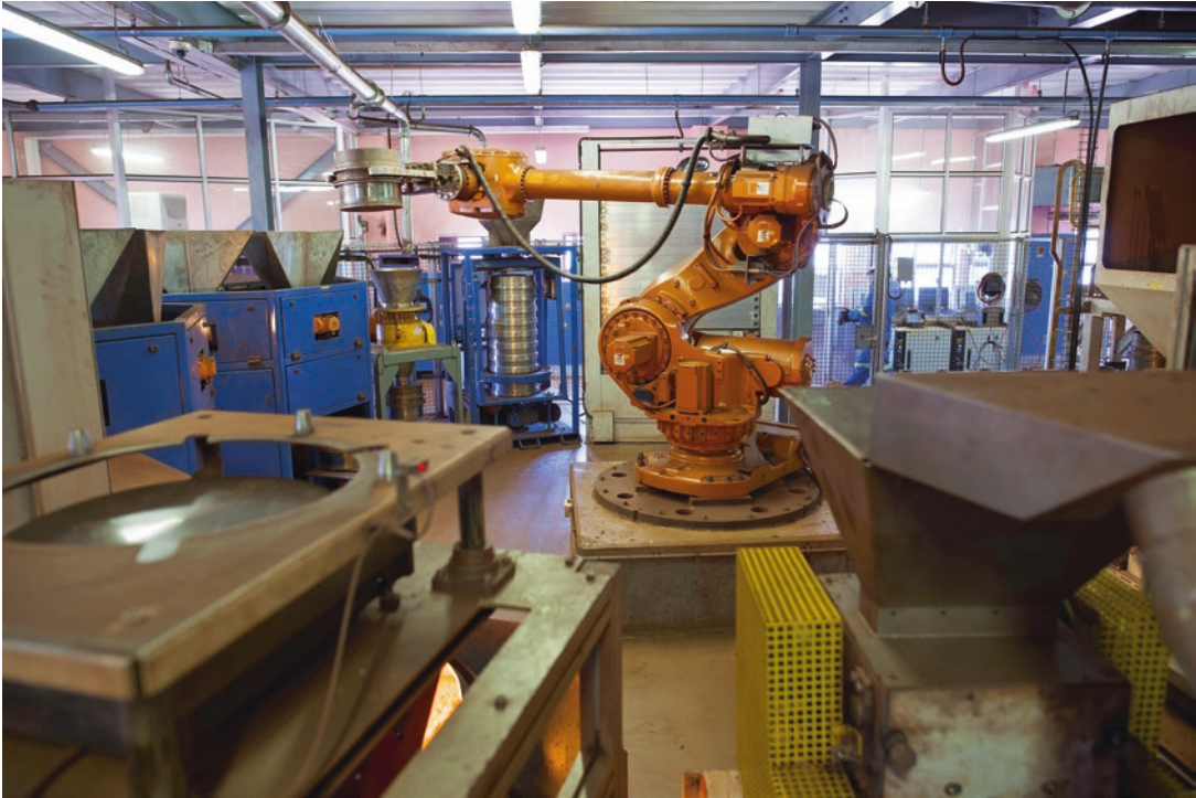
■ Fig. 4.1 Fully automated sample plant-taking samples; the process is completely hands off and uses robotics to perform the analysis (Image courtesy of Anglo American plc.)
