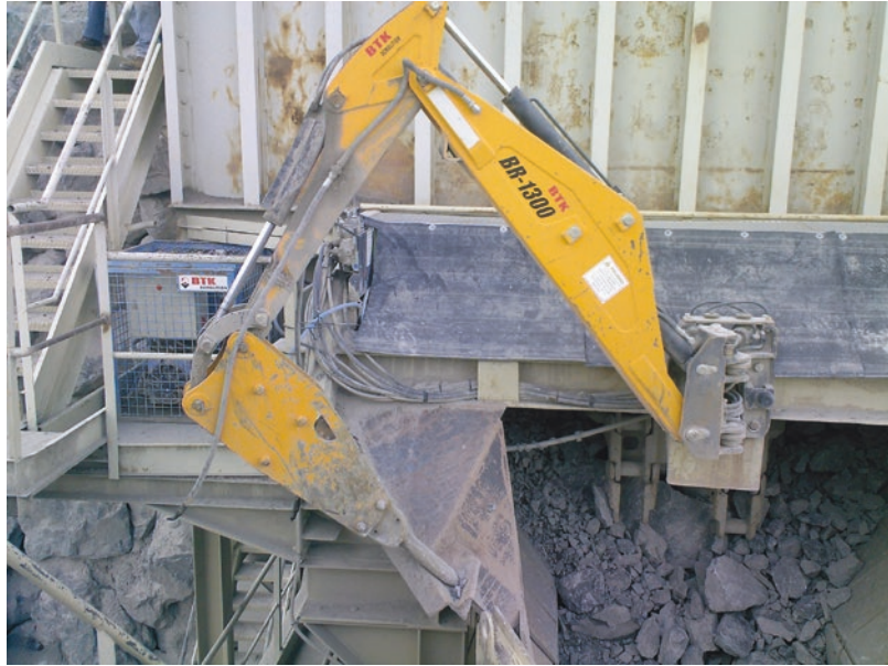
■ Fig. 6.16 Primary jaw crusher with a hammer on the surface
