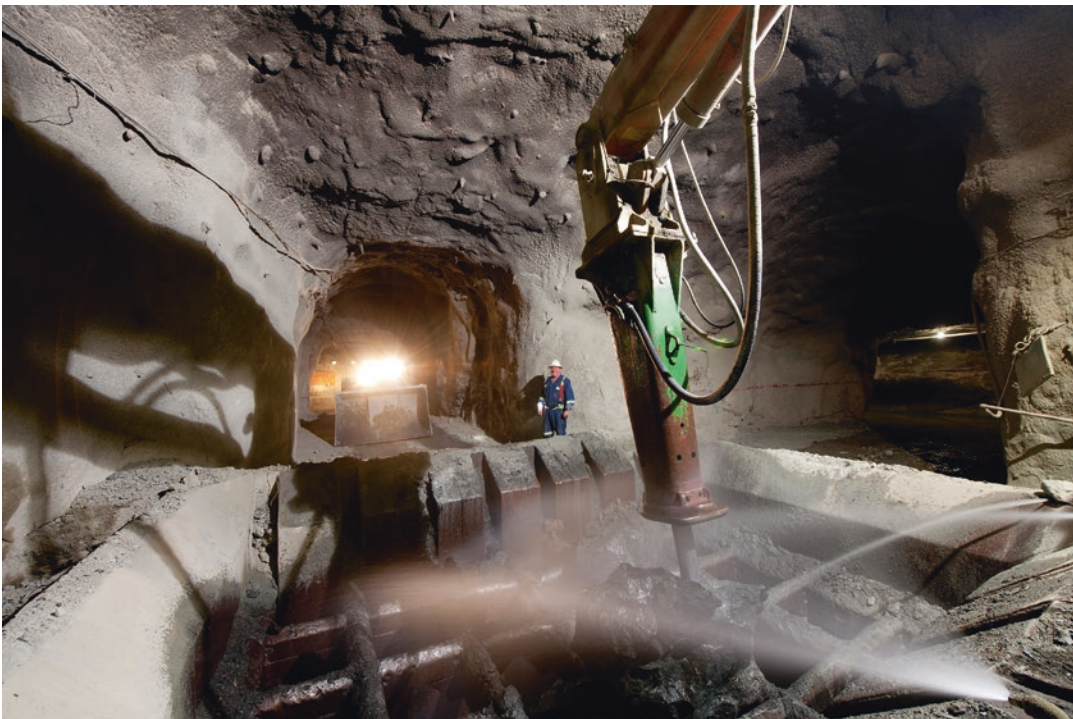
■ Fig. 6.12 Primary crushing in an underground mine (South Africa) (Image courtesy of Petra Diamonds)
