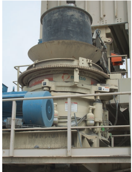
■ Fig. 6.18 Cone crusher in an aggregates processing plant (Image courtesy of Benito Arnó e Hijos S.A.U.)
