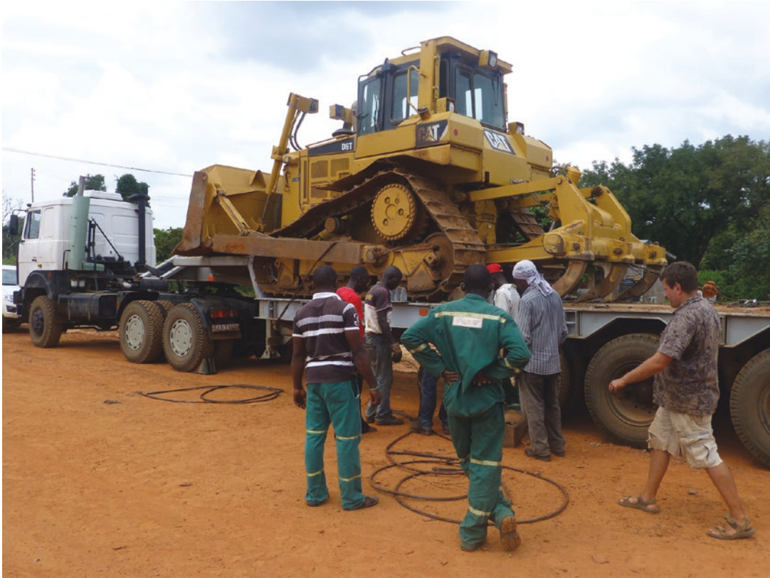
■ Fig. 5.18 Special tow truck transport medium for mining equipment (Image courtesy of Eduardo Revuelta)
