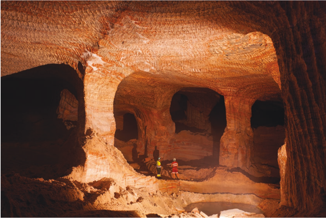
■ Fig. 5.58 Underground mining using unsupported method (Spain) (Image courtesy of Iberpotash)
