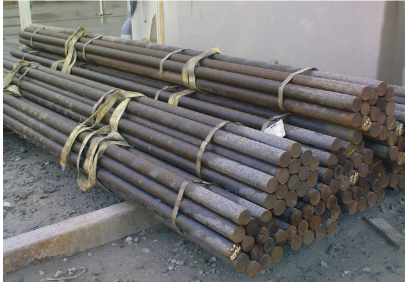
■ Fig. 6.23 Rods for a rod mill (Image courtesy of Daytal Resources Spain S.L.)
