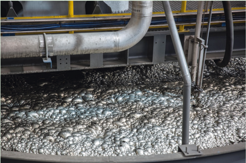
■ Fig. 6.64 Froth flotation of polymetallic ore (Image courtesy of Matsa, a Mubadala & Trafigura Company)
