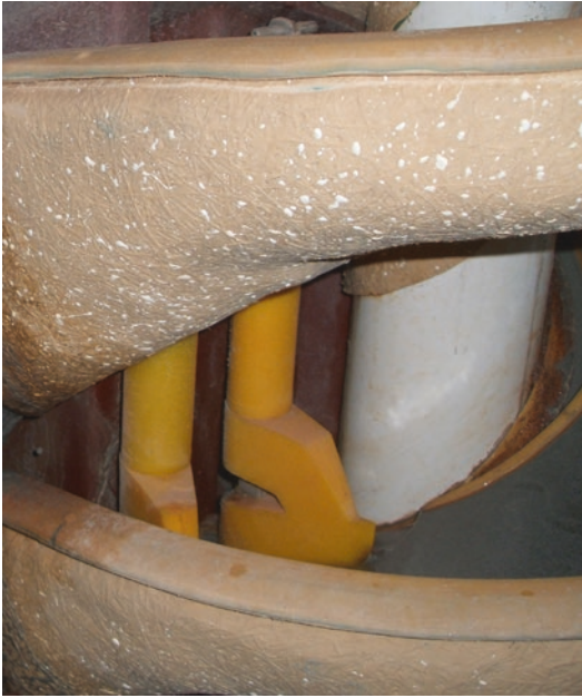
▣ Fig. 6.49 Three splitters at the end of the spiral (Image courtesy of Daytal Resources Spain S.L.)
