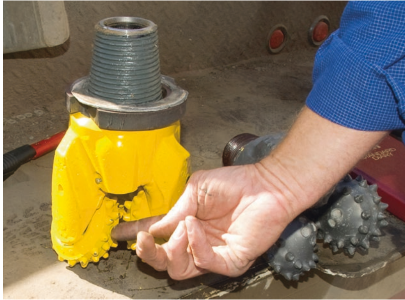
■ Fig. 5.78 Tricone bit (Image courtesy of Atlas Copco)
