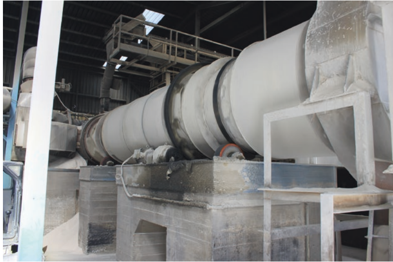
■ Fig. 6.89 Rotary kiln form thermal dewatering (Image courtesy of SAMCA)
