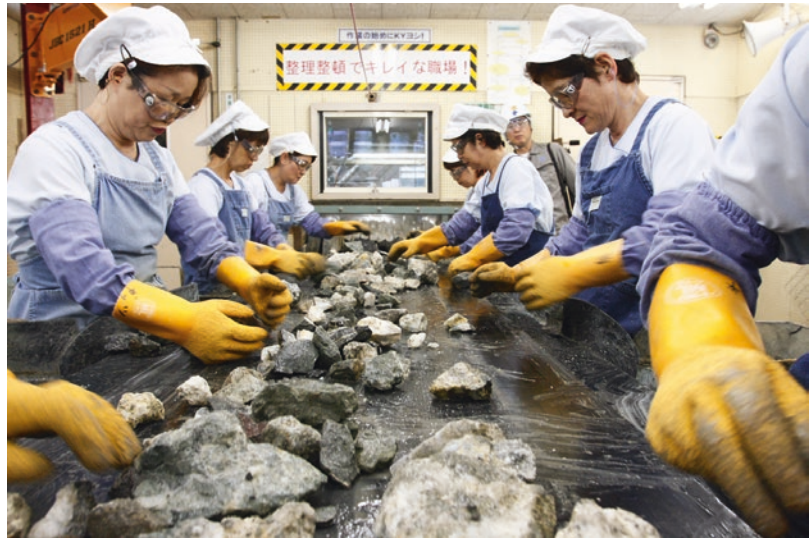
■ Fig. 6.5 Hand sorting at conveyor belt (Image courtesy of Sumitomo Metal Mining Co., Ltd.)
