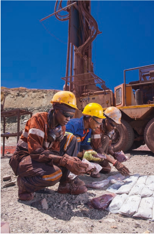
■ Fig. 3.48 Preparing samples after drilling (Image courtesy of Anglo American plc.)
