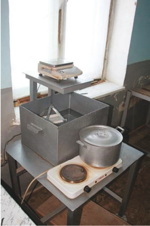
■ Fig. 4.29 Station for measuring dry bulk density (Image courtesy of Lydian International Ltd.)
