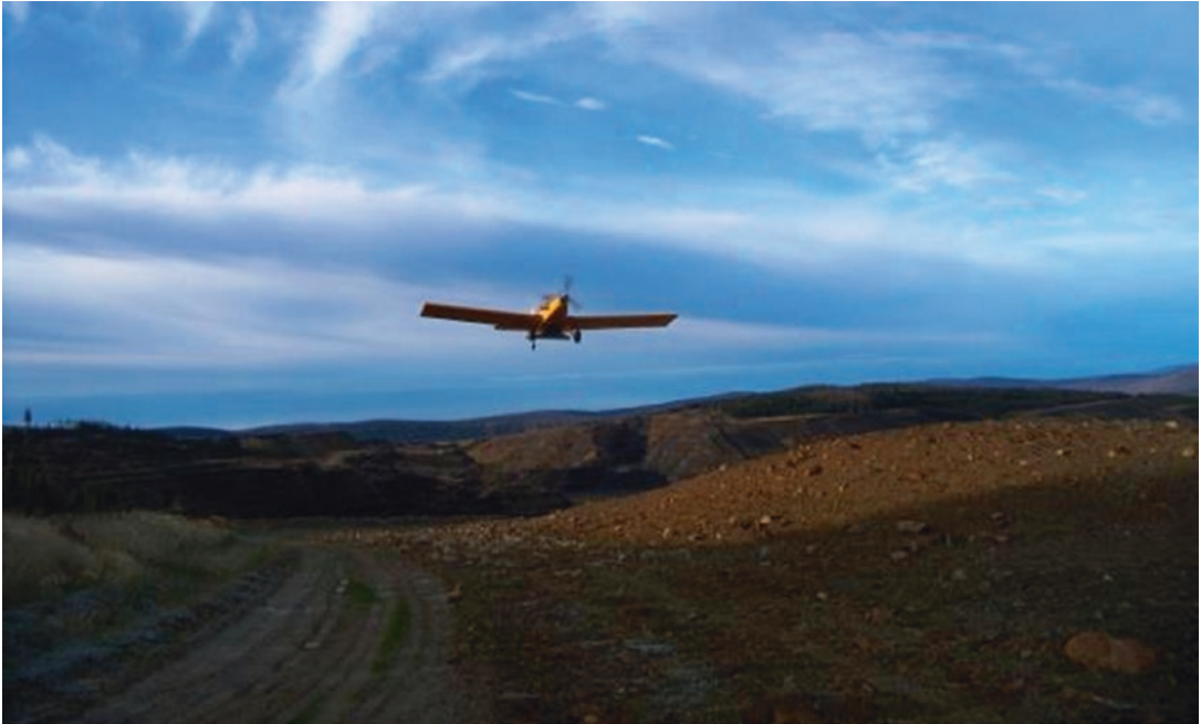
■ Fig. 7.43 Aerial seeding via fixed wing aircraft (Image courtesy of Kinross Gold Corporation)
