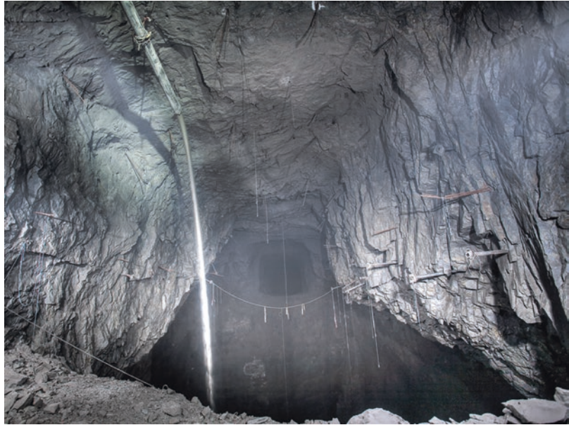
■ Fig. 6.95 Underground mine hydraulic backfilling (Spain) (Image courtesy of Matsa, a Mubadala & Trafigura Company)
