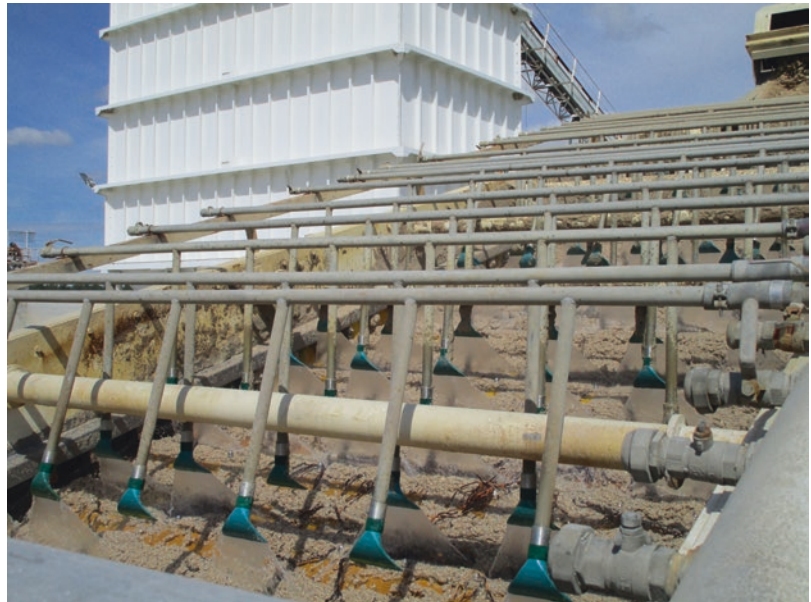
■ Fig. 6.33 Polyurethane nozzles placed cross-sectionally to the material flow (Image courtesy of SAMCA)
