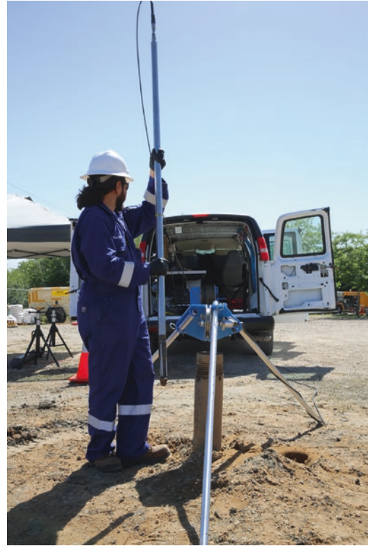
■ Fig. 3.28 Caliper geophysical borehole logging (Image courtesy of Robertson Geologging)
