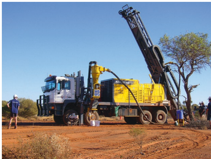
■ Fig. 3.51 Reverse circulation drilling machine (Image courtesy of Atlas Copco)
