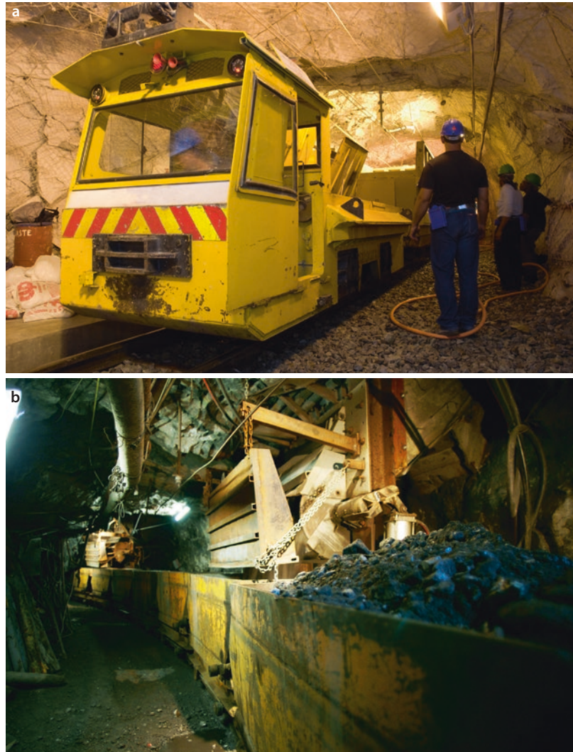
■ Fig. 5.73 Ore handling using trains (a Image courtesy of AngloGold Ashanti; b Image courtesy of Eldorado Gold Corporation)
