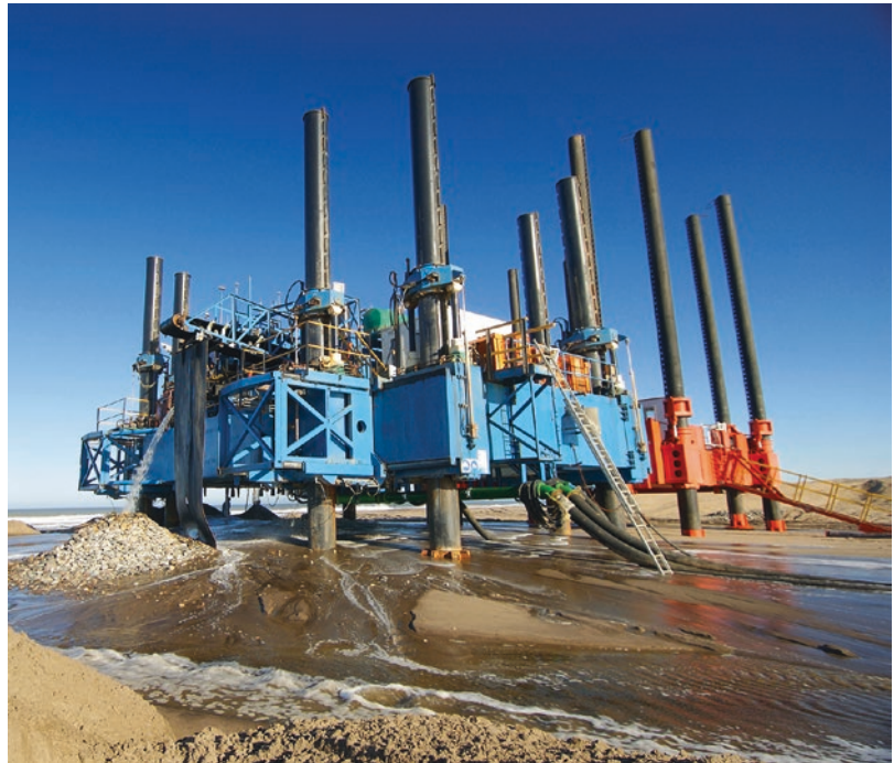
■ Fig. 5.37 Namdeb walking jack-up platform that includes a purpose-designed dredge pump to extract sand and gravel and pick out diamonds in Namibian coastline (Image courtesy of De Beers)
