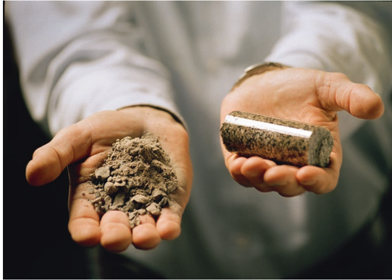
■ Fig. 3.50 Rock chips and core samples (Image courtesy of Atlas Copco)
