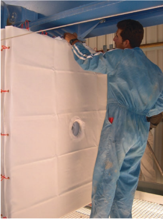
■ Fig. 6.7 Semipermeable membrane for filtering (Image courtesy of TEFSA)
