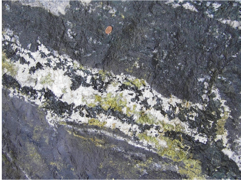
■ Fig. 2.53 Mineralization of magnetite and sulfides in Cala mine (Spain) (Image courtesy of César Casquet)
