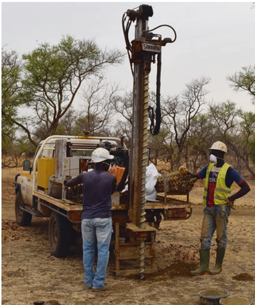
■ Fig. 3.61 Auger drilling at Burkina Faso (Image courtesy of SEMAFO Inc.)
