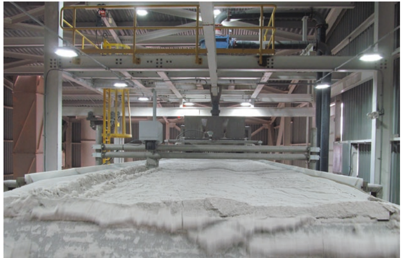
■ Fig. 6.88 Horizontal belt filter and discharge area (Image courtesy of Compositech Filters)
