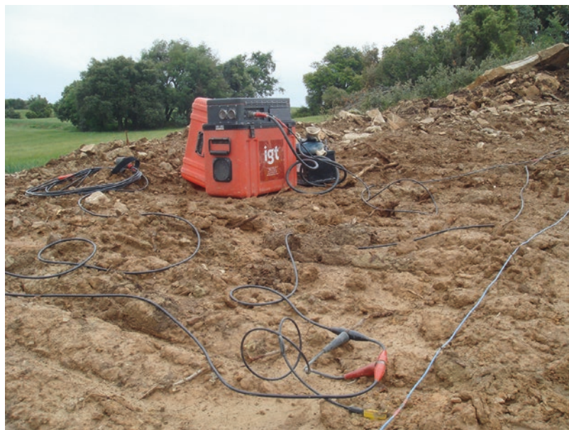
■ Fig. 3.26 Seismic refraction survey (Image courtesy of International Geophysical Technology)
