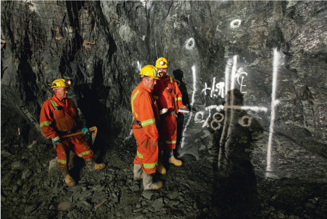
■ Fig. 4.26 Discriminating between ore and waste in underground mining (Image courtesy of North American Palladium Ltd.)
