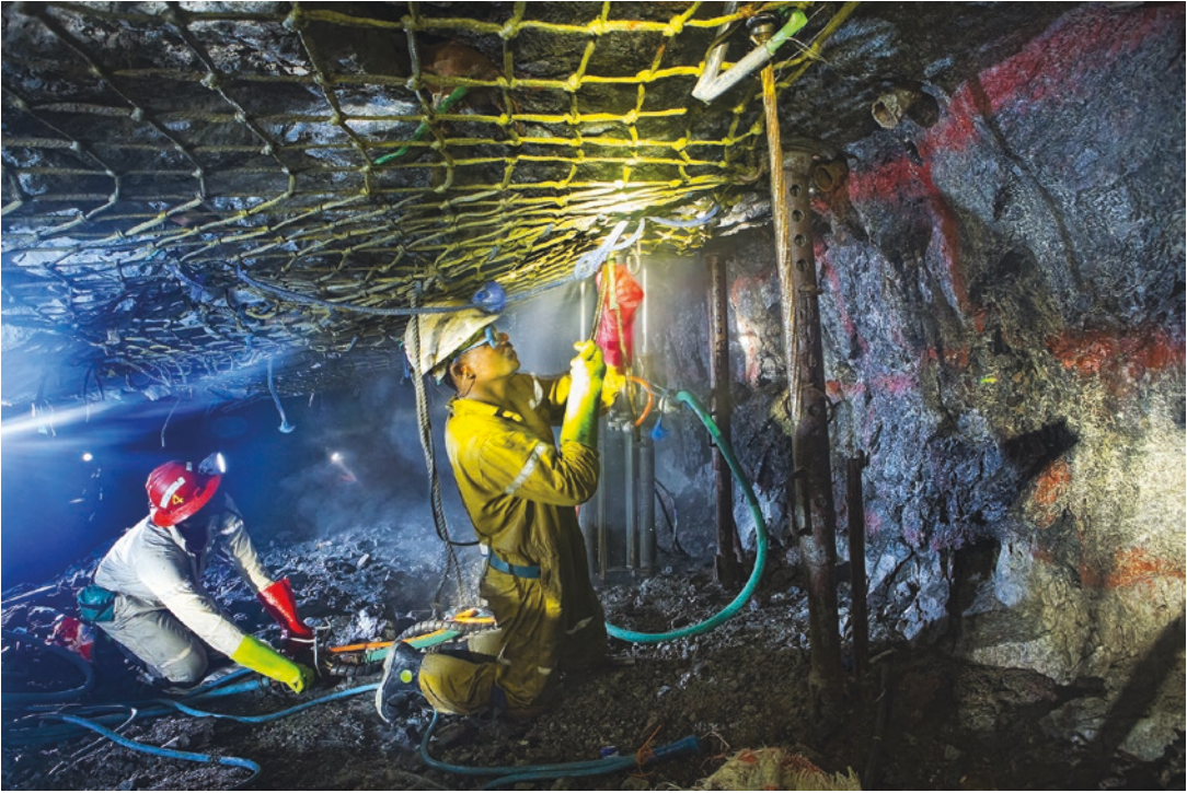
■ Fig. 5.55 Installing cable bolts at Dishaba Mine (South Africa) (Image courtesy of Anglo American plc)
