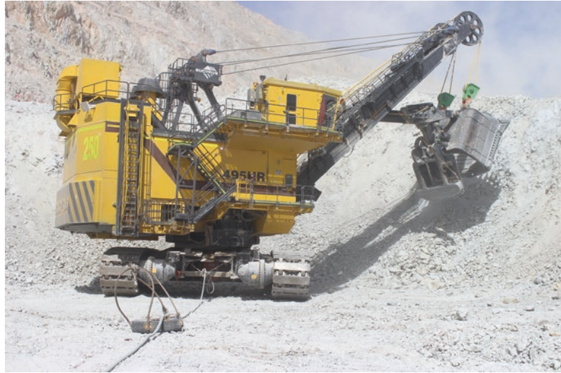
■ Fig. 5.15 Electrical cable shovel (Image courtesy of Codelco)
