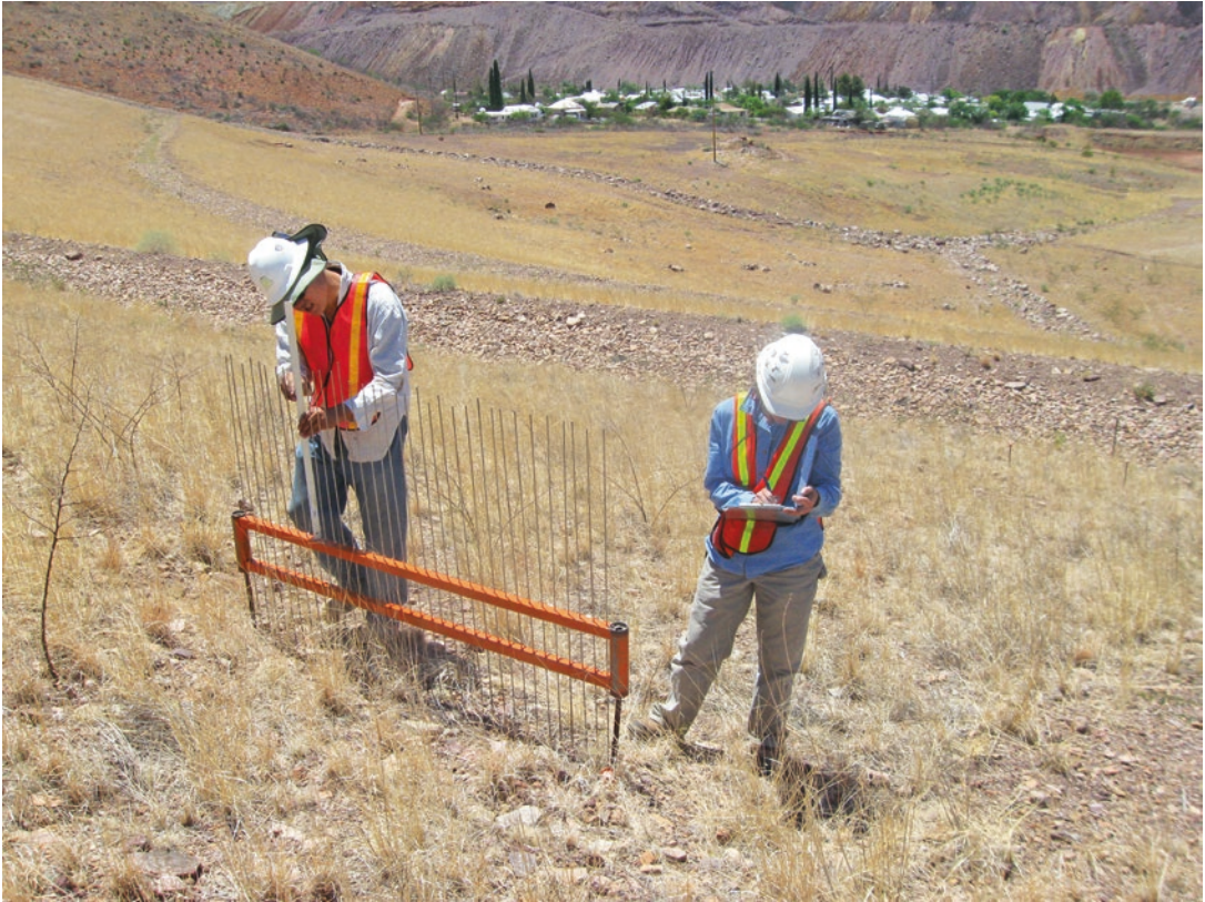
■ Fig. 7.11 Control of erosion using a mechanical erosionometer (Image courtesy of Freeport-McMoRan)
