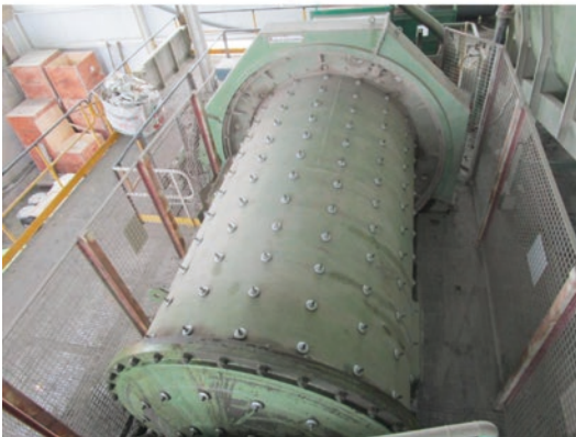
■ Fig. 6.24 Balls and a ball mill (Image courtesy of Daytal Resources Spain S.L.)
