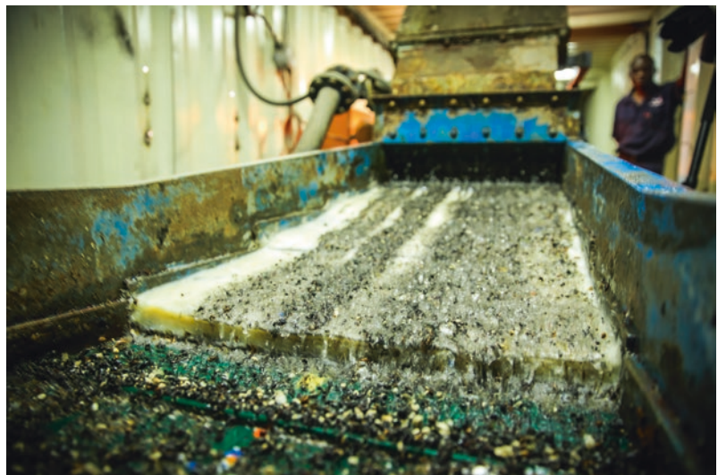
■ Fig. 6.43 Grease table used for secondary recovery (Image courtesy of Petra Diamonds)
