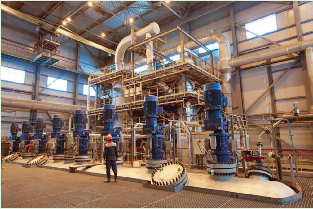
■ Fig. 6.78 Autoclave in Amursk processing plant (Image courtesy of Polymetal International plc.)
