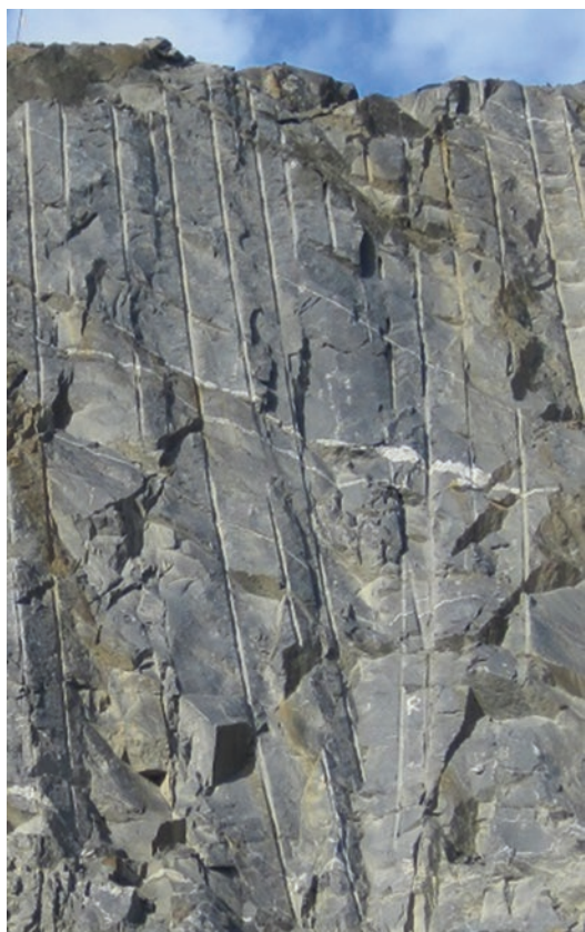
■ Fig. 3.64 Borehole deviation
