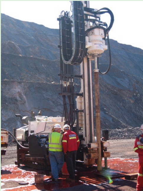
▣ Fig. 3.62 Sonic drilling in iron ore mining (Image courtesy of Sonic Drilling Ltd.)
