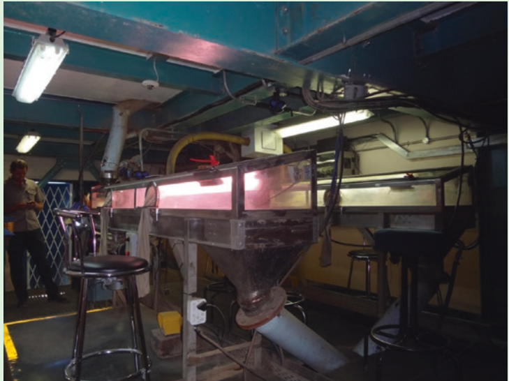
■ Fig. 6.45 Secure hand sort (glove box and drop box) facility at the final recovery plant (Image courtesy of Rockwell Diamonds)
