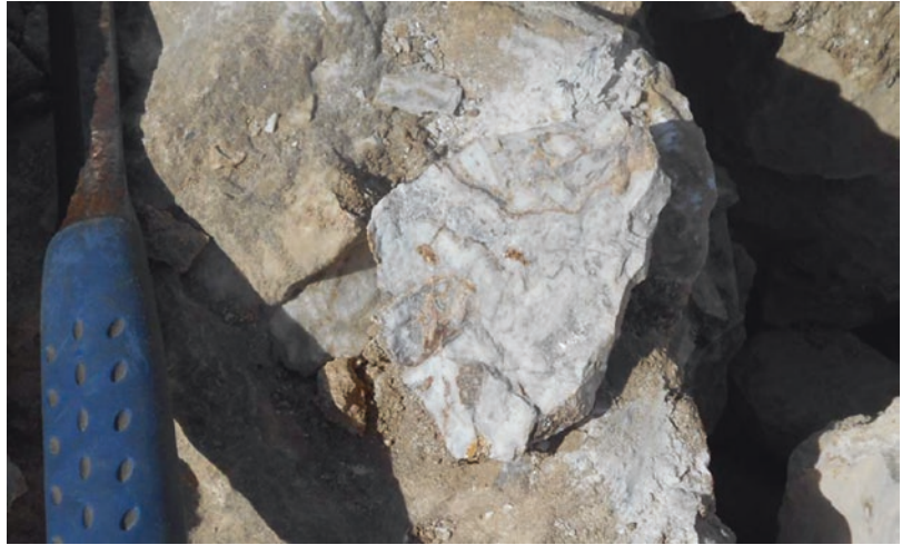
■ Fig. 3.77 Crustiform quartz from Paciencia prospect (Image courtesy of Arena Minerals Inc.)
