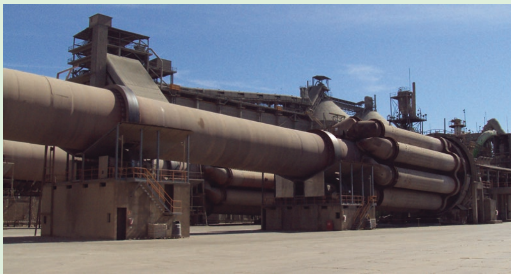
Fig. 2.31 Rotating kiln to manufacture cement (Image courtesy of Grupo Cementos Portland Valderrivas)
