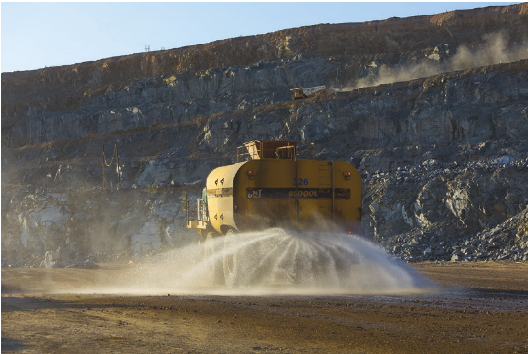
■ Fig. 5.24 Control of dust generation (Image courtesy of Anglo American plc)
