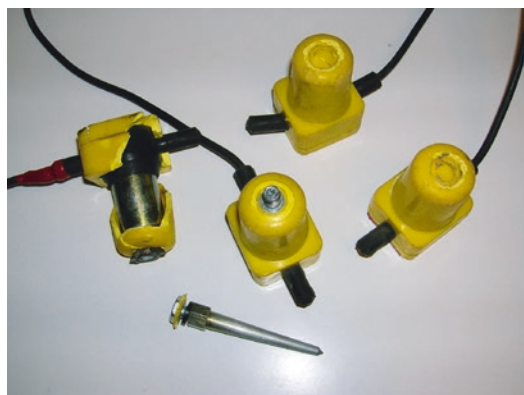
■ Fig. 3.16 Geophones for receiving seismic signal (Image courtesy of International Geophysical Technology)
