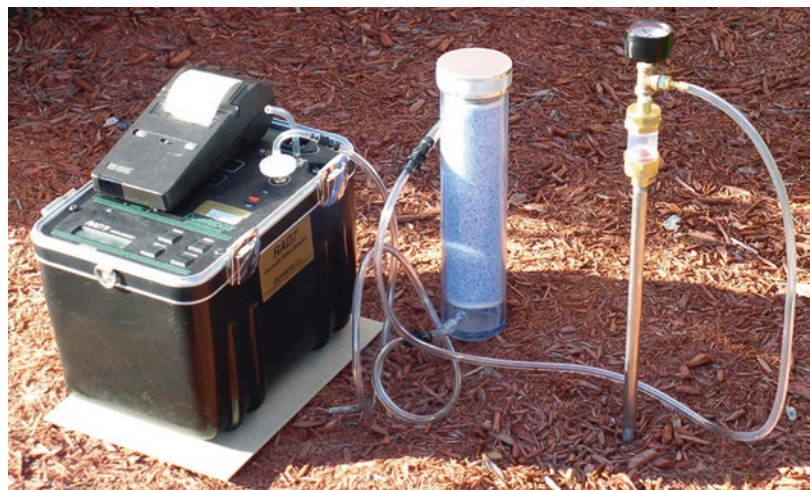
■ Fig. 3.36 Measurement of soil radon using a soil gas probe (Image courtesy of DURRIDGE Company Inc.)
