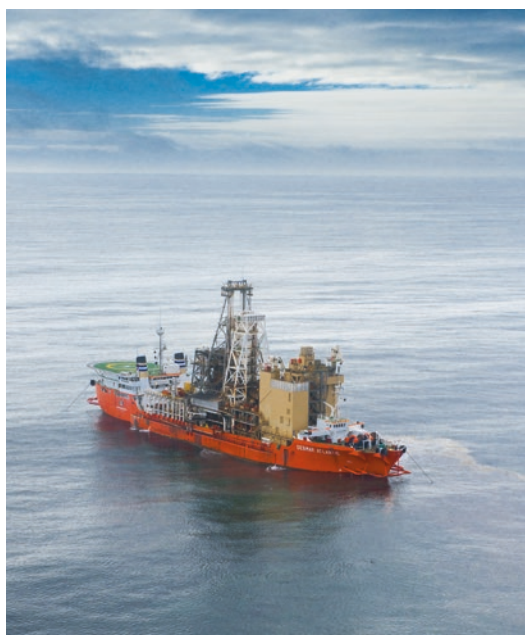
■ Fig. 2.47 The Debmar Atlantic is one of five deep-water mining vessels operating off the Namibian coast to extract diamonds (Image courtesy of De Beers)
