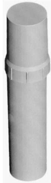
The activity of a dosage contained in a syringe is measured by placing the syringe in a plastic insert which is placed inside the dose calibrator. The activity is displayed in Ci, mCi, or  $\mu\text{Ci}$  units or GBq, MBq, or kBq units. Unit dosages (e.g.,  $^{18}\text{F}$ -FDG) supplied by the manufacturers are not required to be assayed again at the receiving facility. However, it is a good practice to assay it anyway.
