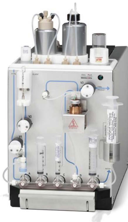
FIGURE 8.4. An automated F-18-Plus nucleophilic fluorination system. (Courtesy of Bioscan, Inc., Washington, DC)
