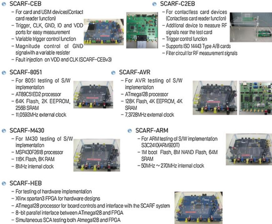
**Fig. 5** Main features of SCARF evaluation boards
