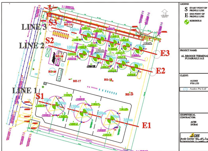
Fig. 23. Layout of 3 MASW lines covering all tanks locations
