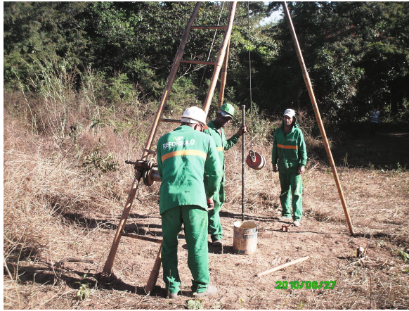
Fig. 11. Implementation of the SPT survey on the river Itacarambi possible to bridge the implementation outline of São Joao Mission.
