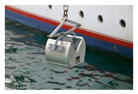
Fig. 2 Grab sampler being deployed from RV Urania
