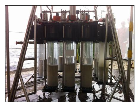
Fig. 7 Megacorer set up with nine sampling tubes has just been retrieved on RRS James Cook
