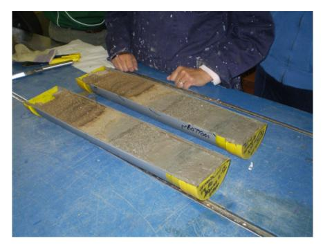
Fig. 11 Split piston core, way up towards the *top left corner*. One half will be archived and the other half will be used for logging and sampling
