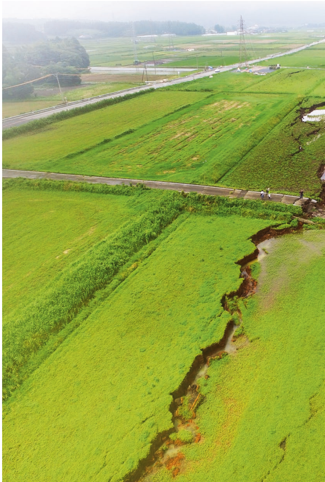
Fig. 36 Drone image showing a coseismic graben structure developed inside Aso caldera
