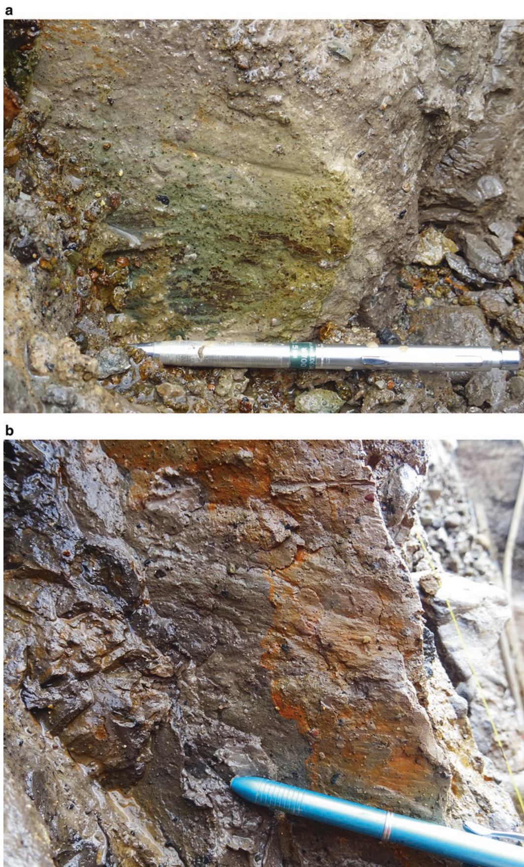
Fig. 16 Slickensides upon coseismic fault planes. (a, b) Coseismic fault plane developed within basement rocks ( sandstone ) and (c, d) unconsolidated surface soil layer. Striations developed on main fault planes indicate a strike-slip-dominated movement sense
