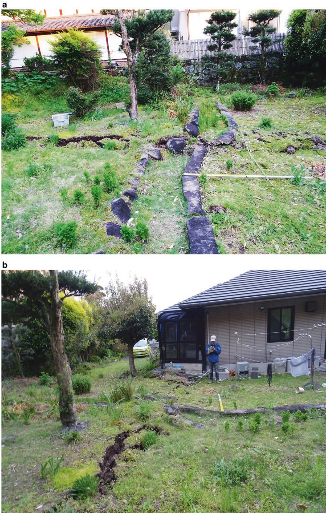
Fig. 9 Right-lateral offset of ditch slope and damaged parking area in a house garden. (a, b) Dextral offset \sim 1.3 m with a vertical component of \sim 0.30 m. (c) Right-lateral offset of ditch slope (offset \sim 0.9 m). (d) Right-lateral offset of parking area (offset \sim 1.1 m)
