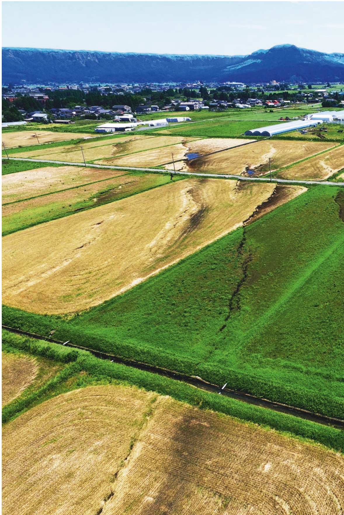
Fig. 38 Coseismic flexure structures formed in rice fields. Drone image showing a flexure feature of coseismic surface ruptures occurred in rice fields that are folded as waveform
