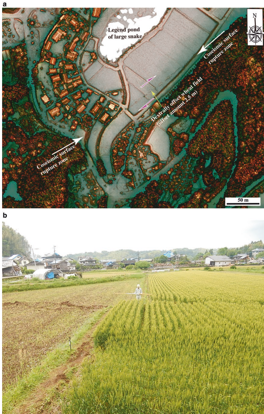
Fig. 12 Red relief image and photographs showing the right-lateral offset of fields. (a) Red relief image (image courtesy T. Chiba). (b, c) Right-lateral offset of wheat field. Photograph taken on 1 May 2016 (d) Photograph taken on 20 June 2016 after the wheat crops
