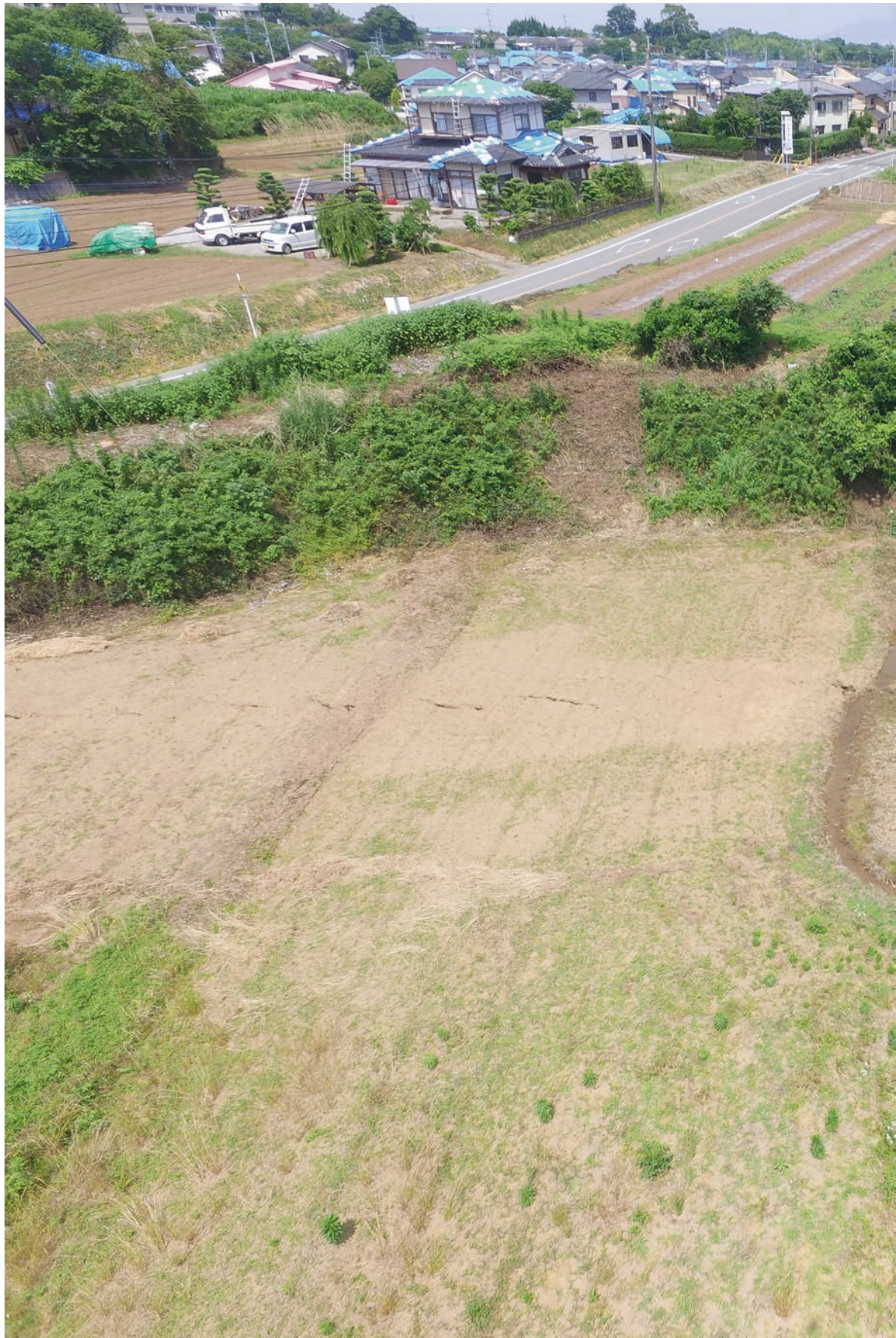
Fig. 53 Drone image showing an overview of the Takagi trench site. A coseismic surface rupture zone occurred along the preexisting fault scarp of the Hinagu fault, where field paths were dextrally offset by
