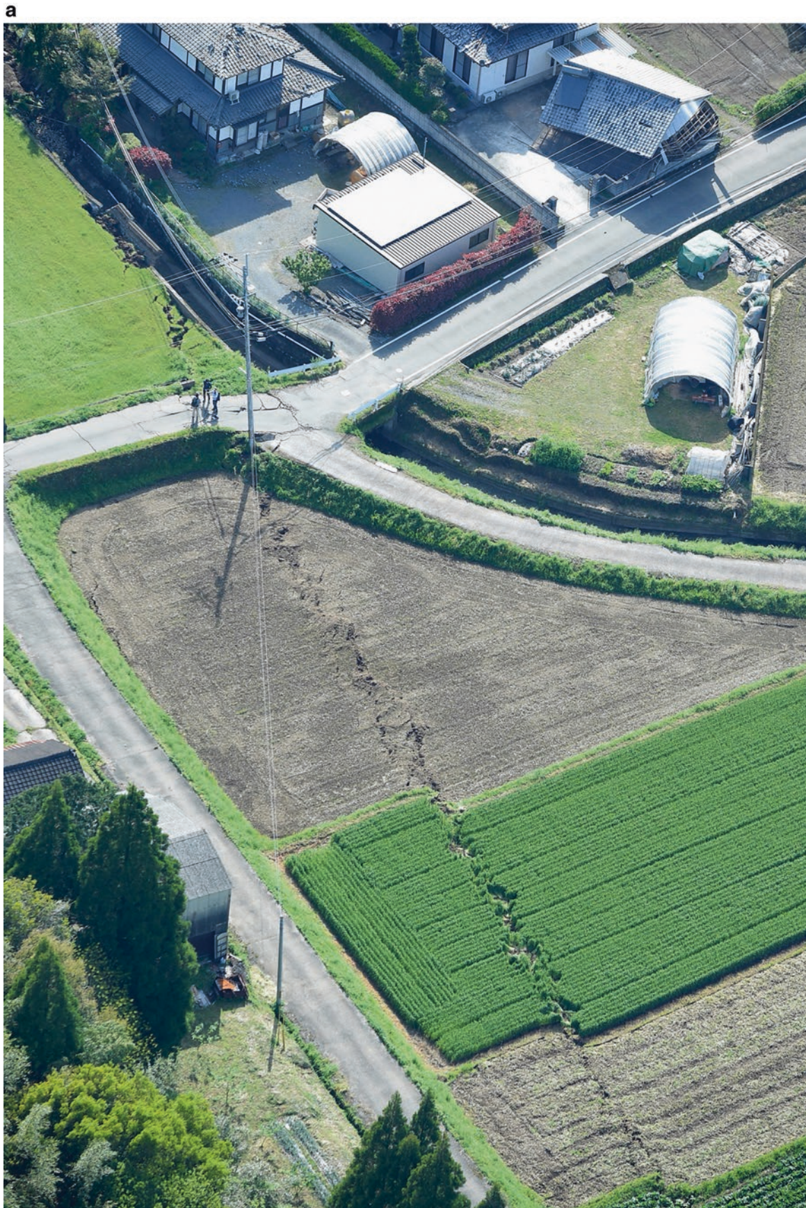
Figure Plate 3 Right-lateral strike-slip offset of wheat fields in the coseismic surface rupture zone. (a) Aerial photograph (with permission from The Mainichi Newspapers). (b, c) Strike-slip offset of field paths,
