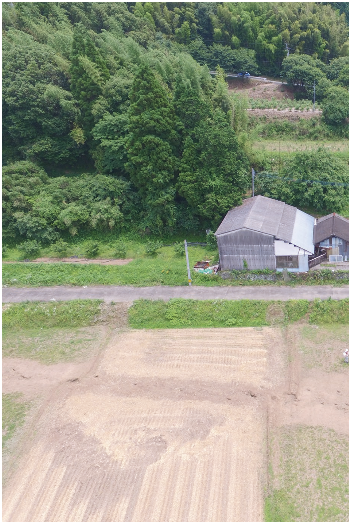
Fig. 60 Drone image showing an overview of the Kamijin trench site. Field paths were dextrally offset by ~2.5 m
