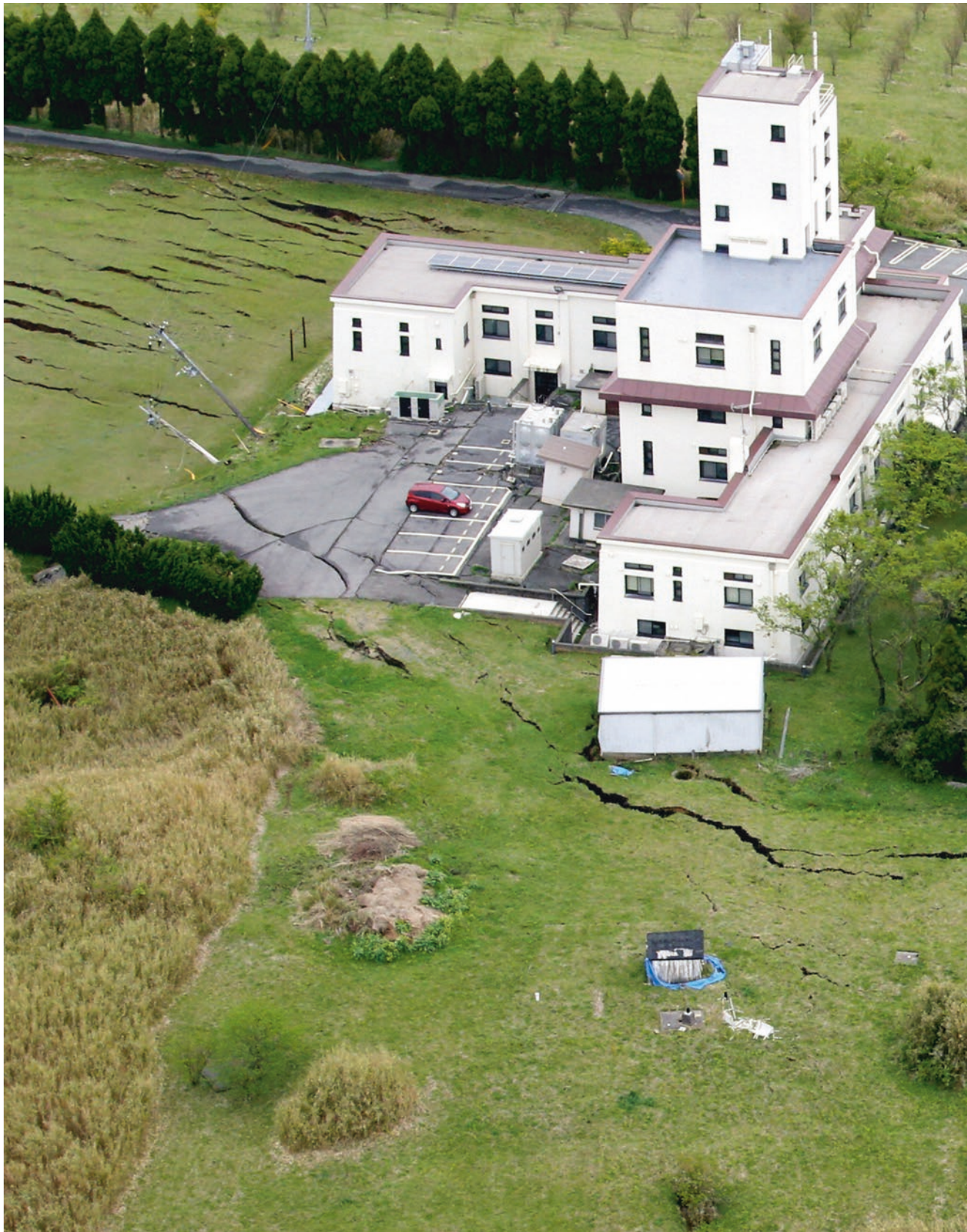
Fig. 67 Aerial photograph showing a close-up view of coseismic tension cracks shown in Fig. 66. Parallel-subparallel coseismic tension cracks developed in the house yard of the Volcanological Laboratory,
