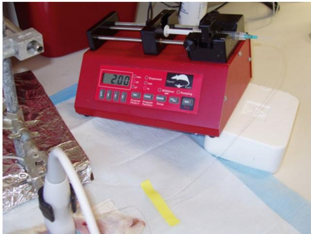
**Fig. 13** Infusion pump connected with the catheter
