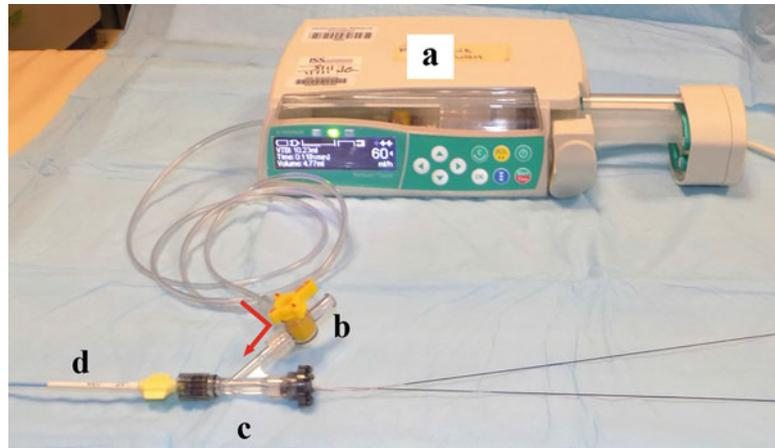
**Fig. 2** Slow intracoronary perfusion system. During the infusion, the Y-connector valve should be tightly locked to prevent the vector solution from loss. Pressure monitor line can be connected to femoral arterial sheath during injection. (a) Infusion pump. (b) Three-way stopcock for exchanging the infusion line and pressure monitor line (also to the manifold for angiography). (c) Y-connector with hemostatic valve and coronary wires. (d) Guiding catheter
