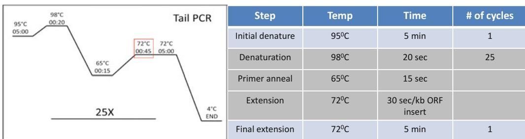
**Fig. 2** PCR setting for synthesizing DNA tailed template. Highlighted in red is the elongation step that must be set based on the size of the sequence insert. Elongation step requires 30 s per KB of ORF insert. PCR setting is based of manufacturer instructions from 2× KAPA HiFi HotStart ReadyMix kit
